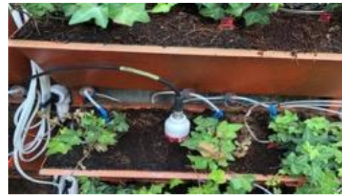
Figure 2.19 The location of the SM150T SMS in the LWS at left section view (left image) and perspective view (right photo)
