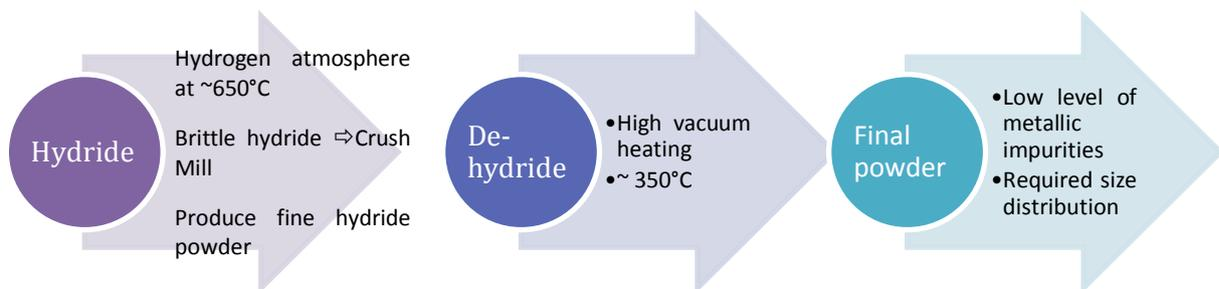
Figure 2. 8 Schematic diagram of HDH process (41)
