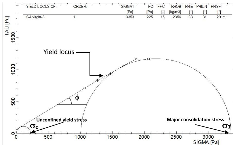
Figure 4. 7 Illustration of the Mohr's circle, major consolidation stress ( $\sigma_1$ ) and unconfined yield stress ( $\sigma_c$ ), internal angle of friction and yield locus for GA powder
