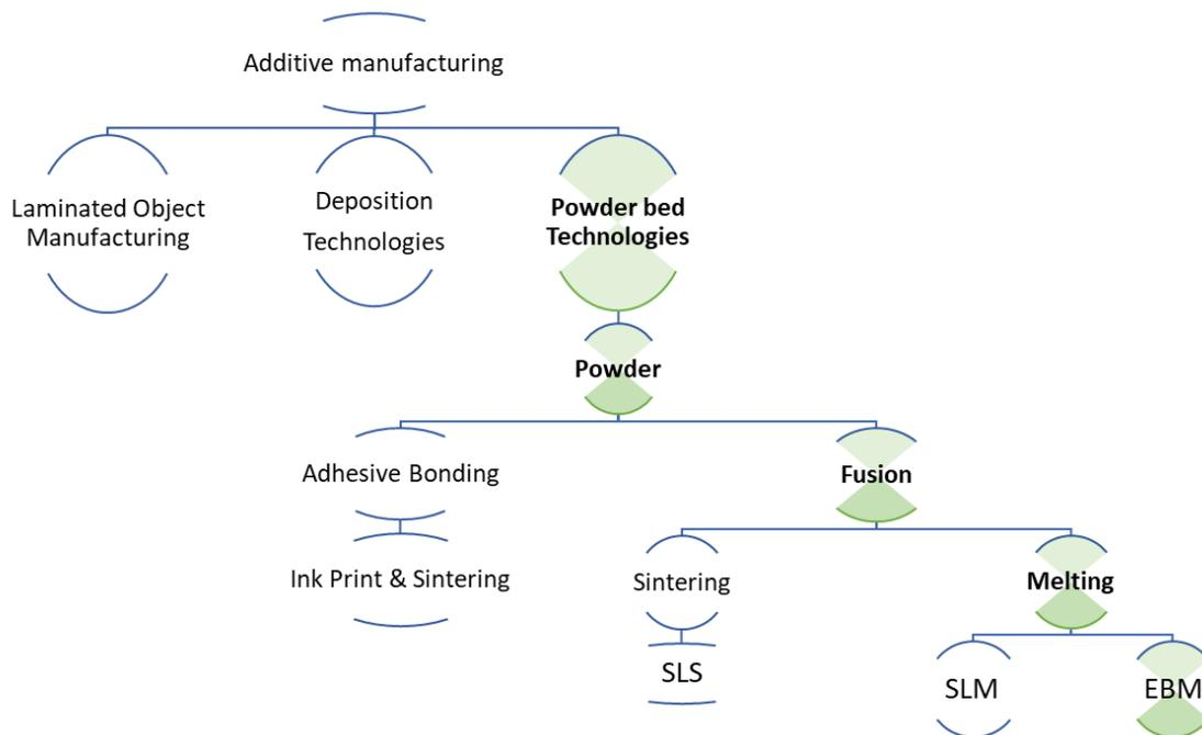
Figure 2. 1 Categorization of additive manufacturing technique
