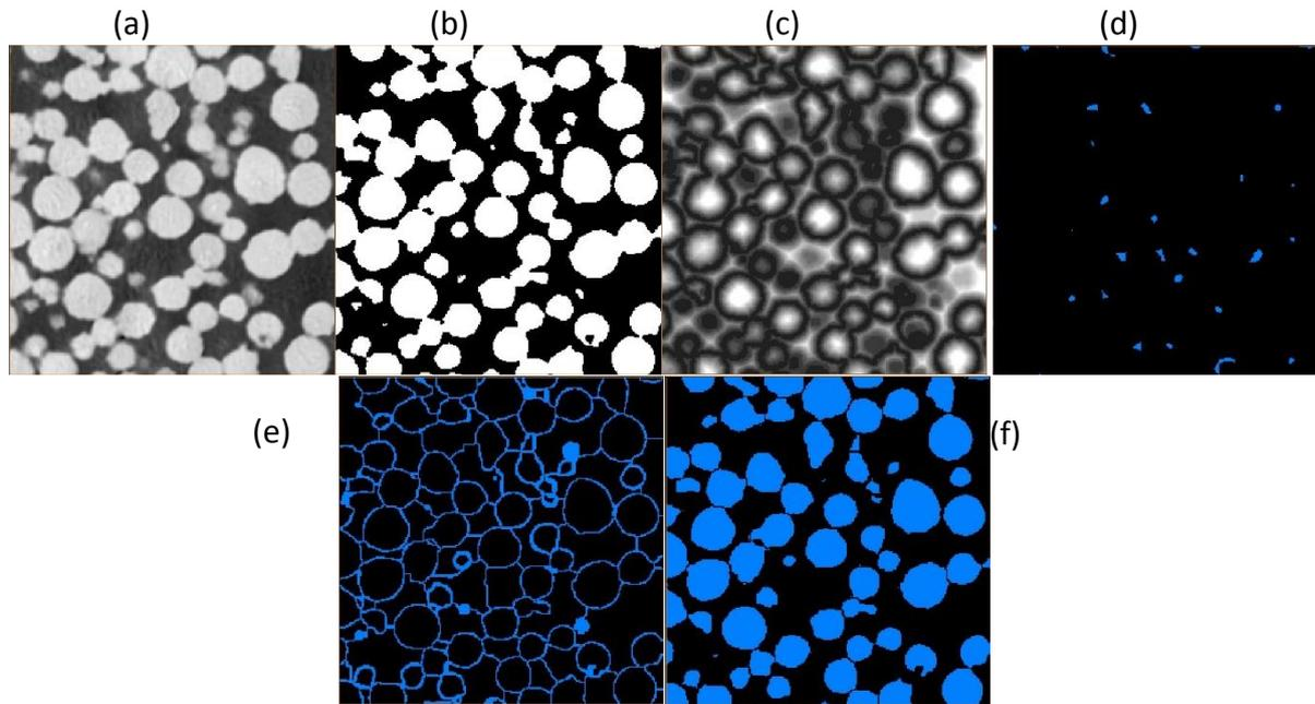
**Figure 3. 7 Steps of digital separation of particles. (a) Original greyscale image of powder GA, (b) initial binary images of attached particles, (c) distance transformation, (d) H-maxima transformation, (e) image after watershed segmentation line, (f) separated particles**
