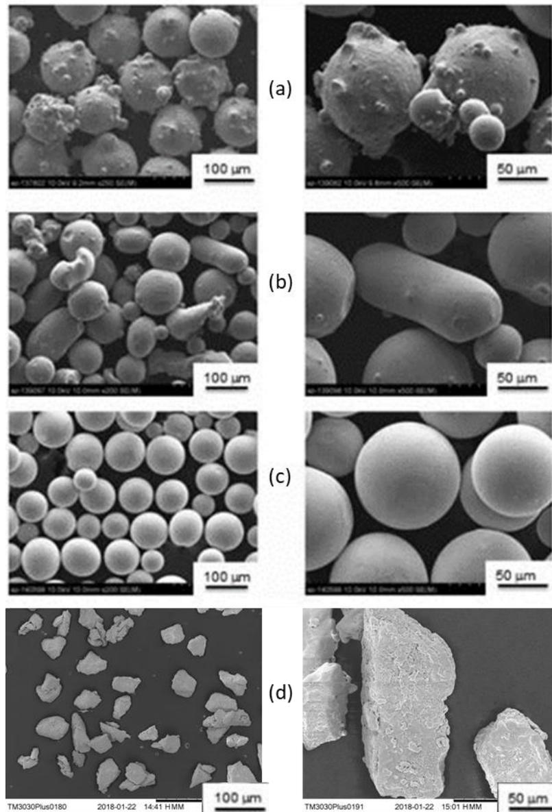
**Figure 2. 10 Spherical Ti6Al4V particles produced by (a) GA process, (b) PA process (c) PREP process (40) and (d) HDH process**
