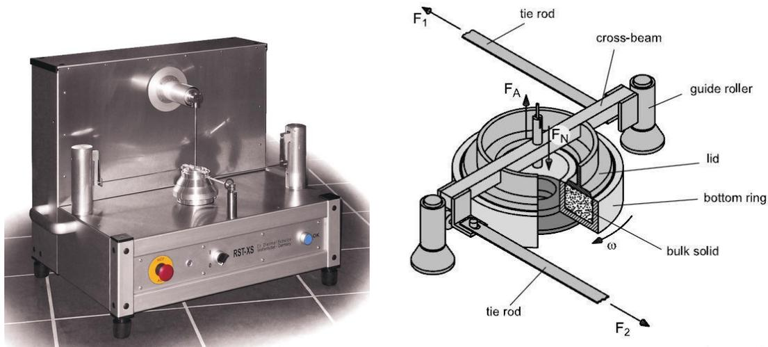
Figure 3. 24 Ring shear cell RST-XS (58)
