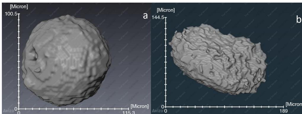
**Figure 3. 9 Close up images of reconstructed particles (a) GA and (b) HDH**
