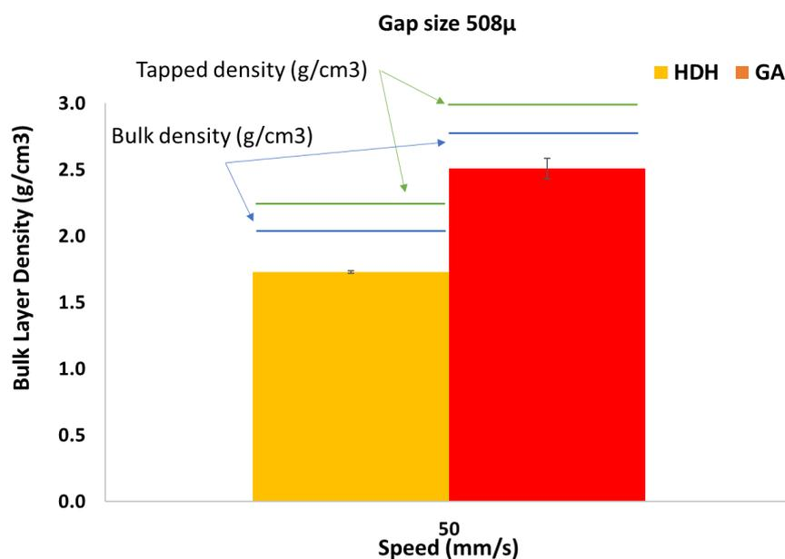
Figure 4. 20 Comparison of powder bed density with apparent and tapped density for (a) GA and (b) HDH
