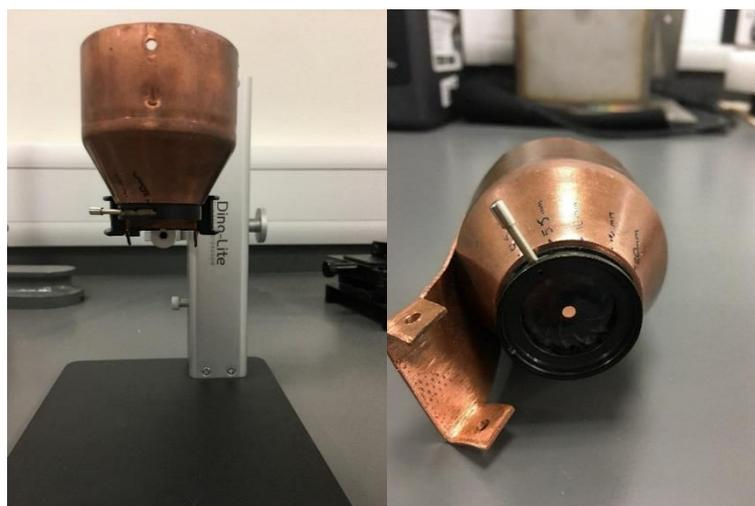
Figure 3. 22 In-house flowmeter (a) whole set-up (b) close-up look at orifice adjustment
