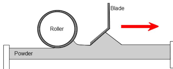
Figure 2. 6 Using the blade and rotating and vibrating roller (29)
