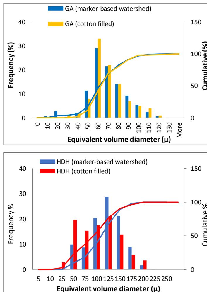
Figure 3. 8 Comparison of the cotton filled and marker-based watershed segmentation methods to characterise of particle size distribution
