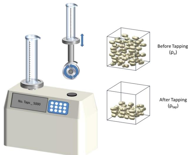
Figure 2. 12 Illustration of tapped density measurement (image credit: Freeman technology)
