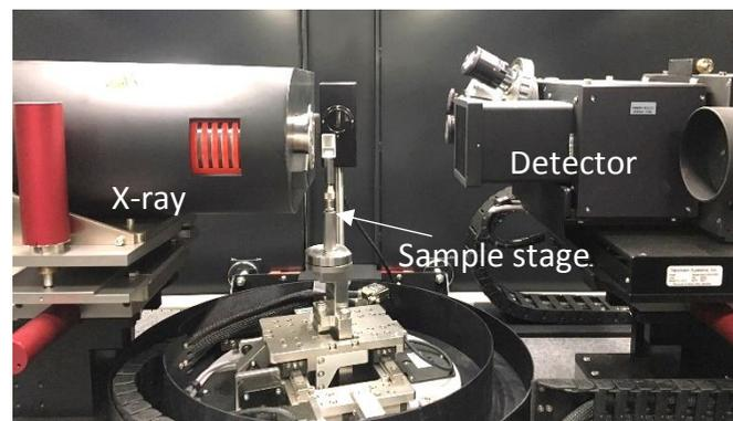
Figure 3. 5 Inside the Micro XCT, Xradia Versa 410
