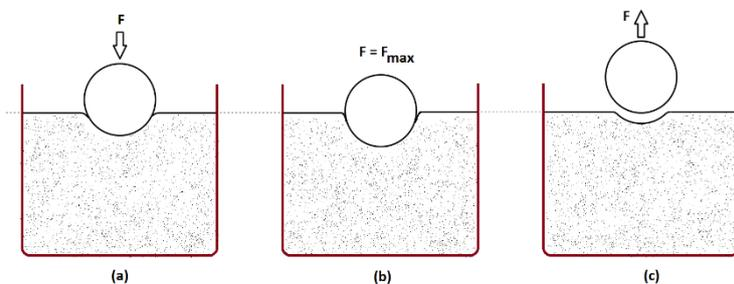
Figure 2. 19 Schematic of ball indentation (a) loading, (b) maximum loading and (c) unloading (76)
