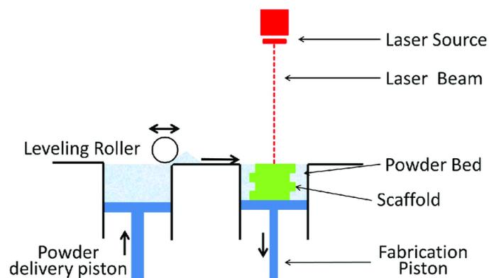
Figure 2. 3 Schematic diagram of SLS process (23)
