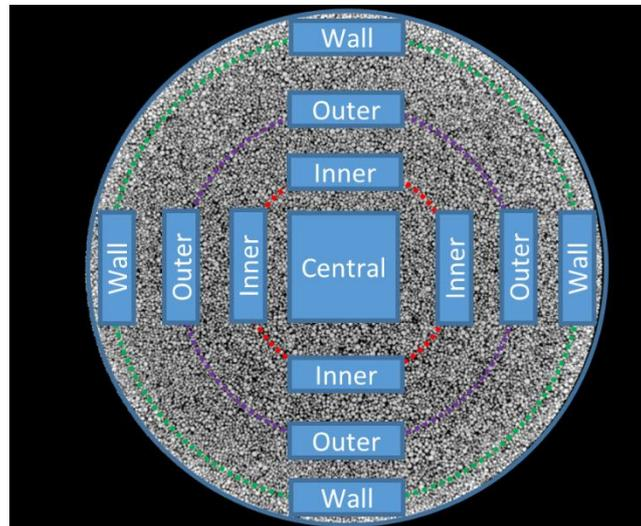
Figure 5. 5 2D Cross section slide of HDH powder with region of interest
