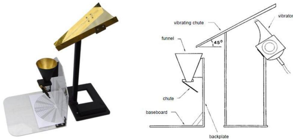
Figure 3. 18 Mark 4 Powder research Ltd. AOR tester
