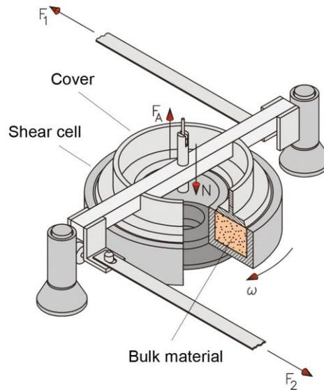
Figure 2. 17 Illustration of Schulze ring shear cell test (58)
