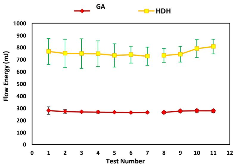
Figure 4. 6 Flow energy measurement at fixed and variable blade tip speed
