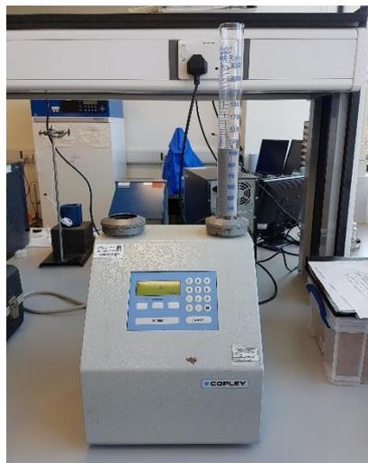
Figure 3. 17 The apparatus of Tapped density equipment
