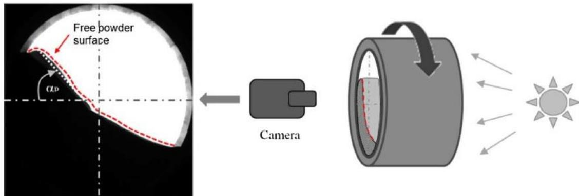
Figure 3. 20 Schematic of avalanche angle measurement
