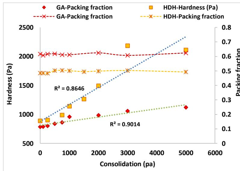
Figure 4. 11 Hardness and packing measurement of GA and HDH samples by using ball indentation
