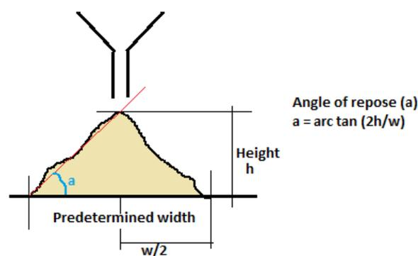
Figure 2. 13 Illustration of angle of repose technique (image credit: Wikipedia)
