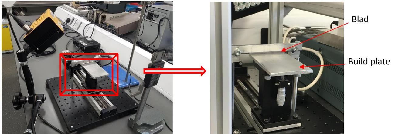
Figure 4. 19 Rig set up of spreading process
