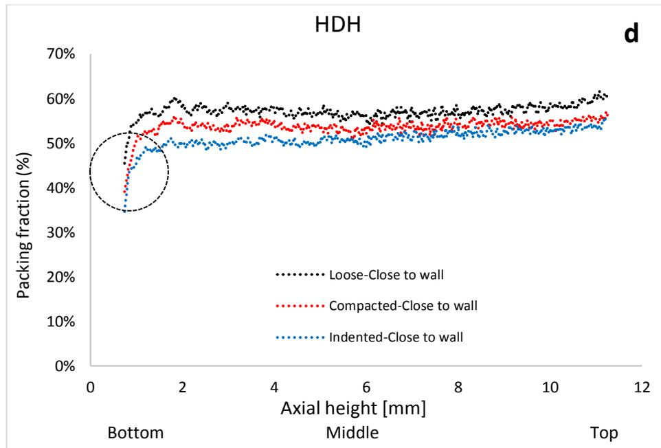
Figure 5. 9 Axial packing fraction for GA powder in (a) central zone, (b) wall section and for HDH powder in (c) central, (d) wall zone at “loose-compacted- indented” stages
