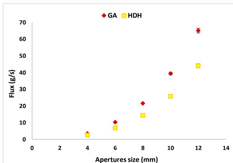
Figure 4. 4 Mass flow rate profile for GA and HDH powders
