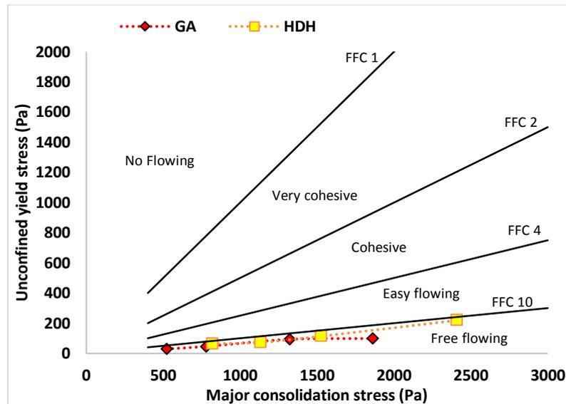
Figure 4. 9 Ring shear RST-XS.s test results for both samples GA and HDH (Ti6Al4V)
