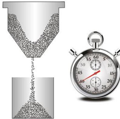
Figure 2. 14 Illustration of powder flowrate measurement (image credit: [bettersizeinstruments.com](http://bettersizeinstruments.com))
