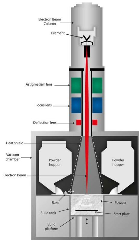
**Figure 2. 4 Electron Beam Melting (EBM) mechanism (image credit: arcam.com)**
