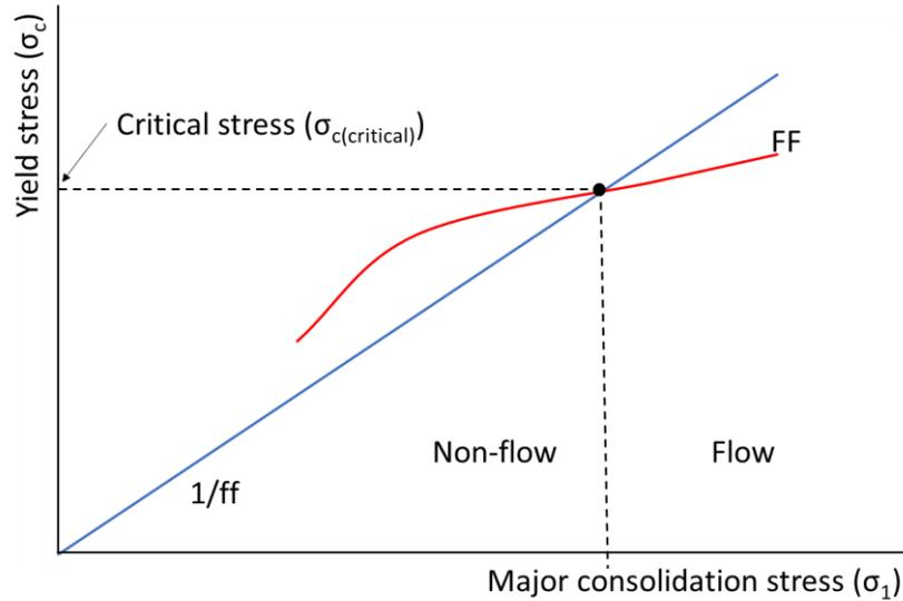
Figure 4.17 Criterion of flow and non-flow regarding to critical applied stress
