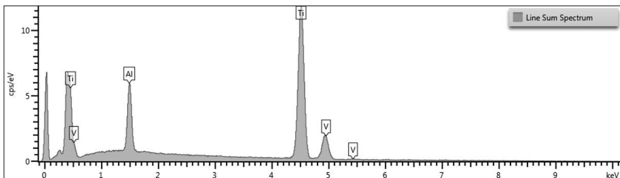
Figure 3. 3 The elemental composition of the Sample 1 according to the X-ray intensity and specific wavelengths
