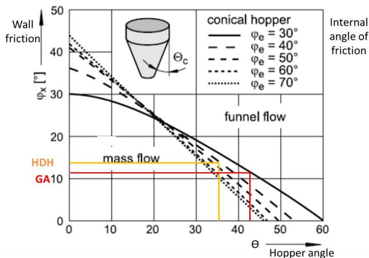
Figure 4. 15 Mass flow diagram for conical hopper (17)
