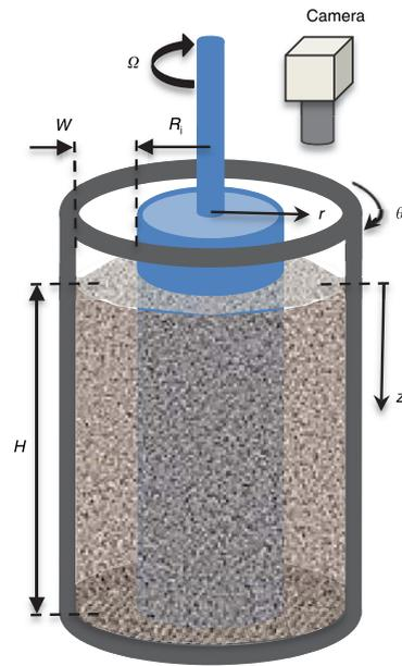
Figure 2. 21 Illustration of Couette device (87)
