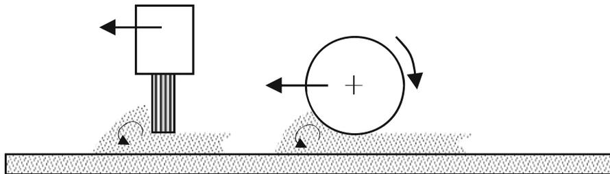
Figure 2. 5 Spreading systems; Roller and Blade (3)
