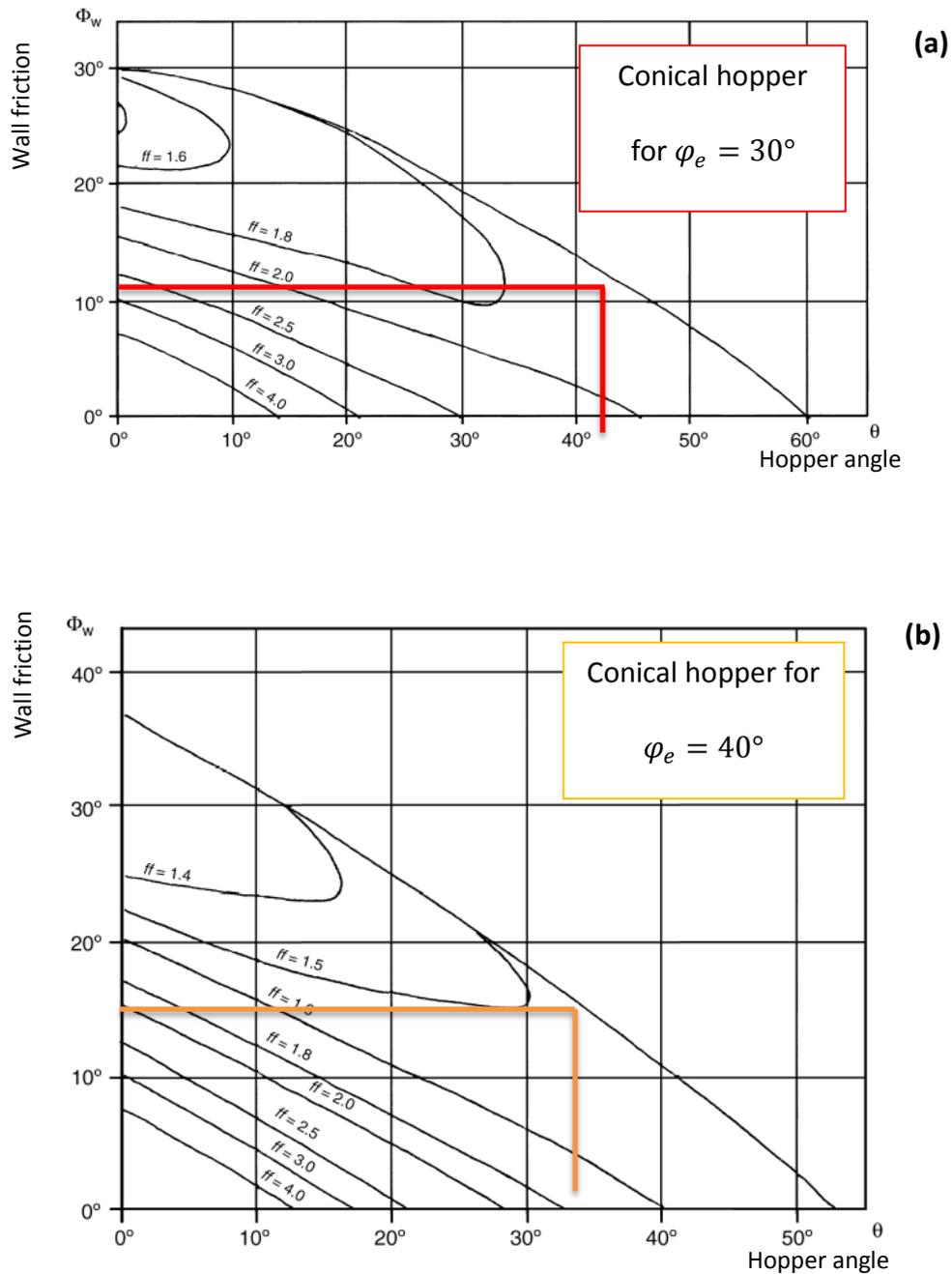
Figure 4. 16 Hopper flow factor values for conical channels, (a) for internal angle of friction of 30 (GA). (b) for internal angle of friction of 40 (HDH) (17)
