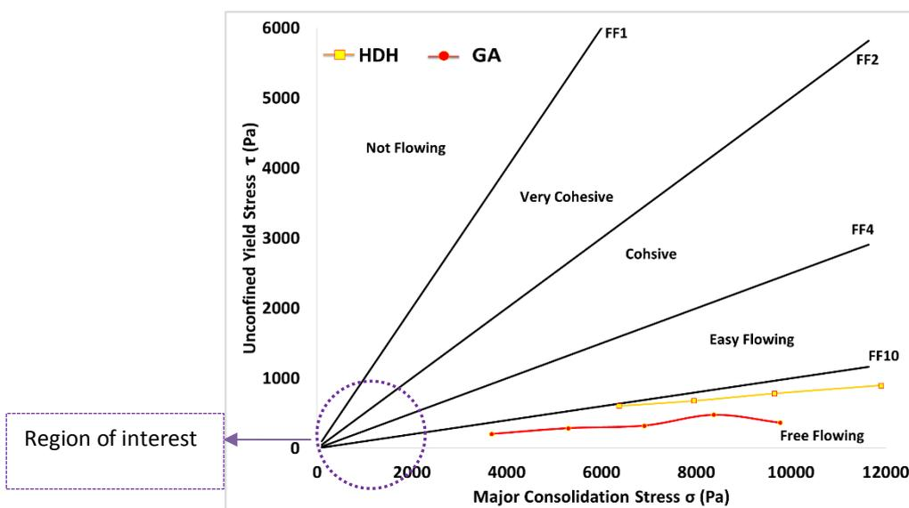
Figure 4. 8 Ring shear test results for both samples GA and HDH (Ti6Al4V)
