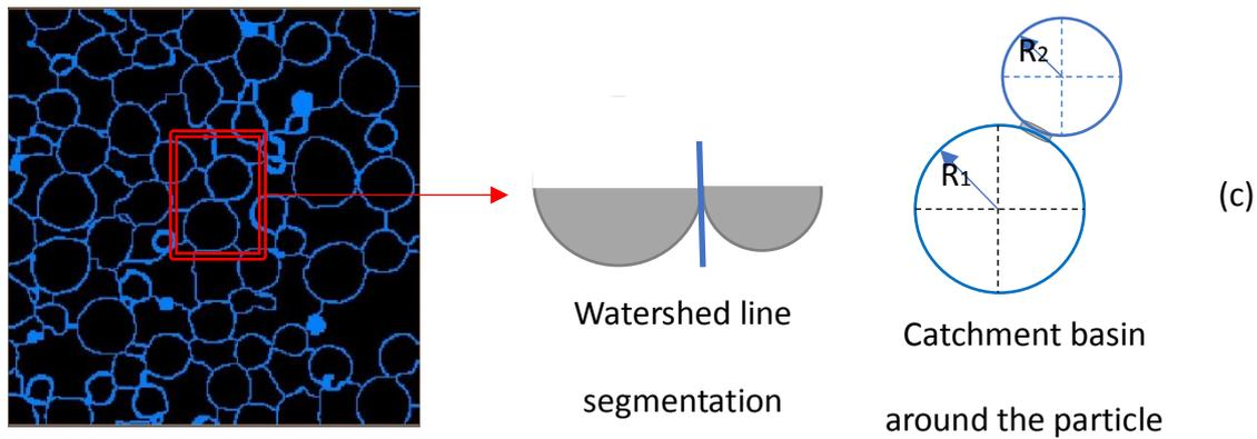
Figure 3. 6 Illustration of watershed segmentation
