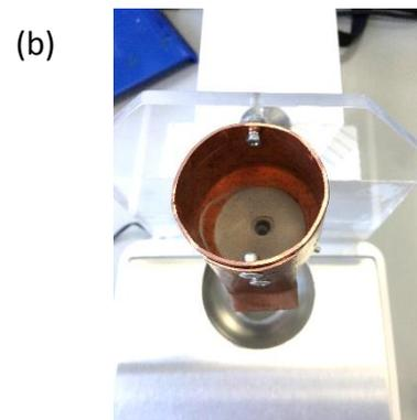
The flowmeter technique for HDH powder demonstrating powder creating rat hole at the 1 mm orifice size.
