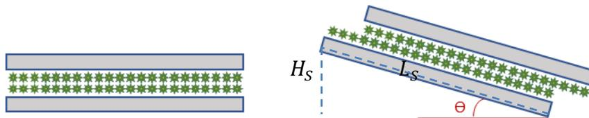
Figure 5. 8 Schematic diagram for measuring CoF between particle-particle
