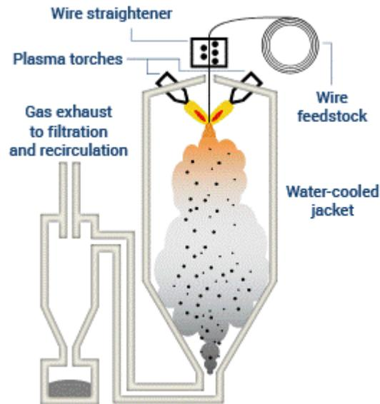
Figure 2. 9 Schematic diagram of Plasma Atomization (PA) (image credit: advancedpowders.com)
