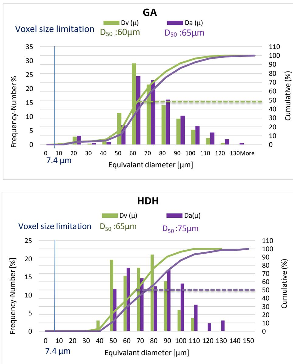
Figure 3. 10 Comparison of equivalent diameter extracted from Volume and surface area of 20,000 individual particles
