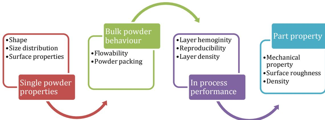
Figure 2. 22 Influencing parameters and their analysing method on metal powder for AM process (97)
