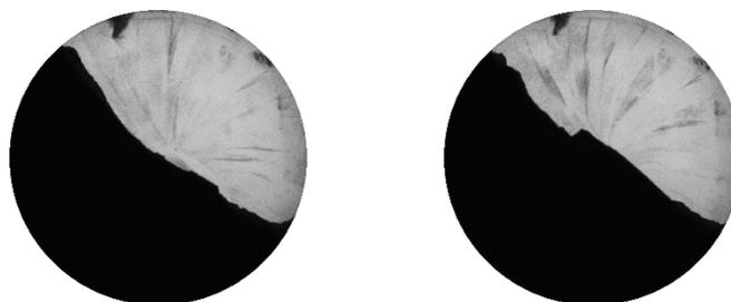
**Figure 4. 3 Illustration of surface fractal and avalanche angle for top (GA) and bottom (HDH) powders just before and after avalanche happening**
