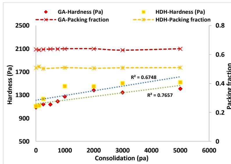
Figure 4. 13 Hardness and packing measurement of GA and HDH on 30 tapped samples
