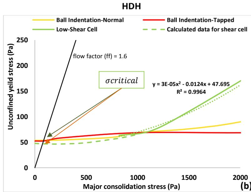
Figure 4. 18 Evaluation of Critical Applied Stress from flow function for both (a) GA and (b) HDH
