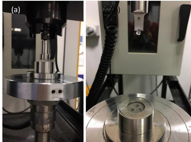
Figure 3. 25 Ball indentation process
