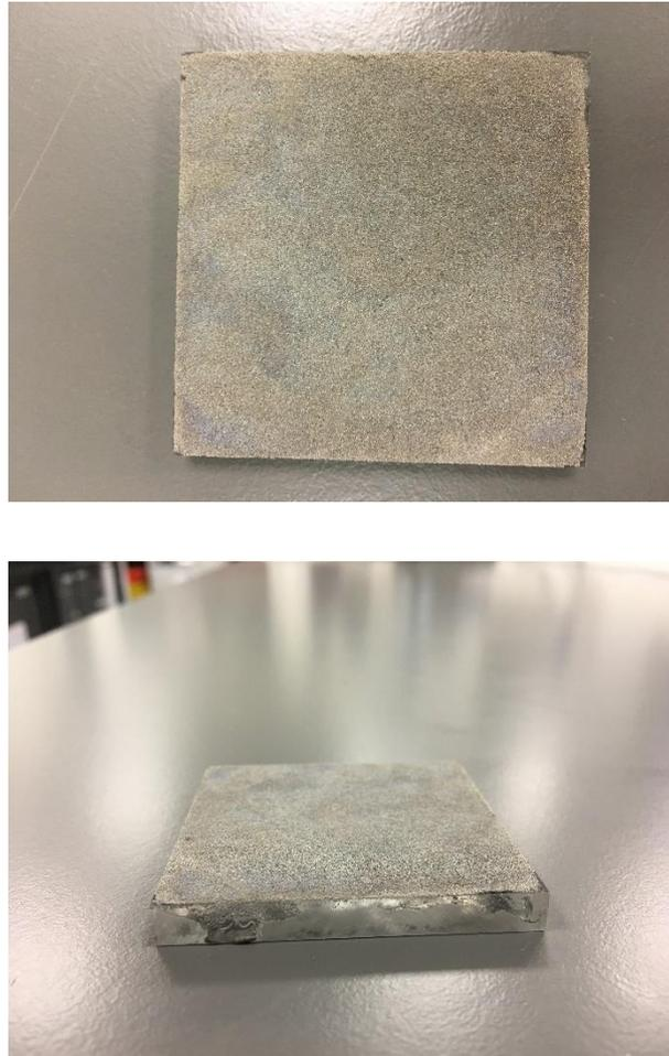
**Figure 5. 7 Image of prepared sample of GA adhered to surface for measuring CoF**
