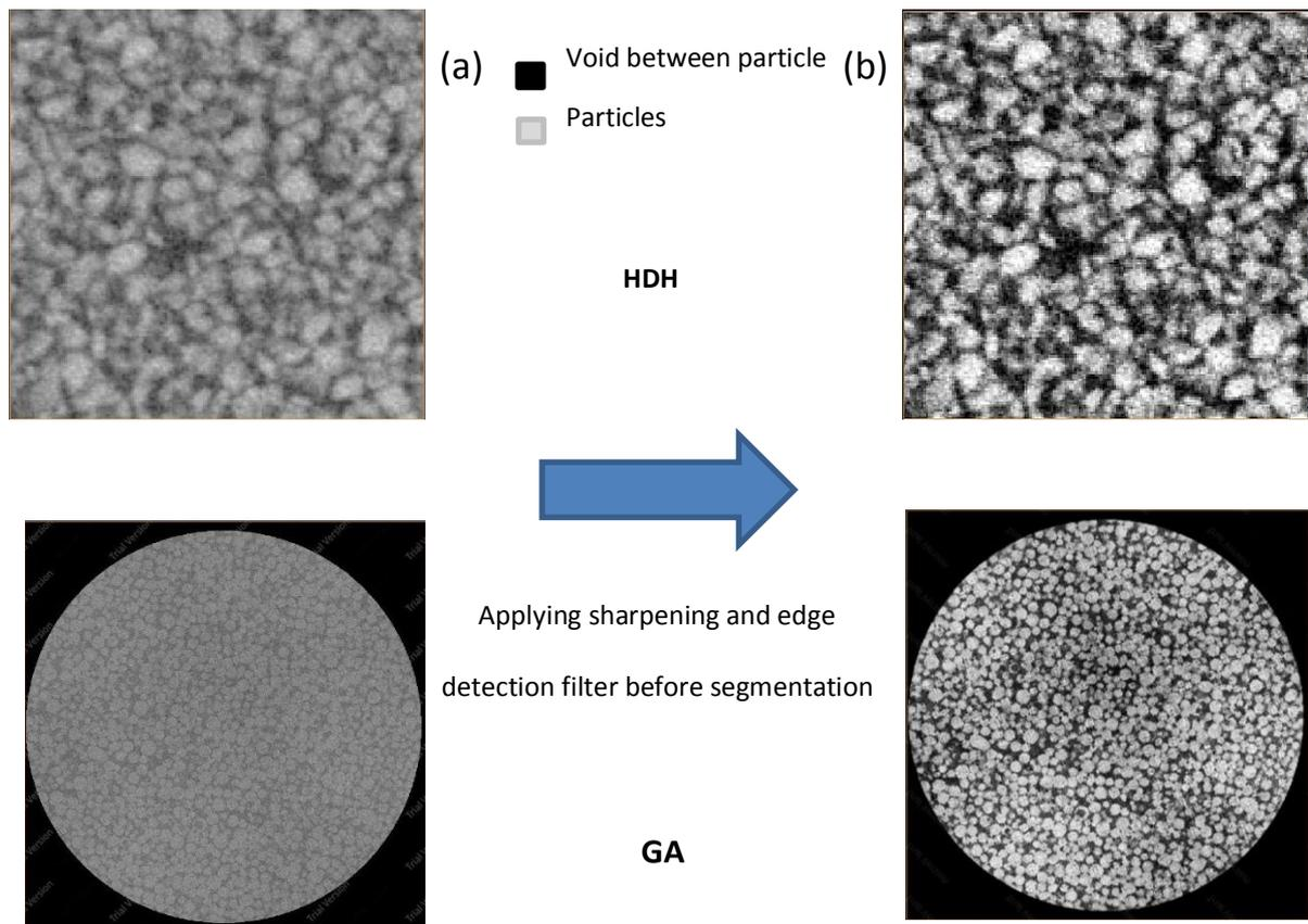
Figure 5. 3 (a) Before and (b) after sharpening filter on sample HDH and GA
