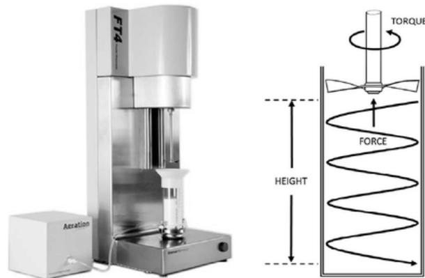
Figure 3. 23 FT4 rheometer tester (71)
