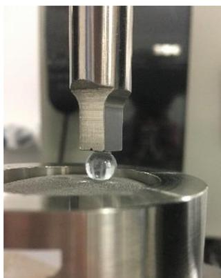
Figure 4. 10 Experimental set up of ball indentation
