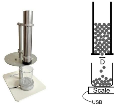
Figure 3. 21 Granuflow and the principle of measuring powder flowrate
