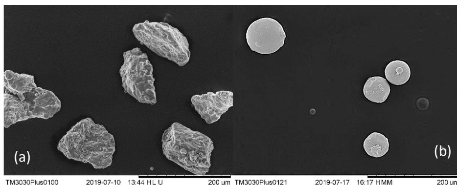
**Figure 3. 1 SEM images of (a) Hydride-dehydride (HDH) and (b) Gas atomization (GA) of Ti6Al4V samples**
