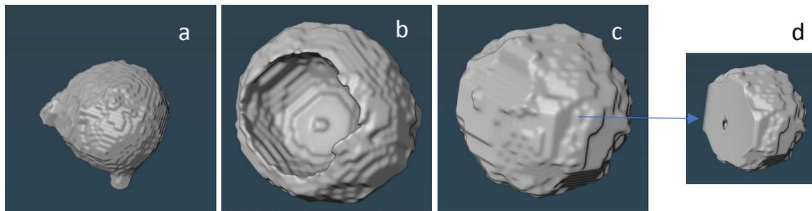
**Figure 3. 12** Different shapes of GA particles (a) particle with satellite, (b) concave particle, (c) porous particle (d) cross section of particle c
