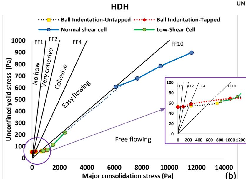
Figure 4. 14 Flow function of (a) GA and (b) HDH samples driven from shear cell and ball indentation techniques
