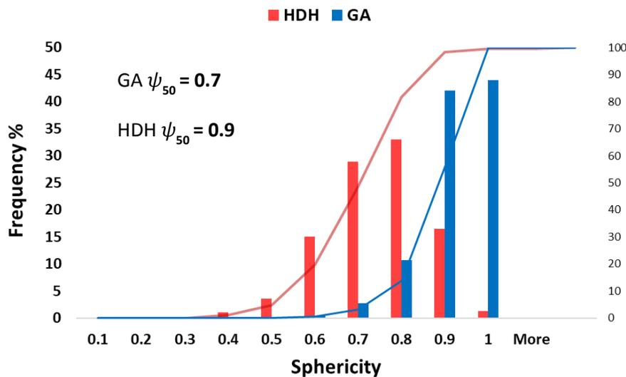
Figure 3. 11 Sphericity of GA and HDH samples
