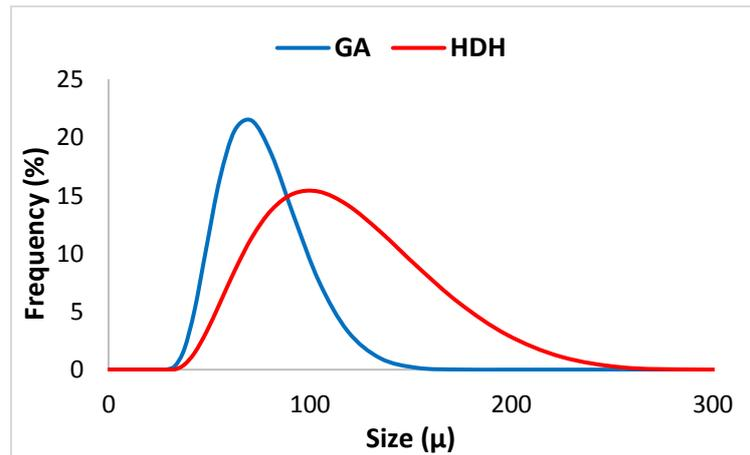
Figure 3. 2 Size distribution of GA and HDH powders measured by laser diffraction
