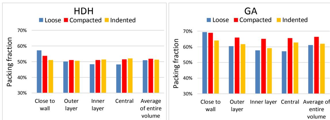
**Figure 5. 6 HDH and GA Powders packing fraction for loose, compacted and indented samples**
