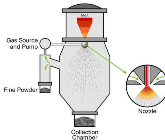
Figure 2. 7 Schematic diagram of Gas Atomisation (image credit: maschinetech.com)
