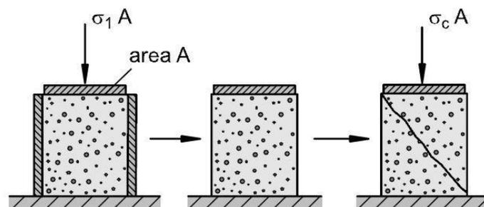
Figure 2. 16 Principal behind uniaxial compression test (69)
