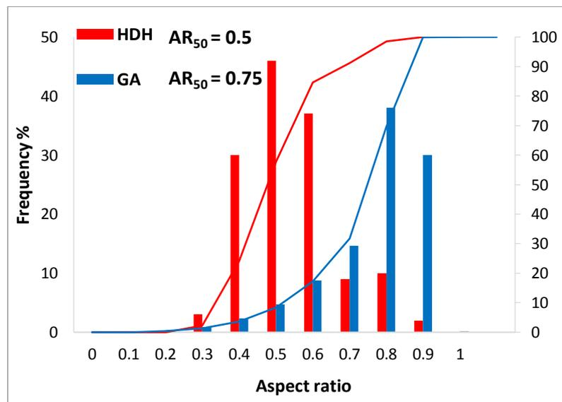
Figure 3. 14 Aspect ratio of GA and HDH samples
