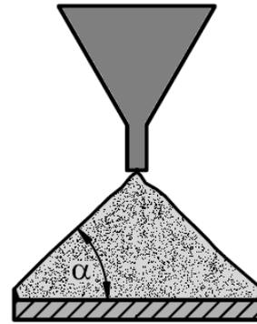
Figure 3. 19 Angle of repose
