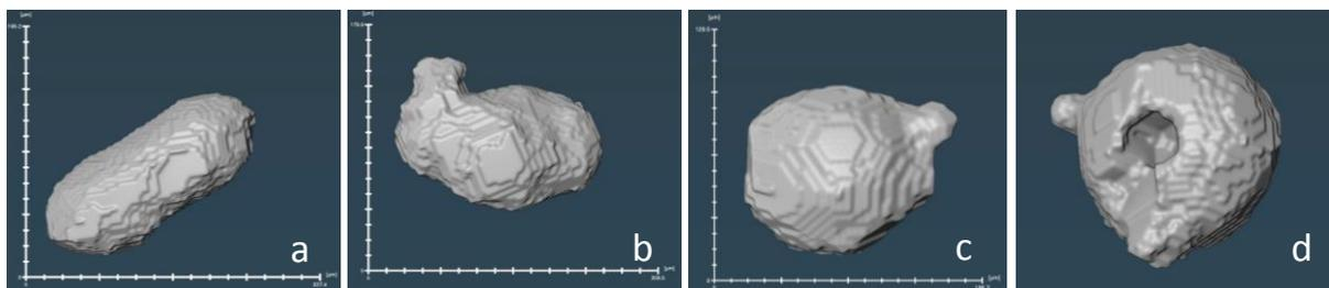
**Figure 3. 15 GA particles with 0.4 to 0.8 range of aspect ratio (AR); (a) AR= 0.43 (b) AR= 0.57 (c) AR= 0.70 (d) AR= 0.83**
