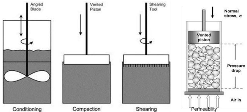
Figure 2. 18 Illustration of FT4 rheometer (image credit: Freeman technology)
