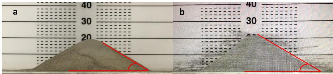
Figure 4. 2 Experimental set up of AOR on (a) GA and (b) HDH samples
