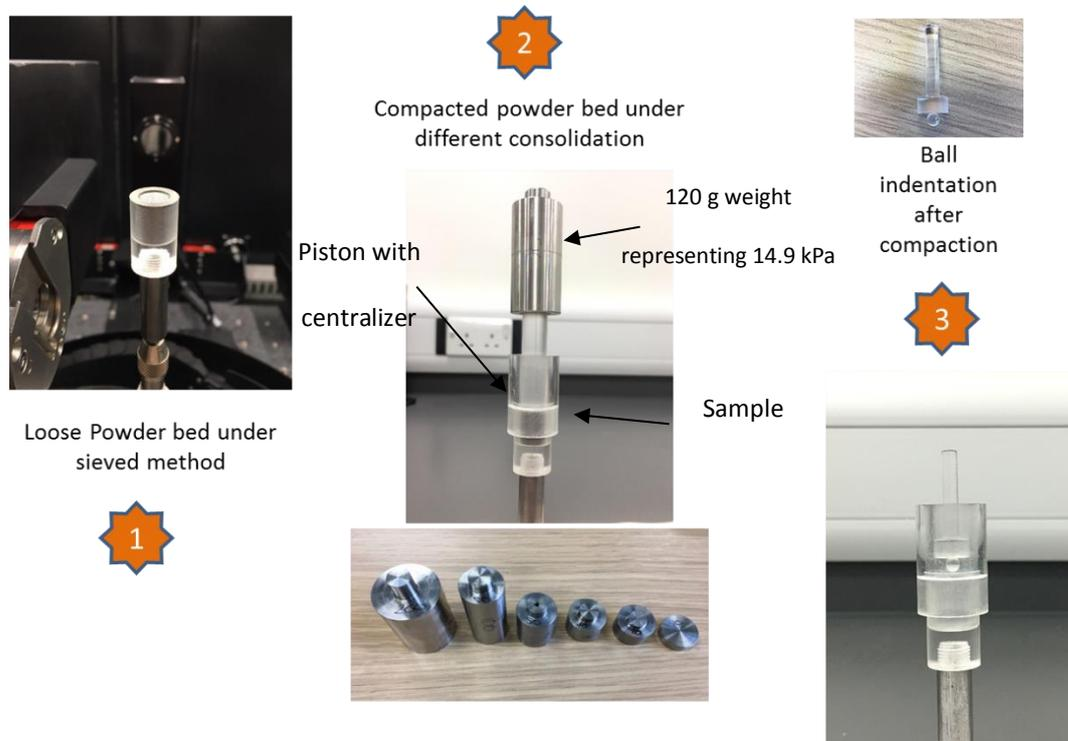
Figure 5. 1 Sample preparation for three stages of indentations during X-ray micro tomography
