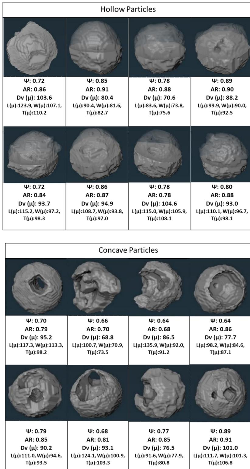
Figure 3. 16 Comparison of hollow and concave particles for their sphericity, aspect ratio, porosity and diameters
