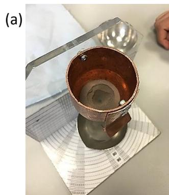
The flowmeter technique for GA powder indicating that powder discharge easily at 1 mm orifice size.
