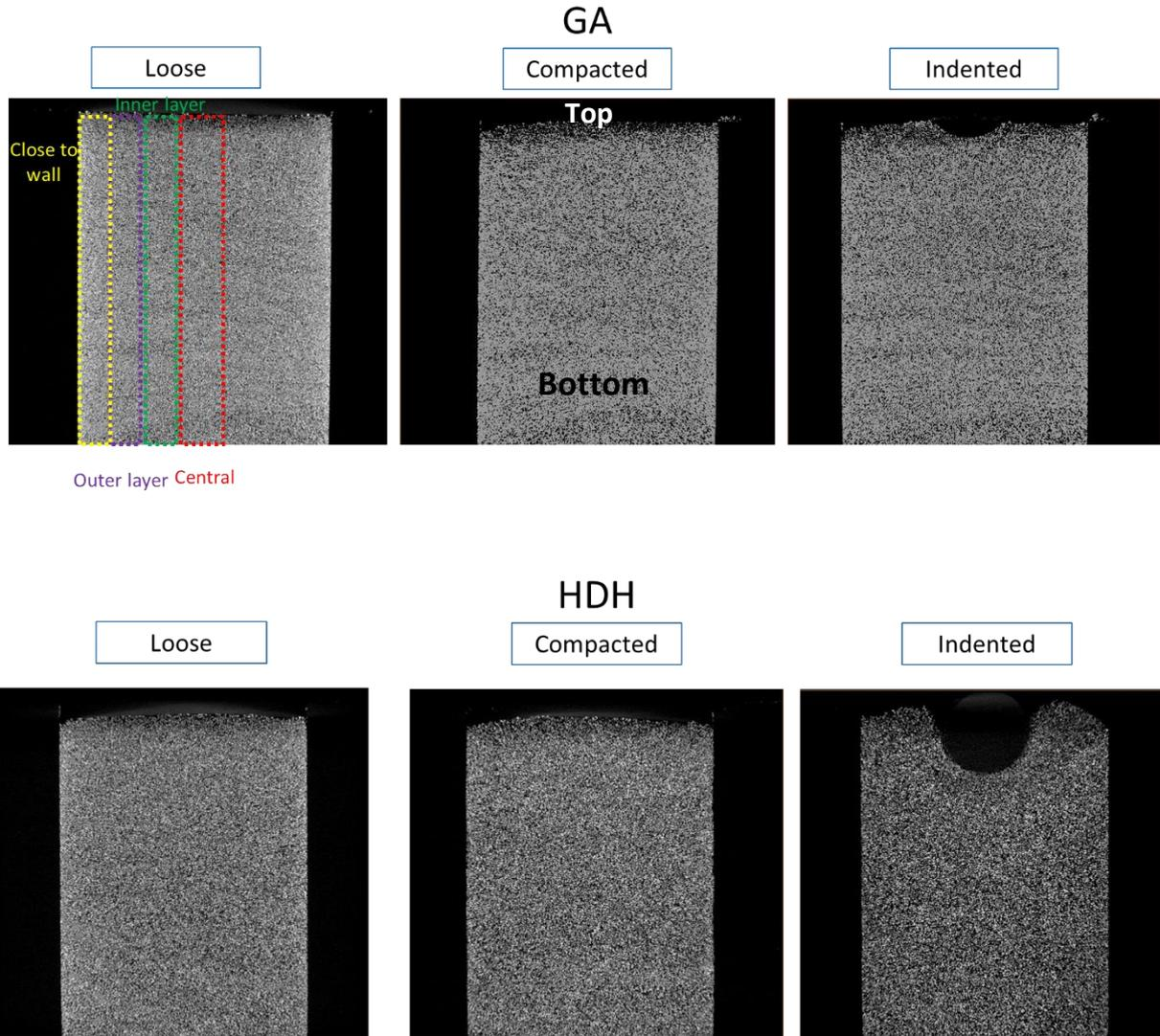
Figure 5. 4 2D Axial greyscale slide through the 3D volume for each test (Loose-Compacted-Indented) of GA and HDH powders
