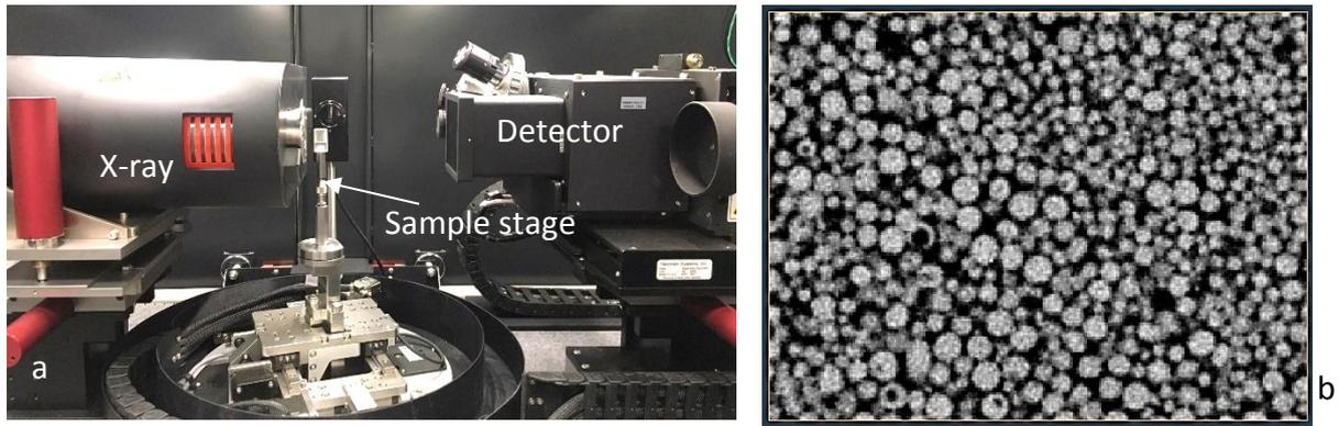
Figure 5. 2 XMT (a) set up, (b) reconstructed image of sample GA
