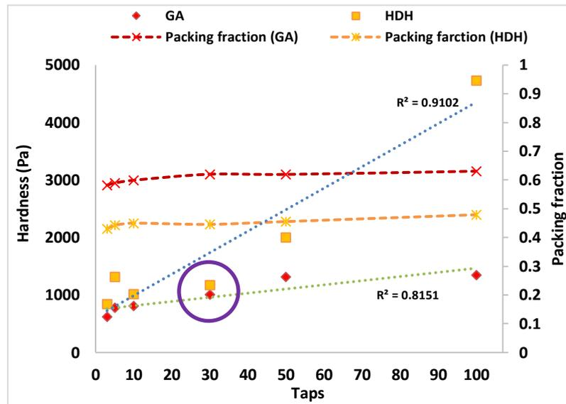
Figure 4. 12 The effect of number of tapping on hardness and packing fraction of GA and HDH powders
