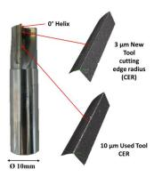
**Fig. 6.2.4.** Three flute Polycrystalline Diamond (PCD) Cutting Tool with Optical Edge Radius Measurements.
