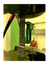
Fig. 3.4.4. Specimen breakage in tensile test with a fibre orientation of 90°.
