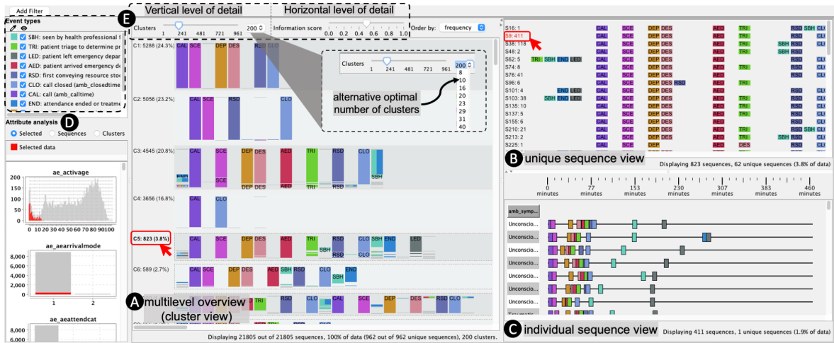
Figure 4.8: Sequen-C visualisation system. In the multilevel overview (A), cluster C5 is selected and its unique sequences are shown in the unique sequences view (B), where unique sequence S9 is selected, showing its 411 individual sequences in the individual sequences view (C). The attribute analysis (D) shows how attributes of the selected data relate to the whole dataset. (E) highlights some of the available controls.
