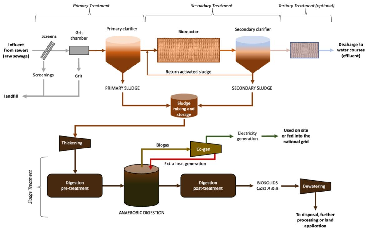
Figure 1-2: Wastewater treatment diagram, including the sludge treatment process and water treatment process. Blocks representing pre and post digestion treatments have been included to generalise this process flow diagram. There is likely to be pre or post-treatment as opposed to both. Depending on the post digestion treatment, dewatering may come before, for example, if the post-treatment is composting. Adapted from (Kor-Bicakci and Eskicioglu, 2019).
