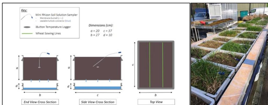
Figure 3-2: Monoliths set up, (left) schematic and (right) in situ photograph of monoliths at the University of Sheffield Arthur Willis Environment Centre, Sheffield, UK, taken January 2018.
