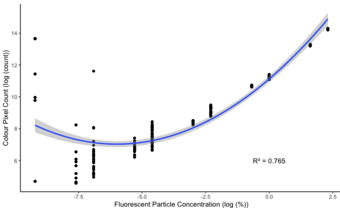
Figure 4-9: Calibration curve with zero samples removed (as  $\log 0 = \infty$ ) but all other samples included ( $R^2 = 0.765$ ,  $y = 11.12 + 1.37x + 0.11x^2$  where  $y = \log(\text{colour pixel count})$  and  $x = \log(\text{Fluorescent Particle Concentration})$ ,  $p < 0.001$ ).
