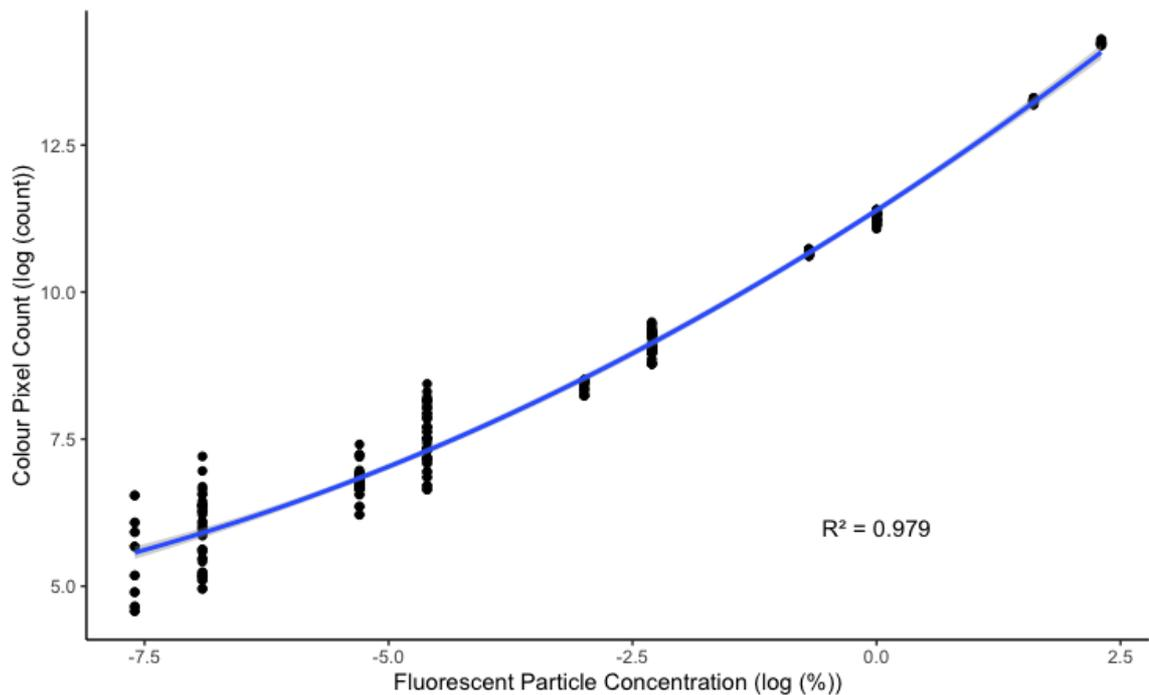
Figure 4-10: Calibration curve with samples containing noise removed, this included all the 0 % and 0.0001 % samples from the dataset, concentration, and the far outliers from 0.0005 % and 0.001 % concentrations. ( $R^2 = 0.979$ ,  $y = 11.39 + 1.07 x + 0.04 x^2$  where  $y = \log(\text{Colour Pixel Count})$  and  $x = \log(\text{Fluorescent Particle Concentration})$ ,  $p < 0.001$ ).
