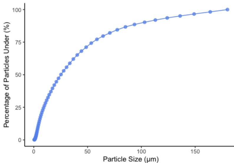
Figure 4-1: Biosolid particle size distribution. Biosolid and dH<sub>2</sub>O solution, passed through a 2 mm sieve and analysed in a liquid matrix particle size analyser (Malvern Panalytical Mastersizer/E laser particle size analyser).
