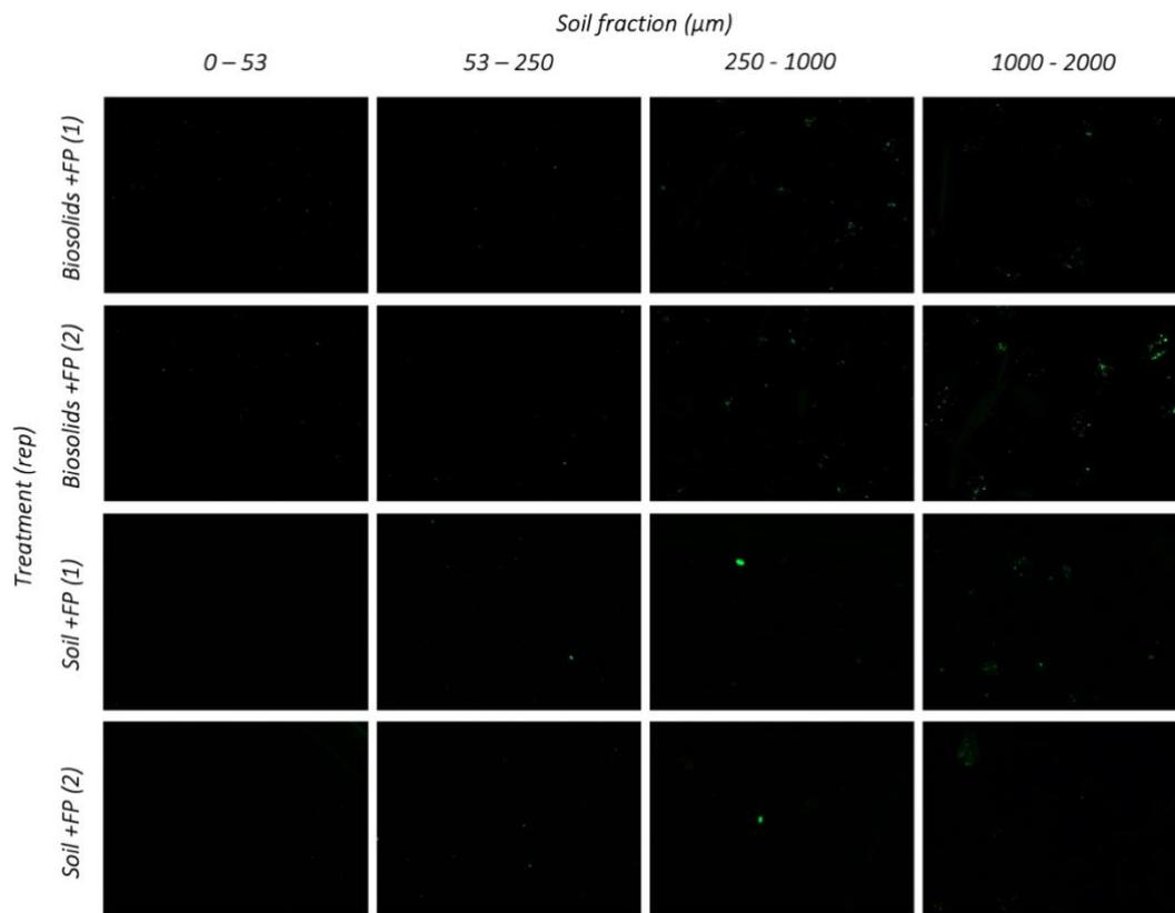
Figure 4-3: Example of the images from fluorescent microscopy from the 0 - 2.5 cm soil core from the Biosolids + FP applied and Soil + FP applied pot, 2 reps of each. Sample sieved to 4 aggregate size fractions and examined under fluorescence.
