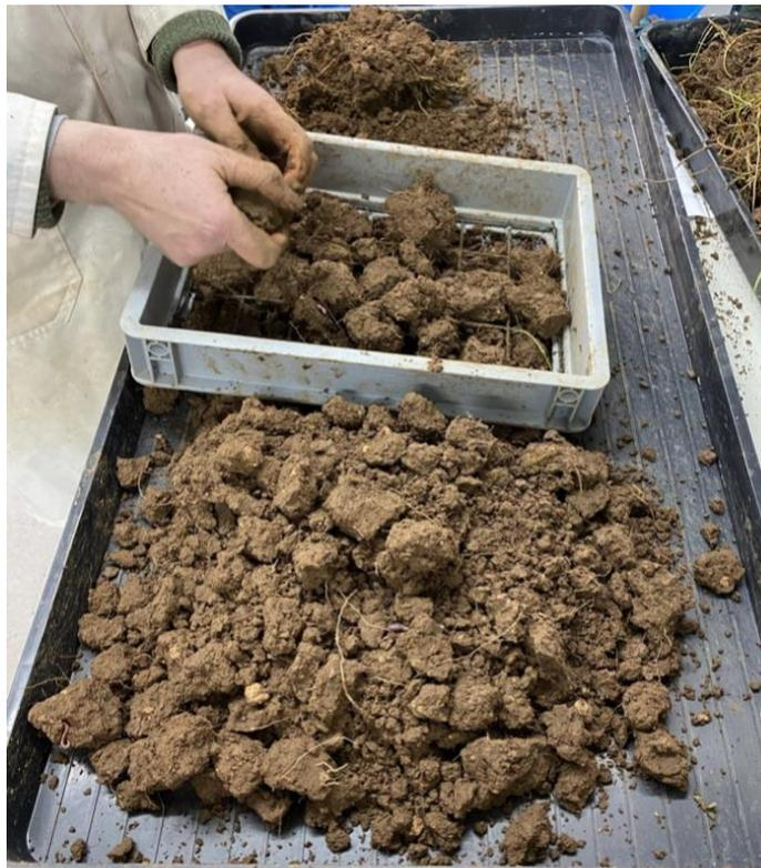
*Figure 5-2: Photograph of soil preparation using a coarse 5 cm sieve to separate soil from vegetation. Prepared soil can be seen in the foreground.*
