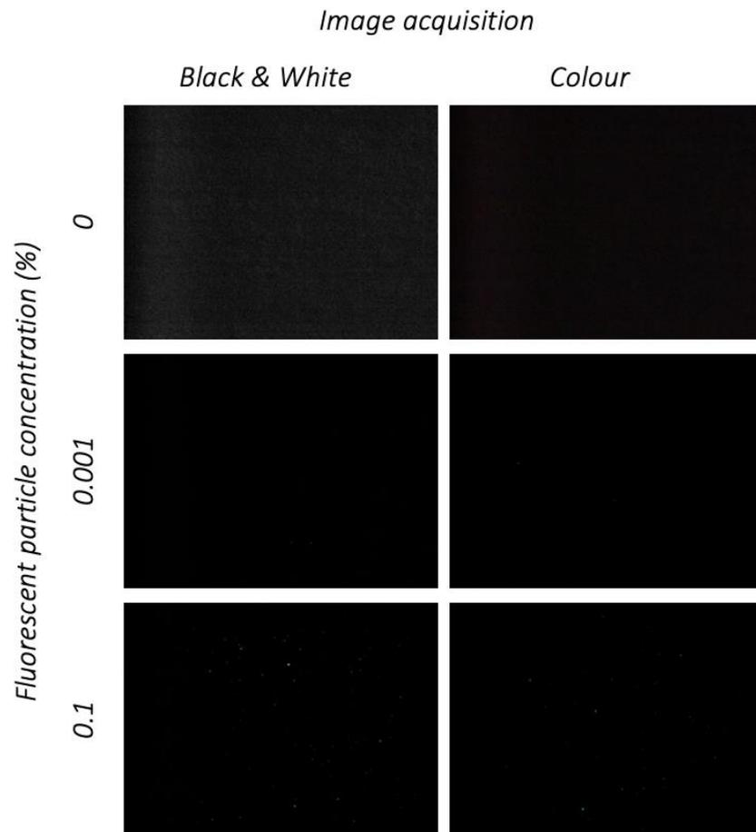
*Figure 4-7: Image acquisition trials. Black & white vs colour. Artificial noise can be seen in the black and white 0% fluorescent particle image. This was also seen in the colour capture of the same sample, although it is difficult to see in the figure.*
