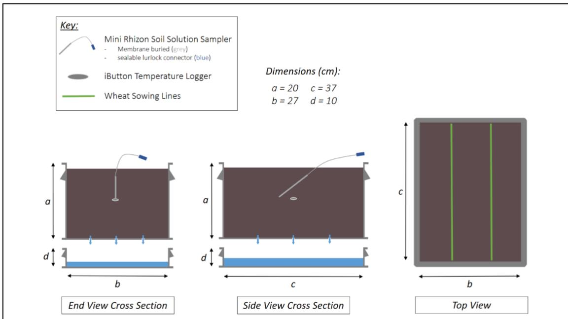
Figure 2-7: Schematic of monolith box set up. All monoliths had a leachate collection tray and mini rhizon soil solution sampler. One in every three monoliths had an iButton temperature logger representing a range of treatment. All arable cropping monoliths had wheat sown at twice the field density and thinned or made up to field density in March 2018.
