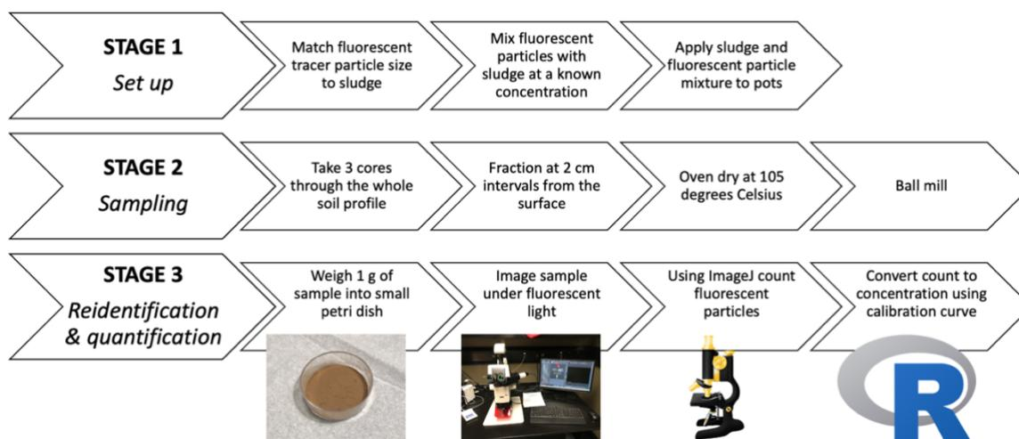
Figure 4-11: Workflow of the method development for the re-identification and quantification of fluorescent particles within a soil matrix.
