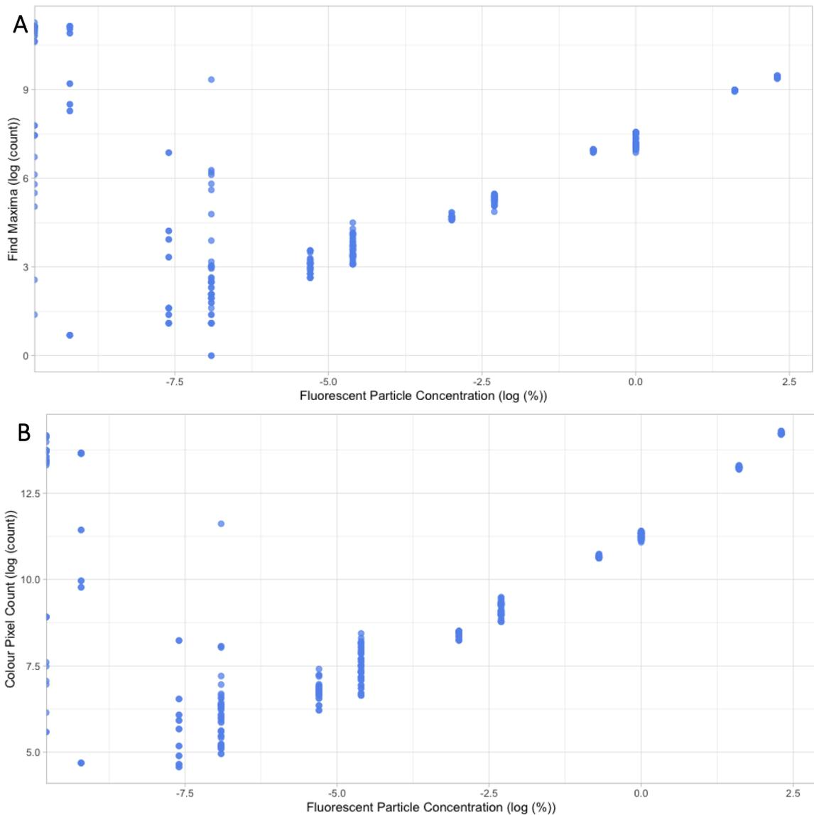
*Figure 4-8: Count data from different methods of image analysis using ImageJ to analyse the concentration of fluorescent particles from standard samples. Plot A) Count data from the Find Maxima tool, showing a more linear relationship before it dissolves into noise at the lowest concentrations. Plot B) Count data from the Colour Pixel Counter tool, the relationship appears to be quadratic and there is less noise towards at lower end of the concentration compared to that of plot A.*
