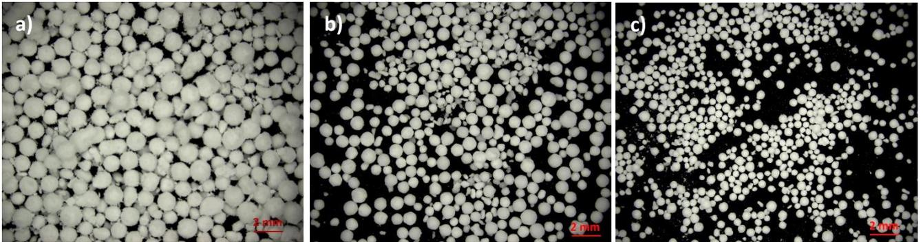
Figure 6.14. The influence of impeller speed on agglomerate size and morphology, at a TBSR of 0.75 with a 5 % solid loading. Conditions at a) 300 rpm, b) 500 rpm and c) 700 rpm.
