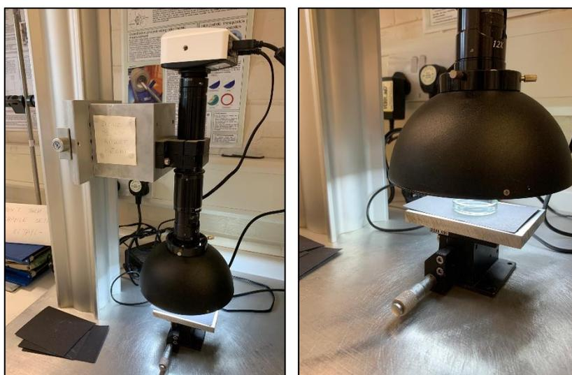
Figure 3.11. The experimental set-up of the Luminera Infinity 3 camera with 12 x zoom lens and LED light dome diffuser.
