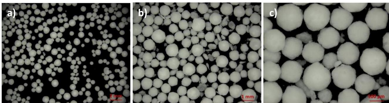
Figure 6.21. Observations of spherical agglomerates and fragments formed 100 minutes after bridging liquid addition.
