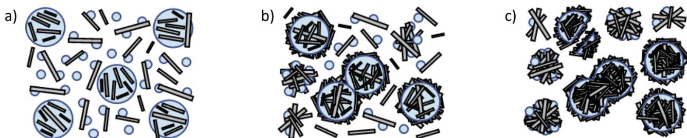
Figure 2.6. Mechanism for the spherical agglomeration method of spherical crystallisation. The bridging liquid is indicated by blue circles and crystals of interest by grey rectangles. Note, the solvent and anti-solvent are not shown in this schematic. Adapted from Mahanty et al., [36].
