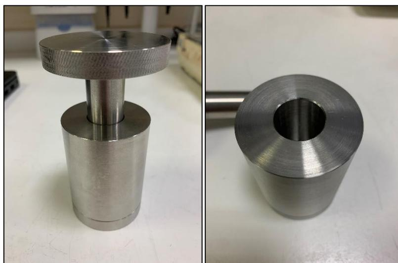
Figure 3.4. The die and press used to form tablets for contact angle analysis.
