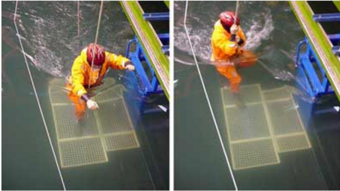
Figure 2.9. Photographs of a human subject in a flume tank subject to floodwaters with a depth of 1.07 m and a velocity of 1.0 \text{ m s}^{-1} . The human subject stands on a steel grate wearing safety clothing and equipment and has clear visibility in and out of water, all of which has the potential to influence their behaviour in simulated floodwaters relative to reality. Source: Karvonen et al. (2000: p. 49).
