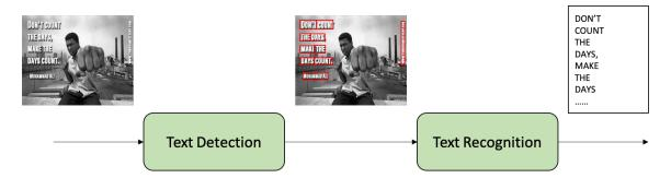
Figure 2.5: Overall architecture of an OCR system.
