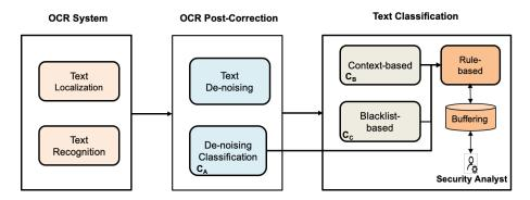
Figure 6.10: The Structure of the developed OCR-based Detectors
