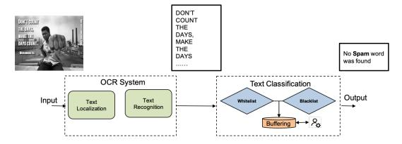
Figure 5.4: Overall architecture of our adversary-aware OCR-based detector. It consists of three models: text detection based on PixelLink, word recognition using CRNN, and a proposed text classification model.
