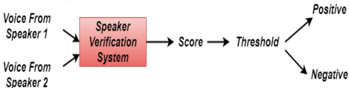
(a): The diagram of a speaker identification system
