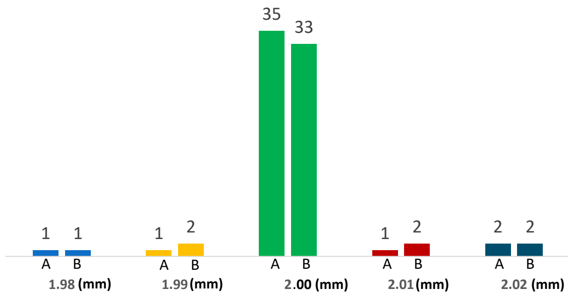
Figure 3.19 - An illustration of the repeatability of the pre-crack with the new methodology with measurements taken from both sides (A and B) of each specimen.
