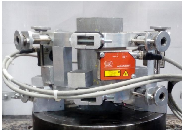
Figure 3.3: Measuring device for axial deformation
