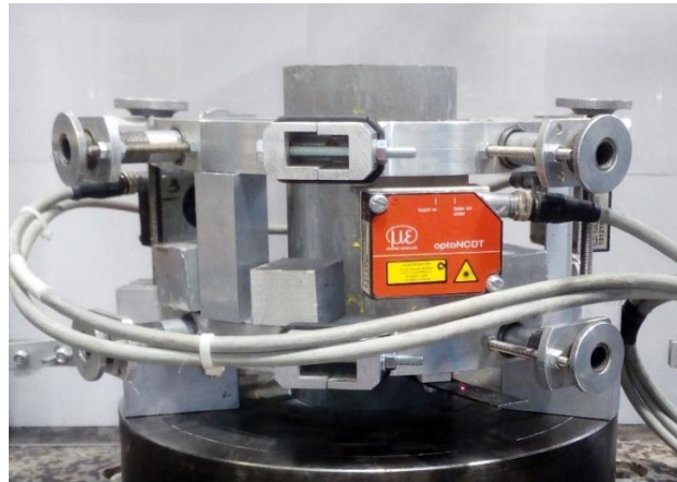
Figure 4.3: Measuring device for axial deformation
