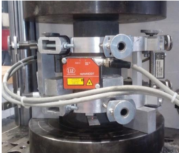
Figure 2.6: Compressive strength and modulus of elasticity test.
