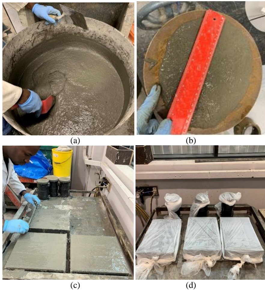
Figure 2.5: UHPC production (a) Fresh E-UHPFRC mix (b) workability test (c) casting and levelling (d) cast prisms and cylinders
