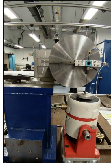
Figure 6.16: Flywheel inerter experimental set-up
