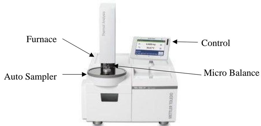
**Figure 3.15: Mettler TGA instrument**
