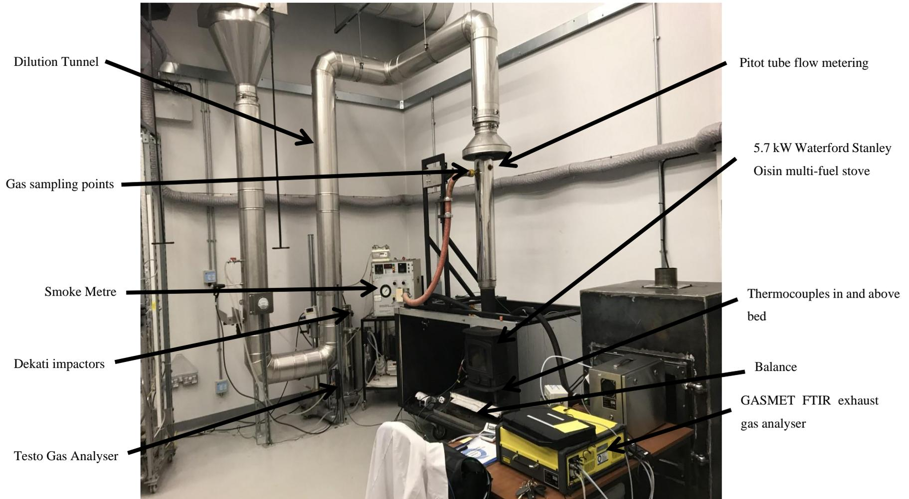
**Figure 3.22: Stove combustion lab setup**
