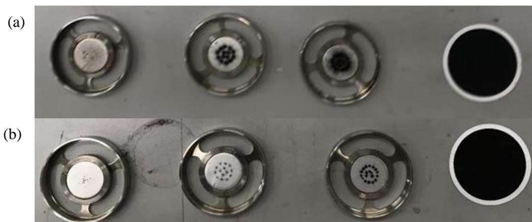
**Figure 5.7: Impactor foils and filters for a) commercial coffee logs b) willow wood logs**
