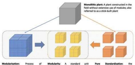
modularisation: Process or converting the design and construction of a monolithic or stick-built plant to facilitate factory fabrication of modules for shipment and installation in the field as complete assemblies Modularity: A standard unit assembled onsite from factory produced modules, usually of smaller capacity than a monolithic plant, to maximize the benefit from modularity effects
