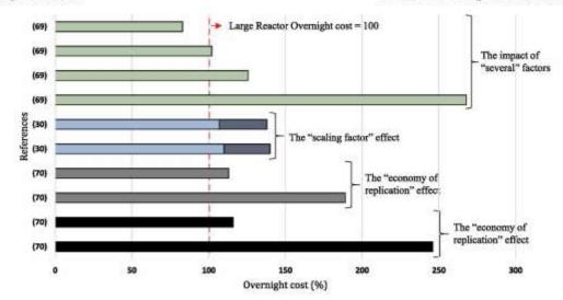
The highest SMR OVC is obtained scaling up from an estimation of an LR OVC without considering other factors. The following OVCs are obtained including the following factors sequentially in the comparison: design simplification and schedule reduction, additional learning determined by factory fabrication that determines a 40% NOAK cost reduction applied to indirect components, contingency, and owner's cost, and the learning curve applied to all components.
