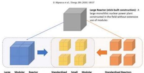
Large Modular Reactor (modularisation): A nuclear power plant assembled onsite mostly from factory produced modules
