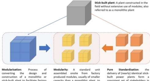
stick-built plant to facilitate factory fabrication of modules for shipment and installation in the field as complete assemblies
