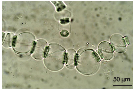
Figure 1.9: The swelling and ballooning of wood fibers in the solvent N-Methylmorpholine N-oxide. Credit: Singh et al. [68]
