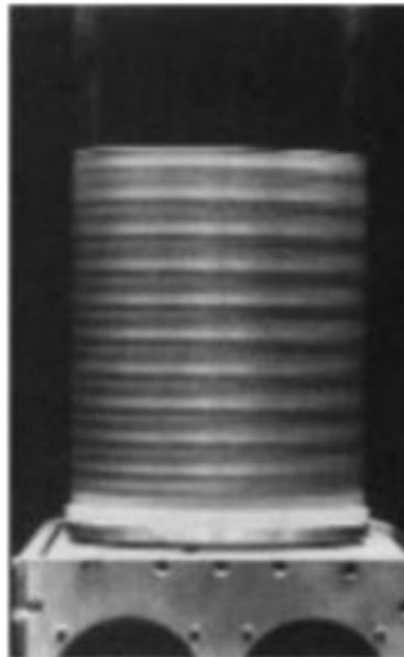
Figure 2.16: A photograph of Taylor-Couette flow in two concentric cylinders. Photograph taken from Stewart and Golubitsky (2011) 90
