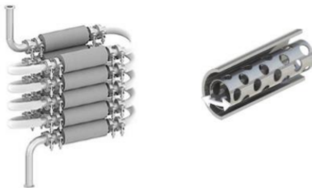
Figure 2.21: (Left) A diagram of a ten tube agitated tube reactor. 111 Fluid passes through up to ten tubes via an inlet at the top of the array and flow through the tubes sequentially until leaving the reactor via an outlet at the bottom. Tubes are modular and can be added or removed as necessary. (Right) A diagram of the interior of a tube. 111 Each tube contains a free-moving agitator bar. As the ATR is subject to lateral shaking, the bars are forced to move, agitating the liquid flowing through the tube.
