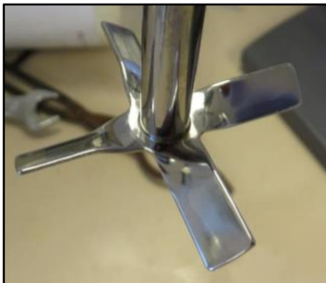
Figure 3.9: The impeller attachment used during back-extraction of Cu(II) from the Cu(II)·2L complex in the pre-used Mextral ® 84H.
