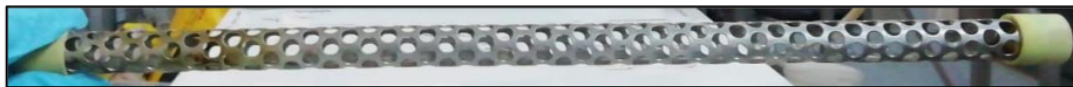
Figure 5.6: The agitator bar in the ATR tube. Motion of the bar influenced by the shaking of the ATR causes the two liquids to disperse. This is facilitated by the holes along the length of the bar. The feet on the each end of the bar raise it from the base of the tube to prevent damage.
