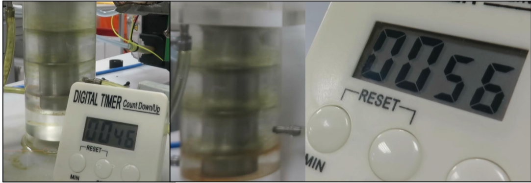
Figure 4.6: Frames from rise time measurement videos. (A) A digital timer sits in the foreground of the TCDC to measure the amount of time coloured tracer material remains in the TCDC. (B) A digital timer is used to measure rise time in the D-cell contactor.
