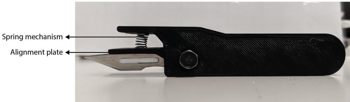
Fig. 3.19 Actual snapshot of the in-house, 3D printed and assembled cross-cutter, highlighting the alignment plate used to maintain the planar alignment of the blades, and the spring mechanism to ensure a constant pressure is applied during the testing procedure.
