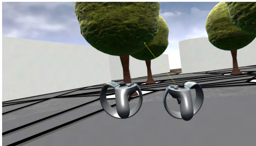
Figure 6.3: Controllers and yellow line traced to indicate the location that the user is pointing.
