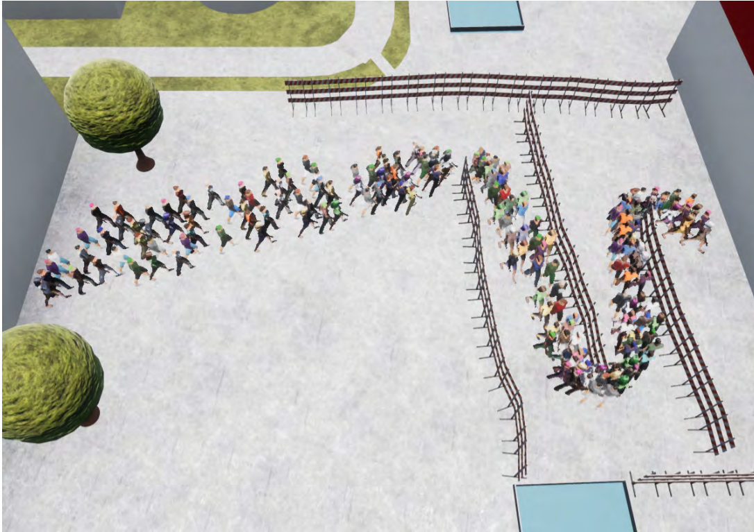
Figure 3.34: Pedestrians adjusting their path after the user created a corridor by sketching barriers.
