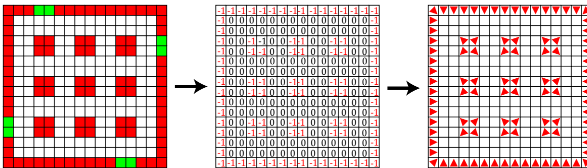
Figure 3.11: (Left) Initial grid obtained from the environment. (Centre) Two-dimensional array where ‘-1’ indicates obstacles and ‘0’ walkable areas. (Right) Final collision map after computing the force of each cell.
