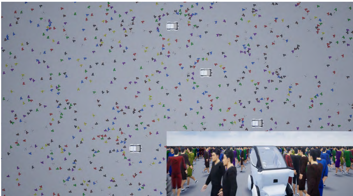
Figure 2.2: Zoomed-in section of 2,500 agents crowd visualised in Unreal. Four groups navigate in opposite directions, two moving from left to right and two heading between top and bottom. Top: scene view from above showing agents and autonomous vehicles; Inset: shows an eye-level view of the simulation
