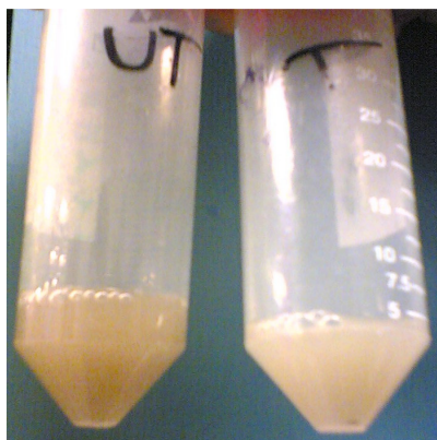
Figure 7-18 picture shows the digested sludge sample before treatment (UT) and after treatment (T);
