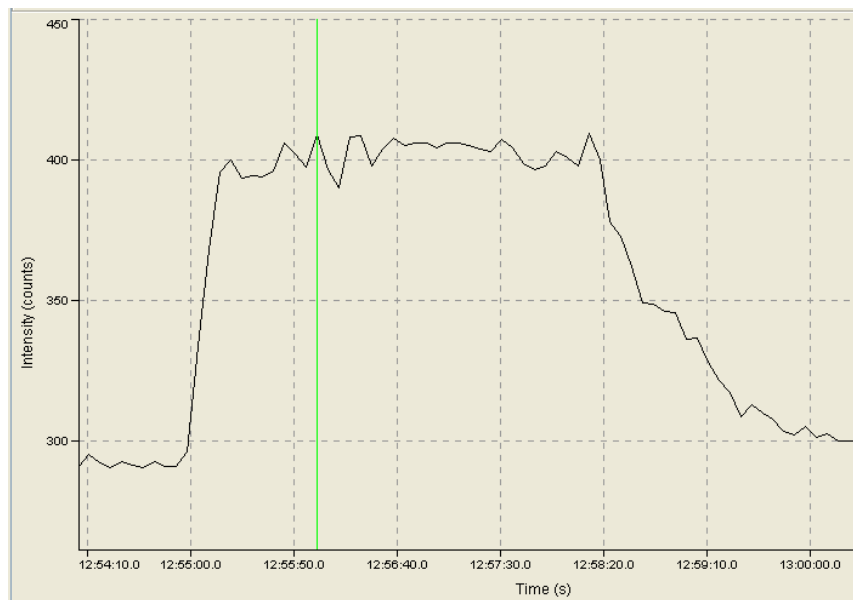
Figure 5-5 the signal recorded during mercury experiment; (A) the recorded spectrum, (B) strip chart showing the signal versus time
