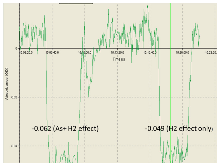
Figure 6-31 a strip chart recorded for the arsenic absorbance signal; The signal recorded upon injecting 10 \mu\text{g/L} arsenic at 1.3 \text{ M HCl} and 1.5\% \text{ m/v NaBH}_4 . The difference between the recorded signals ( 0.013 ) is proportional to the amount of analyte injected.
