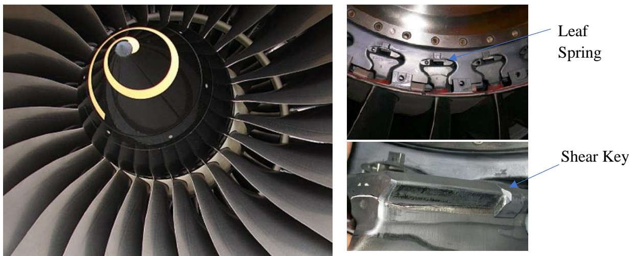
Figure 2-1: Fan assembly (left). Fan blade dovetail connection (top right) and fan blade root (bottom right) [1]
