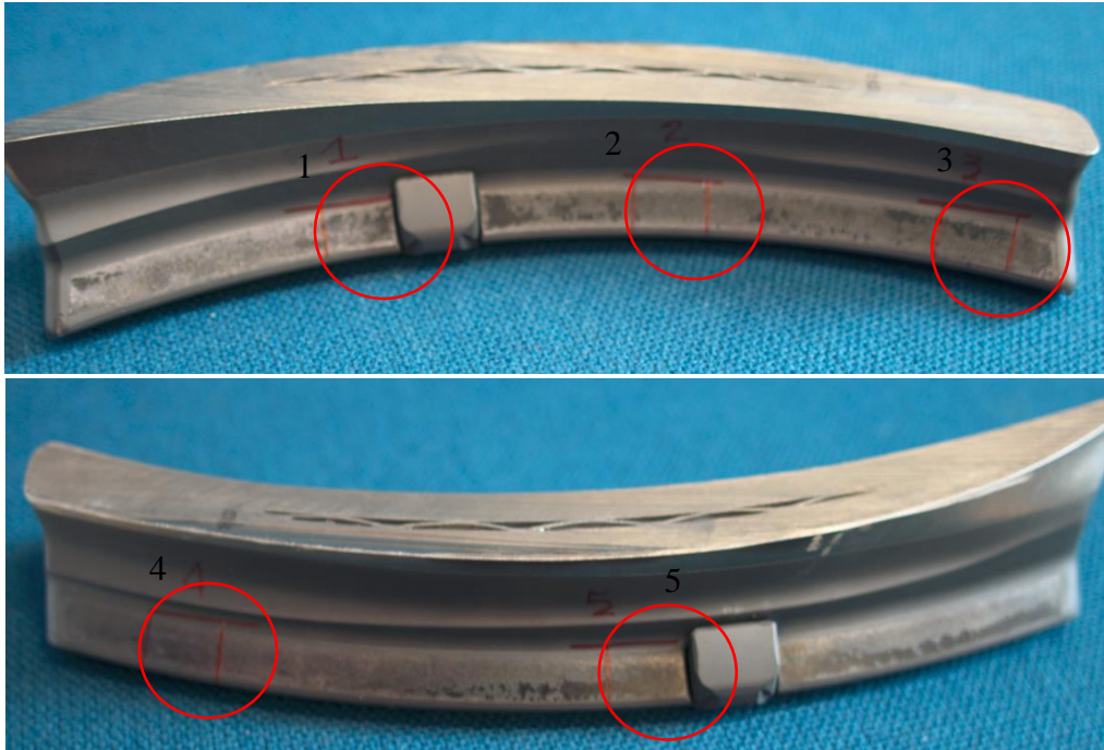
Figure 3-6: Fan blade cut positions (marked in red). Intrados (above) and extrados (below).
