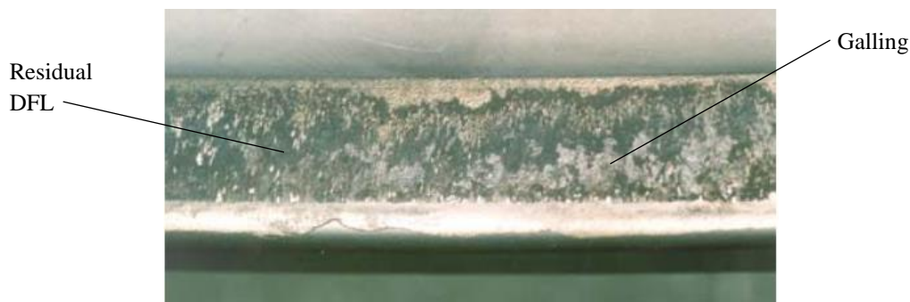
Figure 3-1: Rolls-Royce RB211 Trent 892 blade dovetail root inspected by the ATSB [10].
