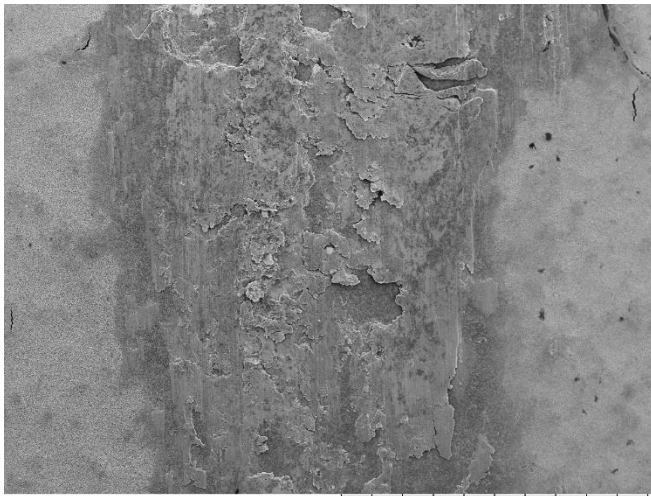
Figure 0-2: Blade surface: 300MPa, 150µm, 10 kcycles.
