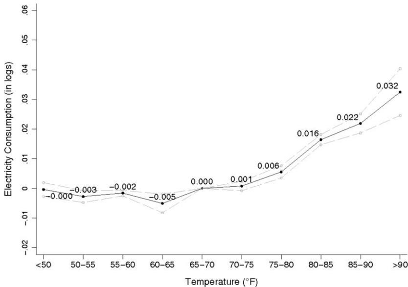
**Figure 2-3 Application of temperature bins method for Mexican residential electricity consumption** Source: Davis and Gertler (2015)
