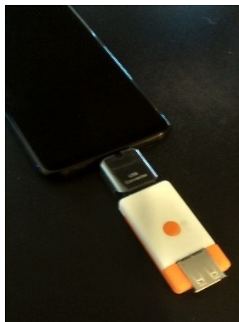
(b) Phone with USB on-the-go (OTG) adaptor
