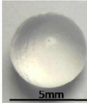
**Fig. 2.22: Calcium alginate beads produced by dripping method; pure alginate in gel state [90]**
