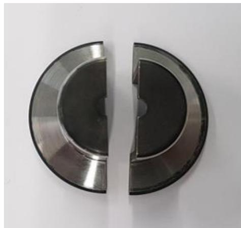
*Figure 85 Collets for sub-size tensile specimens produced for this project*
