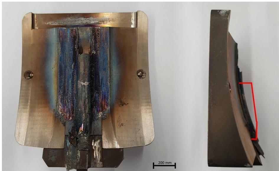
Figure 61 Photograph showing an example of abutment wear during a Conform™ trial.
