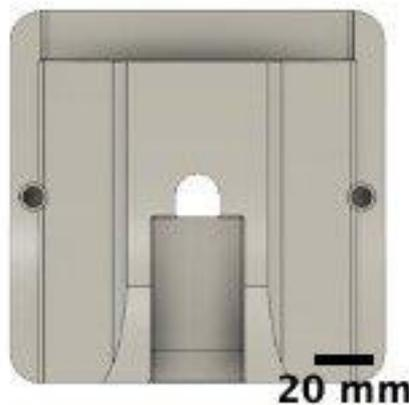
*Figure 36 CAD drawing of the die chamber.*
