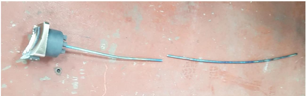
*Figure 74 CP Ti HDH Gr 2 and Ti-6Al-4V swarf derived wire produced during Trial 10.*
