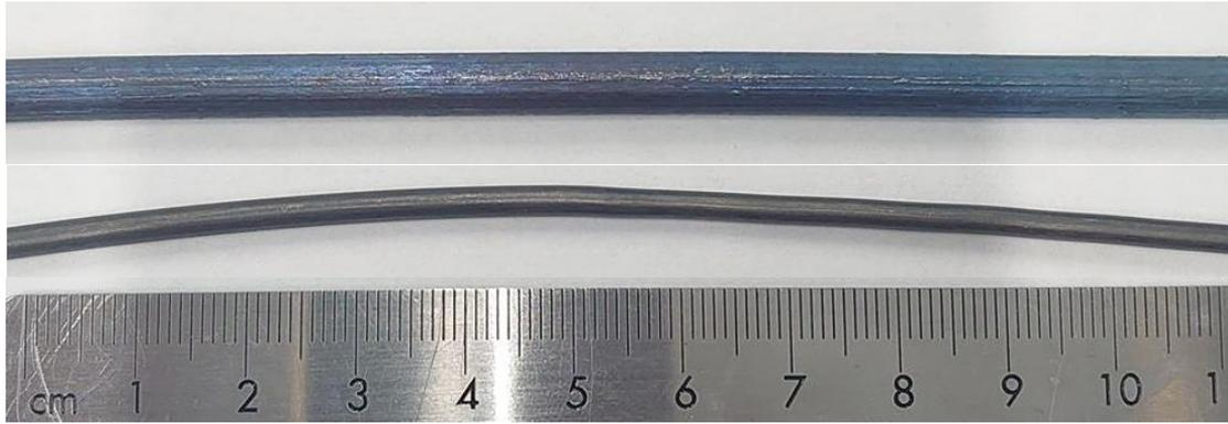
Figure 95 Photograph of as-Conformed CP-Ti Gr 2 wire with blue oxide film (top) and  $\phi$  3.00 mm cold-wire drawn wire with bright surface (bottom) from the same extruded product.
