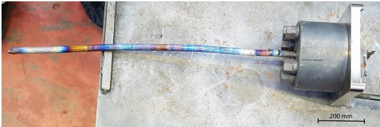
*Figure 72 Photograph of CP Ti HDH Gr 2 rod extruded through the die during the Conform process from trial*
