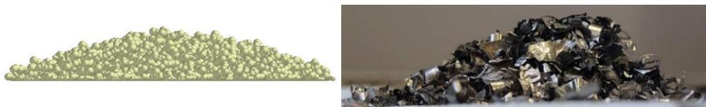
Figure 44 (a) Simulated Angle of Repose for Ti-6Al-4V swarf particles; (b) Experimental Angle of Repose for Ti-6Al-4V swarf.
