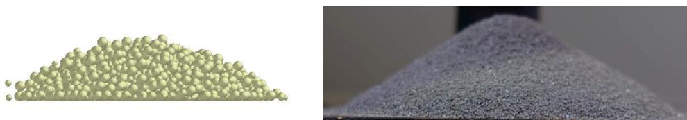
Figure 42 (a) Simulated Angle of Repose for Ti-6Al-4V GA particles; (b) Experimental Angle of Repose for Ti-6Al-4V GA particles.
