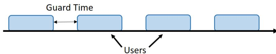
Figure 3.2. Time Division Multiple Access (TDMA).
