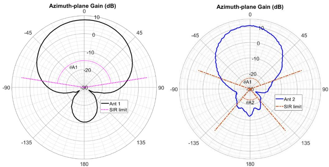
Figure 4.5: Polar plot of the antenna pattern of Ant 1 and Ant 2.
