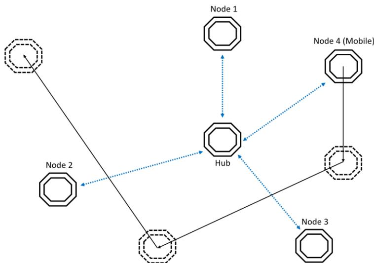
Figure 4.1. Riverbed Modeler project model design example, where the blue lines indicate the communication link and the black line represents the trajectory of the mobile node.
