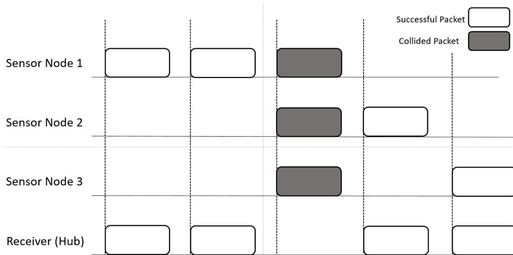
Figure 3.7. An example of packet reception with Slotted Aloha Protocol.
