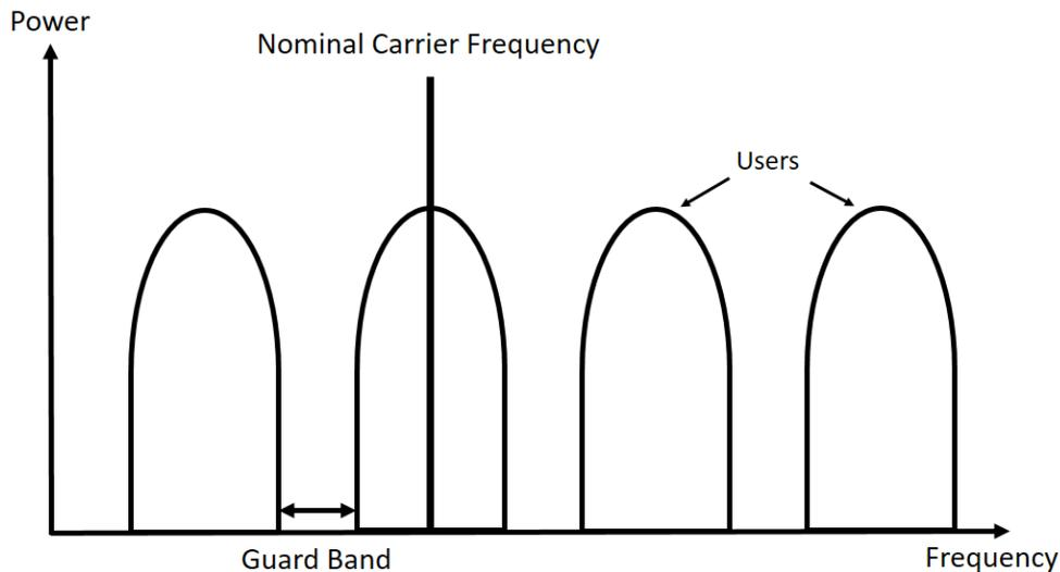
Figure 3.1. Frequency Division Multiple Access (FDMA).
