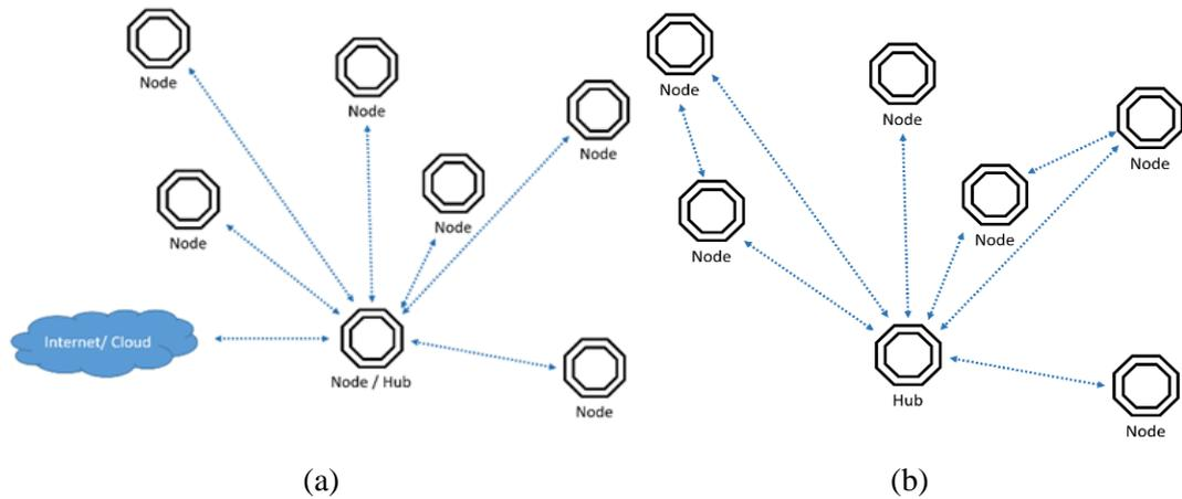
Figure 2.1. Different types of network architectures.
