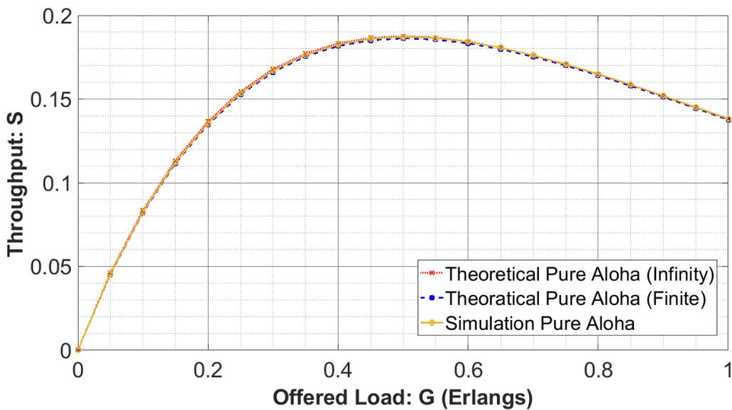
Figure 5.4. Pure Aloha throughput 50 sensor nodes.
