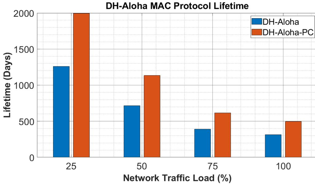
Figure 6.2: Comparison of expected sensor node lifetime with DH-Aloha MAC protocol variants.
