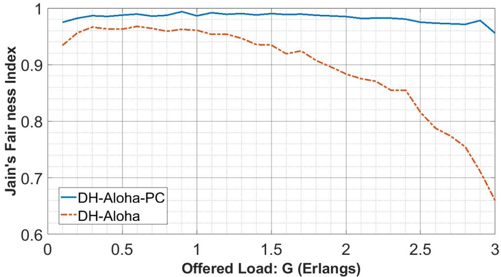
Figure 6.5: Jain's fairness index with the power control strategy applied in a WSN with 50 nodes.
