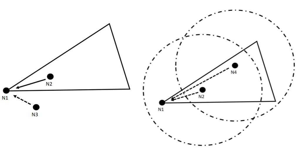
Figure 3.9. The new deafness problem (left) and the new interferer problem (right) for directional MAC protocols.
