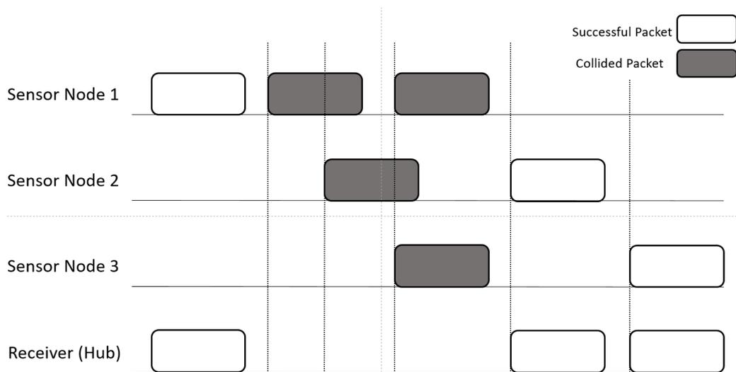
Figure 3.6: An example of packet reception with the Pure Aloha Protocol.
