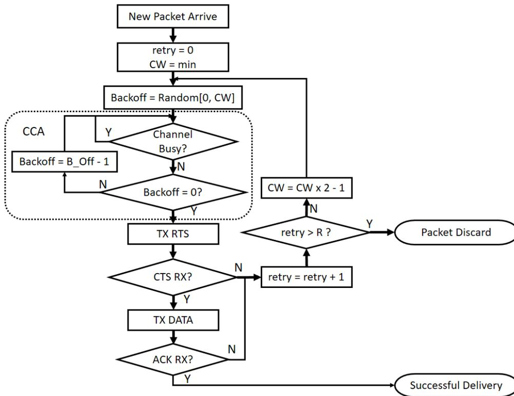
Figure 3.8. CSMA/CA/DCF channel access procedures.
