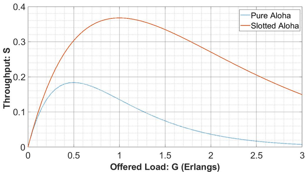
Figure 5.1. Theoretical throughput performance of Pure and Slotted Aloha.
