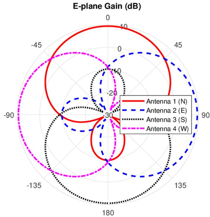
Figure 5.13: Polar plot of antenna E-plane patterns showing the extent of overlap.
