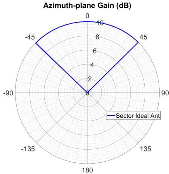
Figure 4.4. An example polar plot of an ideal sector directional antenna with a beamwidth of  $90^\circ$ .
