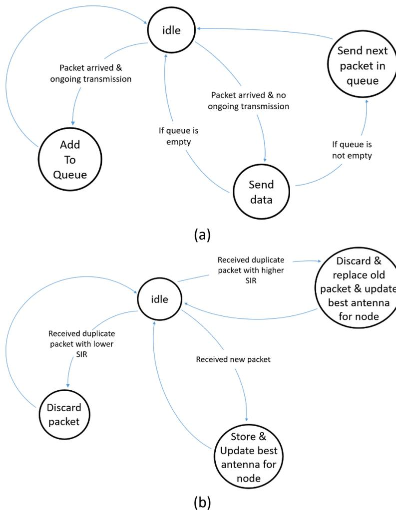
Figure 5.6. DH-Aloha system state diagram (a) sensor node, (b) hub node.
