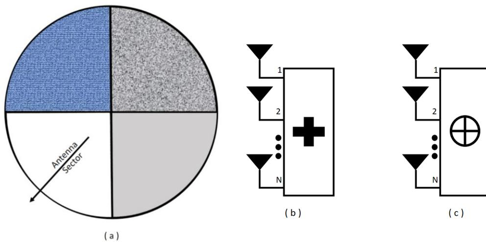
Figure 3.3. Directional antenna model, (a) Antenna sectors, (b) Adaptive array function, (c) Switch based function.
