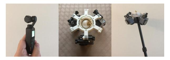
Figure 86, photogrammetry equipment. DJI Osmo Pocket (left), custom action camera rig (middle & right)
