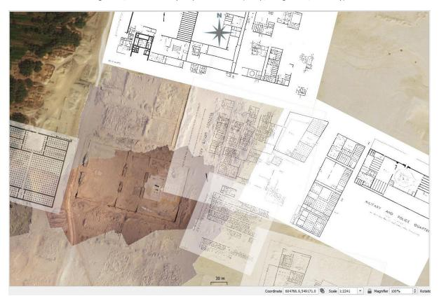
Figure 23, a selection of orthographic photography and georeferenced plans at different transparencies to show layering.
