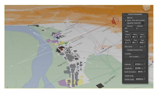
Figure 159, view of the sunlight system in 3dsmax using a proxy map for initial setup
