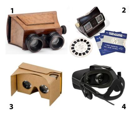
Figure 6, the evolution of stereo head mounted displays: (1) Brewster Stereoscope (CC BY-SA), (2) Sawyer's View-Master (CC-0), (3) Google Cardboard (CC-0), (4) Oculus Rift (CC-0)
