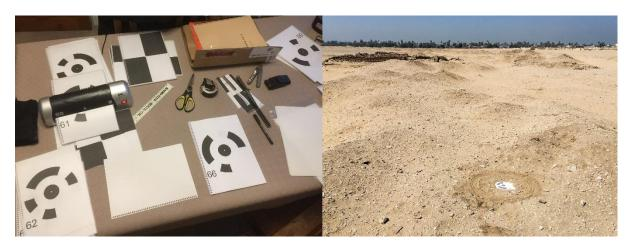
Figure 85, photogrammetry markers being prepared (left) and in use (right)
