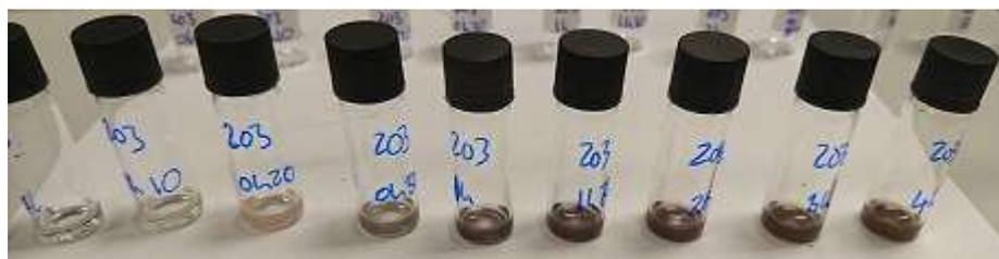
Figure 3.11: Photograph depicting samples of crude reaction mixture drawn off from the diglyme-solvated DCC protocol between **1a** and **2a** at 100 °C, utilising PdAu-PVP as catalyst. From left to right the samples were drawn at time (hours:minutes) = 0:00; 0:10; 0:20; 0:30; 1:00; 1:30; 2:00; 3:00 and 4:00.
