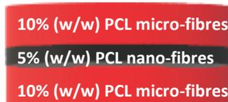
**Figure 6.2.3:** Schematic of the final tri-layered scaffold created with three layers: microfibers (red), nanofibers (black), and microfibers. These layers are made from poly (caprolactone) with different concentrations.
