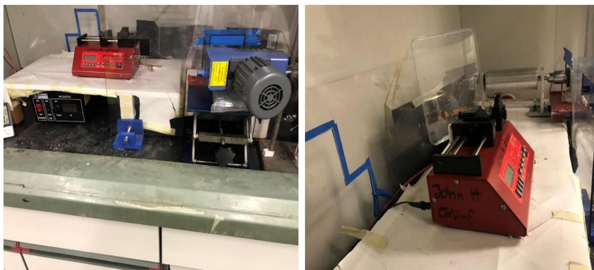
**Figure. 2.2.8:** The electrospinning apparatus used to produce the 3D electrospinning PCL scaffolds as discussed in Chapter 1.
