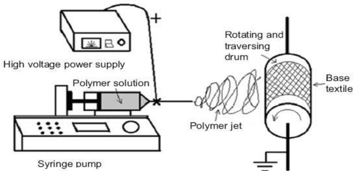
**Figure. 1.13.4:** Schematic of electrospinning machine <sup>(8)</sup> illustrating the components described in section 1.13.4.
