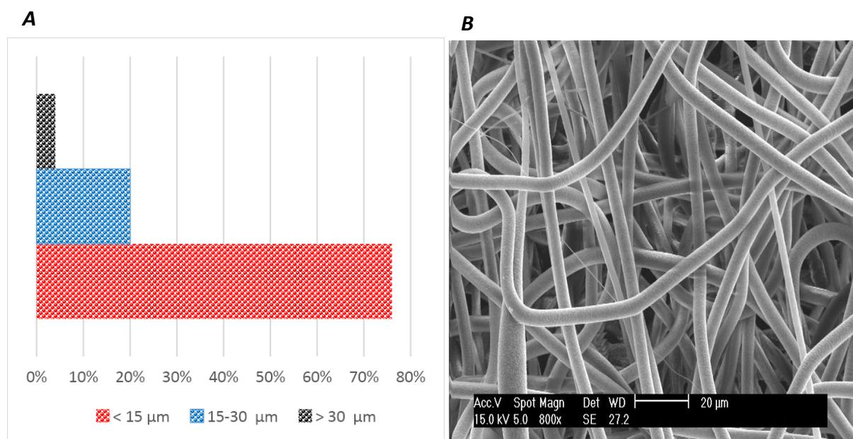
**Figure 5.3.1:** 10wt% PCL electrospun scaffold characterisation; A: the percentage of fibres at different diameter ranges B: SEM image of electrospun fibre morphology and diameter. The polymer pellets were dissolved in DCM and spun in the 40 $\mu\text{L}/\text{min}$  flow rate, 17kV, 17cm working distance, 300 rpm (rotating collector). Scale bar = 20 $\mu\text{m}$ .
