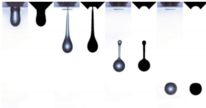
Figure 1.3: Comparison of drop formation in axisymmetric simulations and large-scale experiments, where the nozzle diameter is 2 mm. Reprinted figure with permission from Castrejón-Pita et al. (2011) Copyright 2011 by the American Physical Society.
