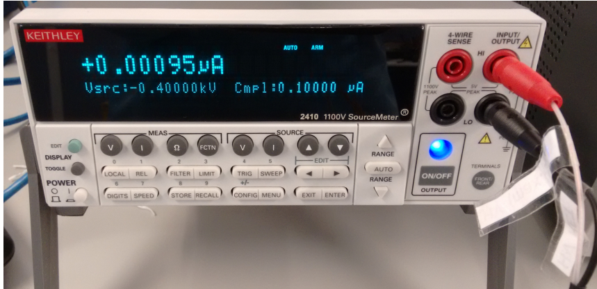
Figure 6.3.6: Photograph of a high-voltage power supply delivering a negative bias to the module sensor, as a means to suppress noise during the DAQ testing.
