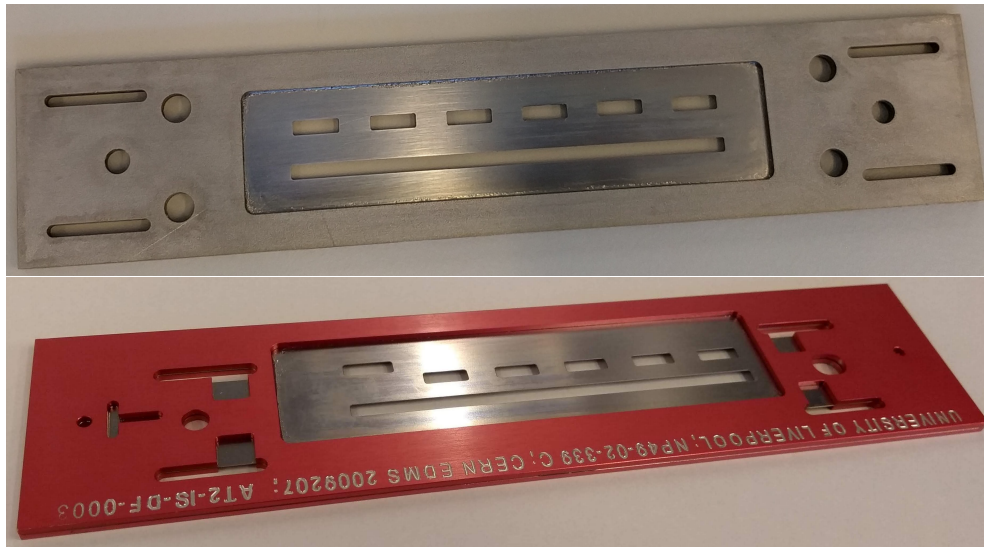
Figure 6.2.10: Photographs of the module-sensor gluing stencil, used in older ABC130 designs (top) and the latest ABCStar (bottom).
