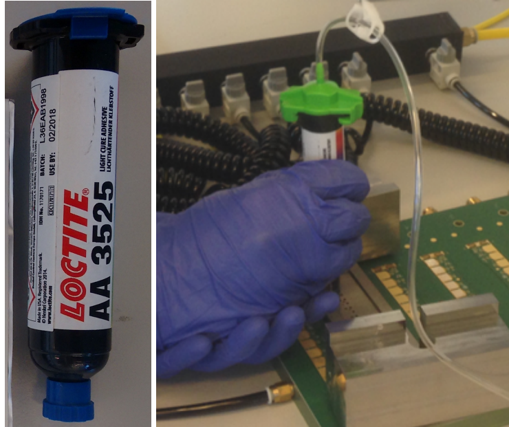
Figure 6.2.7: Photographs of the UV glue-dispensing container (left) without its needle, and the process of the glue being pneumatically-injected through the hybrid stencil (right), with the exception that this photograph features an earlier trial where the glue was placed on the hybrids rather than the chips.
