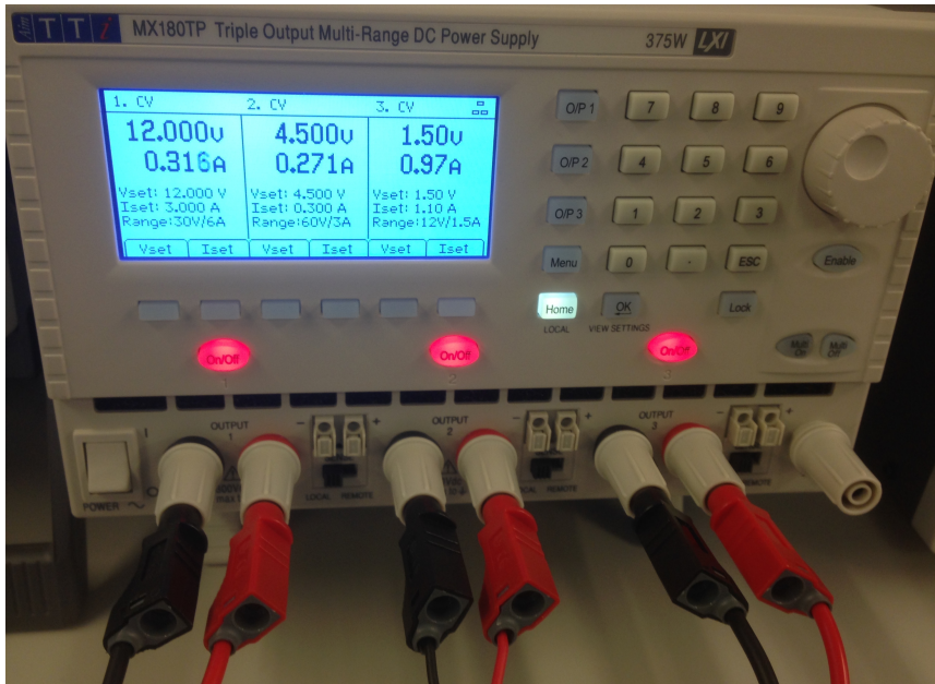
Figure 6.3.2: Photograph of a low-voltage power supply delivering power to the various components within the DAQ testing system. From left to right, the channels shown are powering the Nexys FPGA, the SLVS buffer board and a single hybrid-on-panel.
