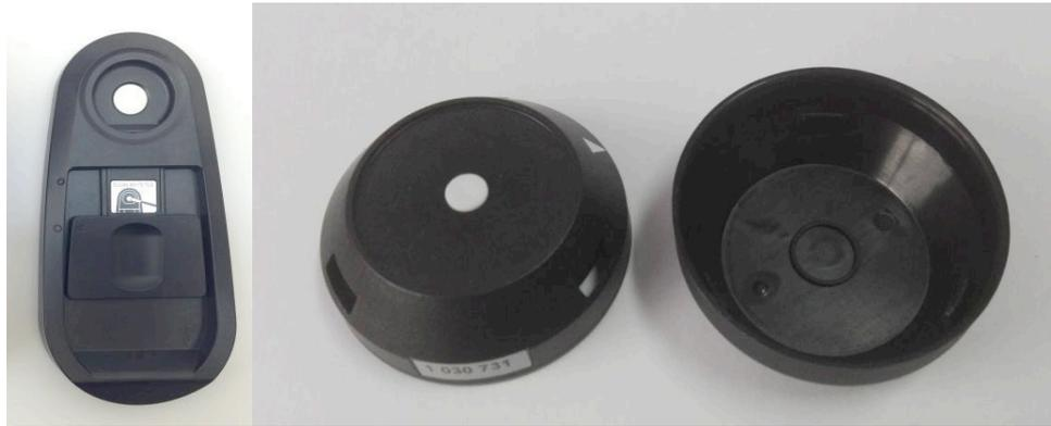
**Figure 3.1.4:** i1 Pro 2 calibration white tile (left) and illumination head (right)
