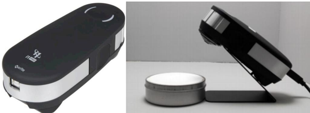
**Figure 3.1.3:** i1 Pro2 and measurement geometry
