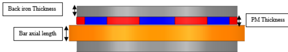
Fig 4. 1 Schematic of an axial single sided squirrel cage PMECC
