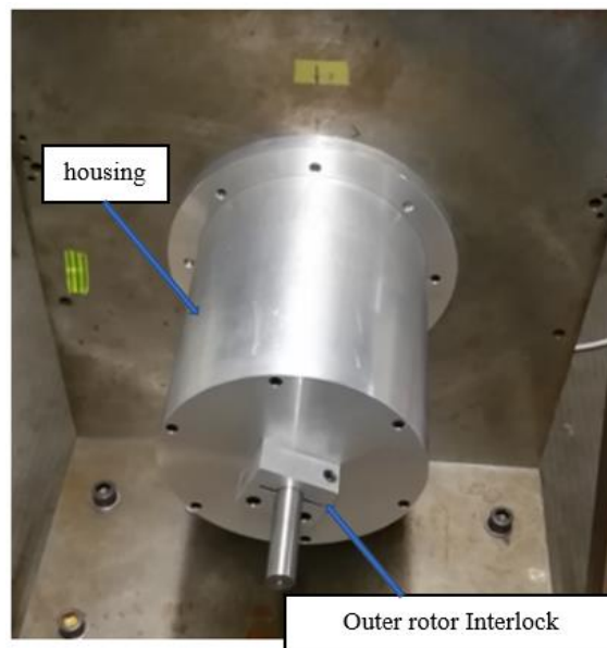
Fig 6. 8 Interlock of the outer rotor.
