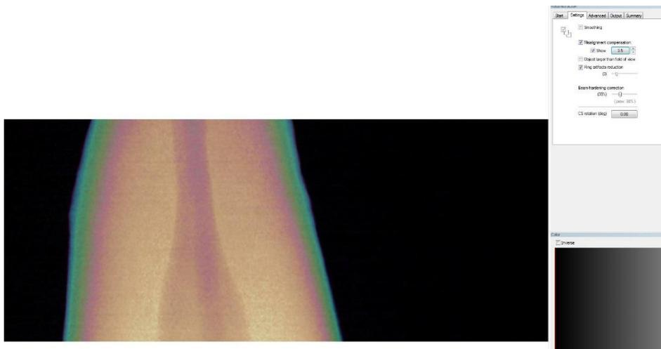
**Figure 2-** NRecon parameters selection and preview image of the root to ensure no rings or mishaps will be shown in the root slices image.
