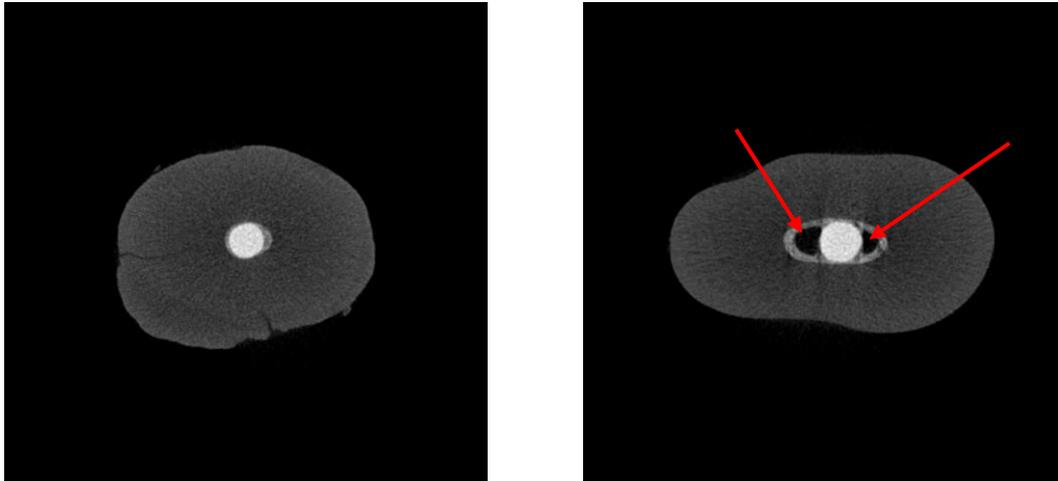
**Figure 15-** Two middle third's slides (high and low voids volumes) of samples obturated with MTA Fillapex sealer, red arrows point for voids within obturation
