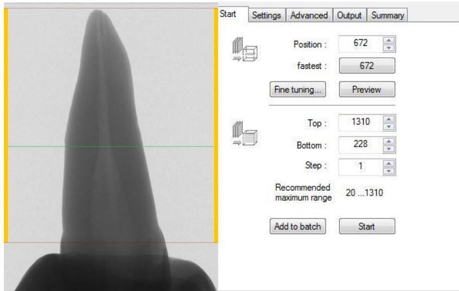
**Figure 1-** NRecon reconstruction of the entire tooth, bottom line placed near the CEJ while top line should be placed at the end of radiographic apex.
