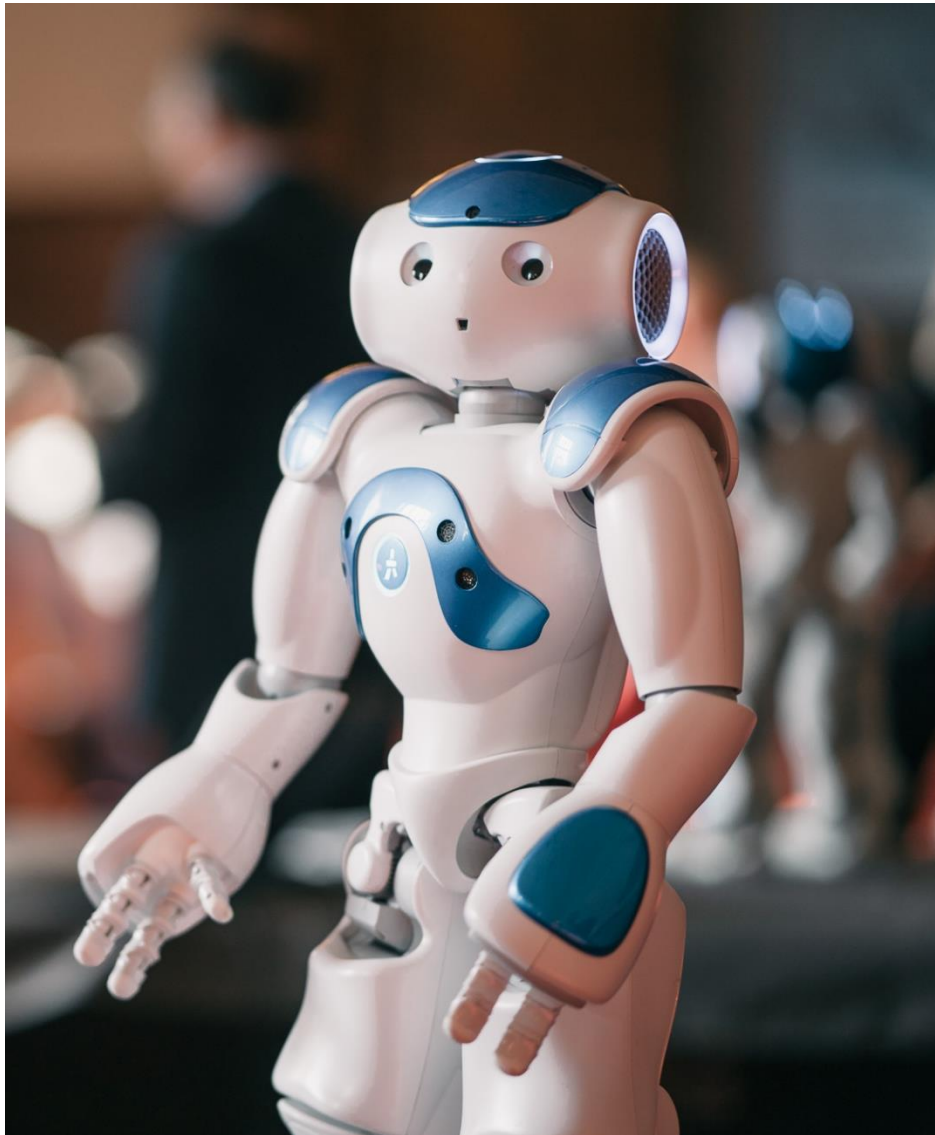
Figure 15: The humanoid robot NAO. Height: 57cm.
