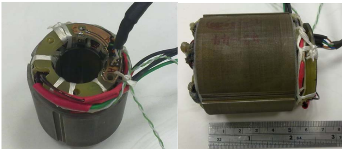
Fig. A.12 Stator of the tested motor.
