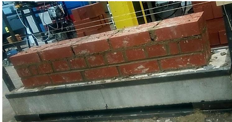
Figure 4.30. Wall specimen bonding pattern (image during construction)
