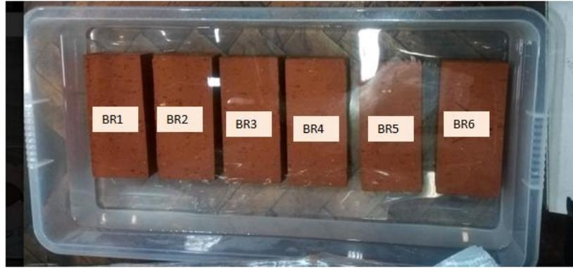
Figure 4.2. Brick samples immersed in water
