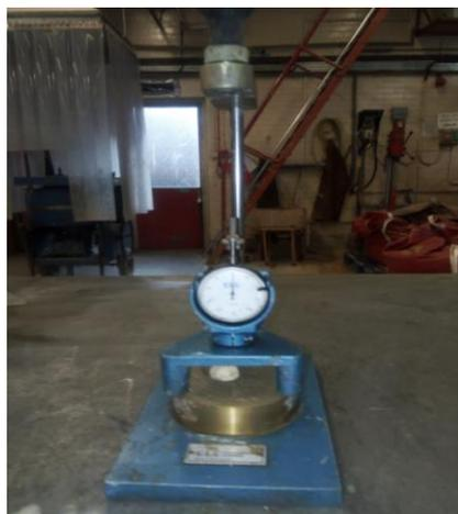
Figure 4.7. Test setup for dropping ball test
