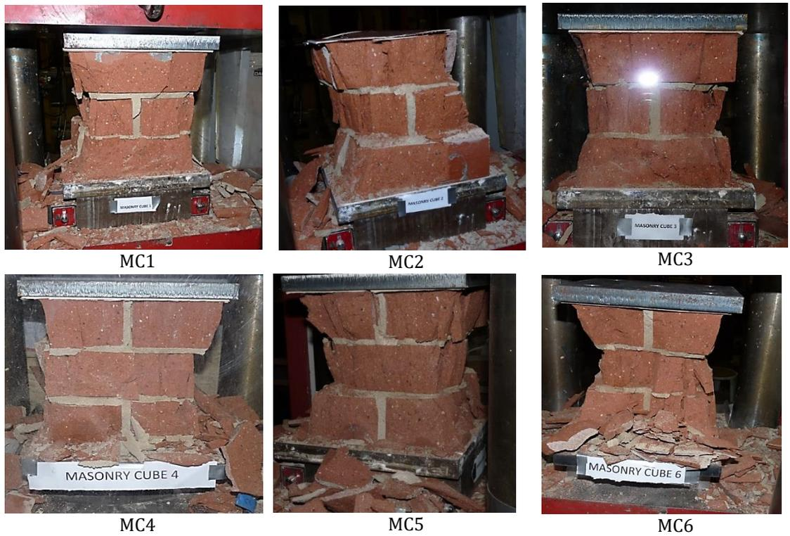
Figure 4.14b. Failure of masonry cubic specimens
