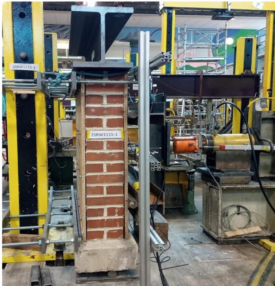
Figure 4.34a. Larger-scale test arrangement (Side view showing the general arrangement)
