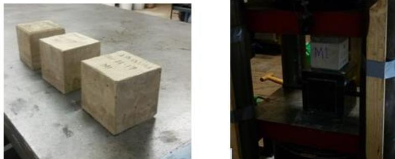
Figure 4.9: Compressive strength test of hardened mortar
