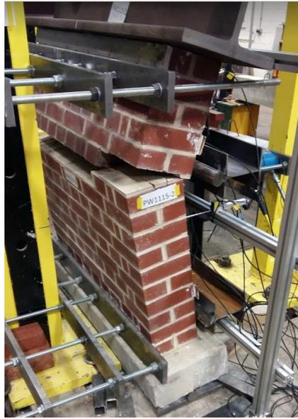
Figure 4.39. Failure pattern of PW1115-2
