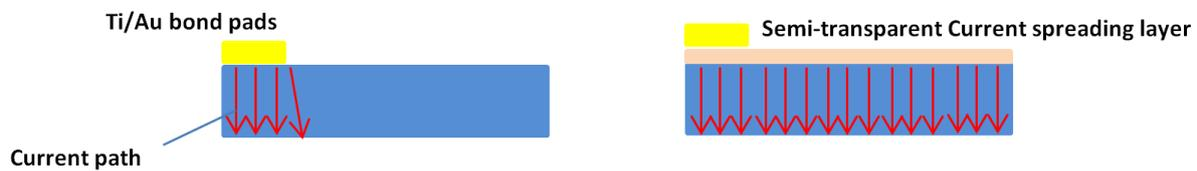
**Figure 3.8** Schematic illustration of current path a) without current spreading layer and b) with current spreading layer.
