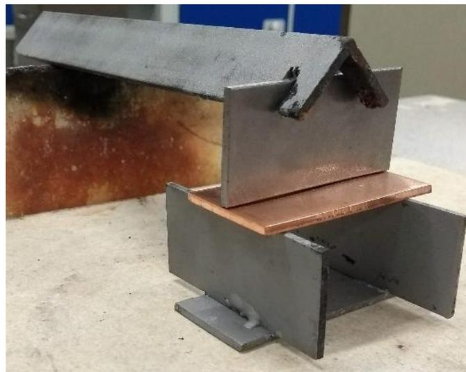
**Figure 3.2: A photograph of the metal coupon arrangement held in place using jigs before the filler metal or flux paste is applied.**
