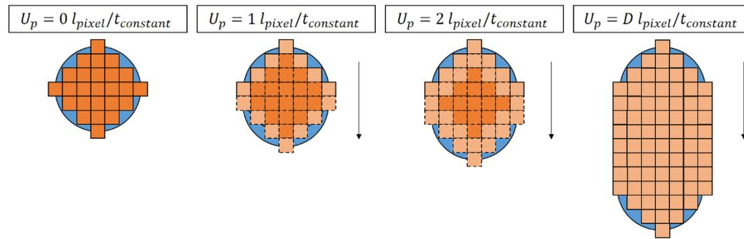
Figure 27. Blurry particles caused by the movement of the particles.
