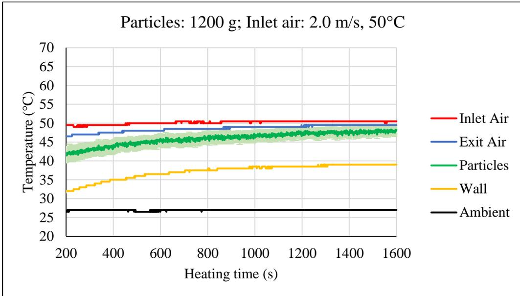
Figure 61. Online monitoring of 1200 g particles heated by 2.0 m/s and 50°C inlet air.
