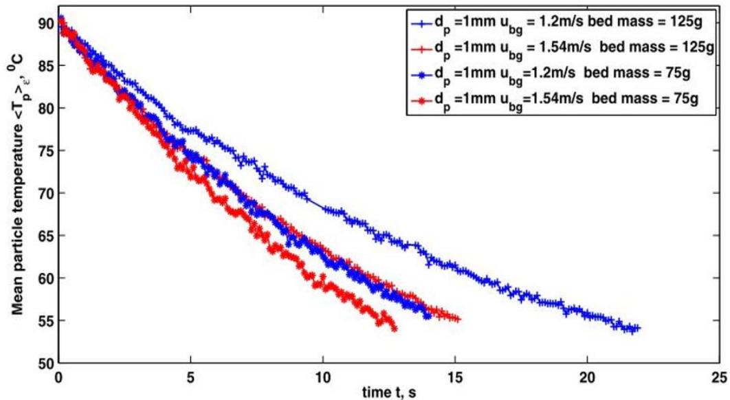
Figure 18. Mean temperatures of particles with time in a cooling process (A. V. Patil, Peters, Sutkar, et al., 2015).
