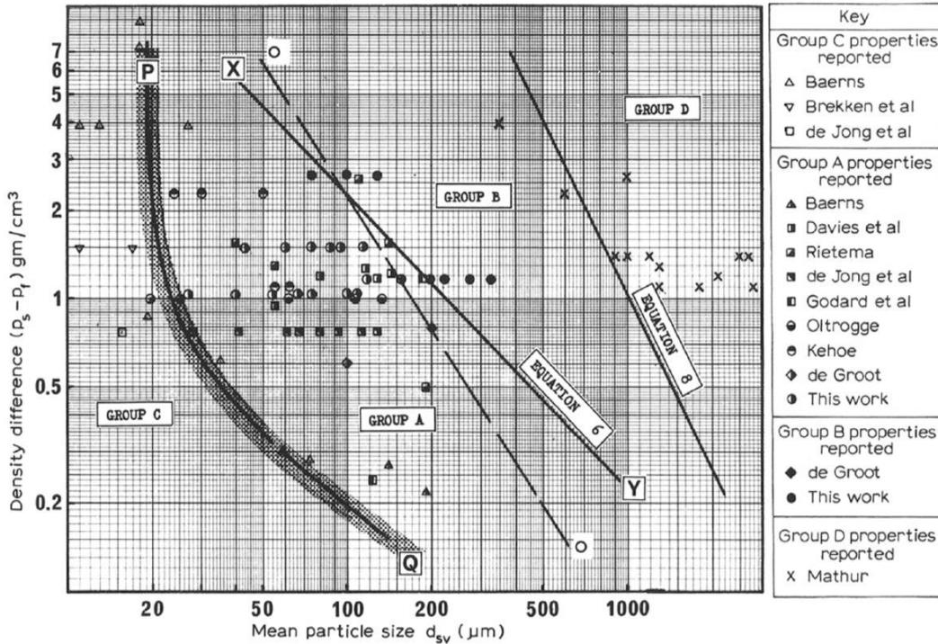
Figure 3. Diagram of the Geldart classification (Geldart, 1973).
