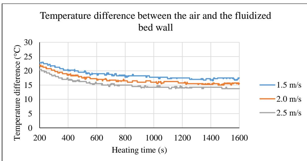
Figure 59. Effect of the inlet air velocity on the temperature difference between the air and the fluidized bed wall.
