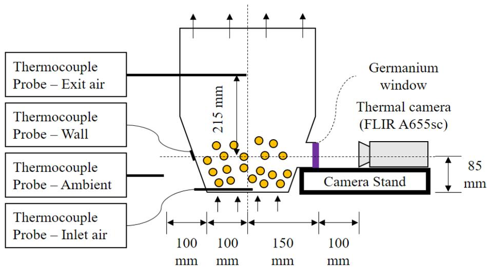
Figure 24. Experimental setup.
