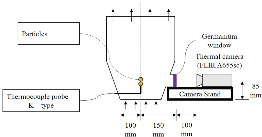
Figure 46. Calibration method B (experimental setup).
