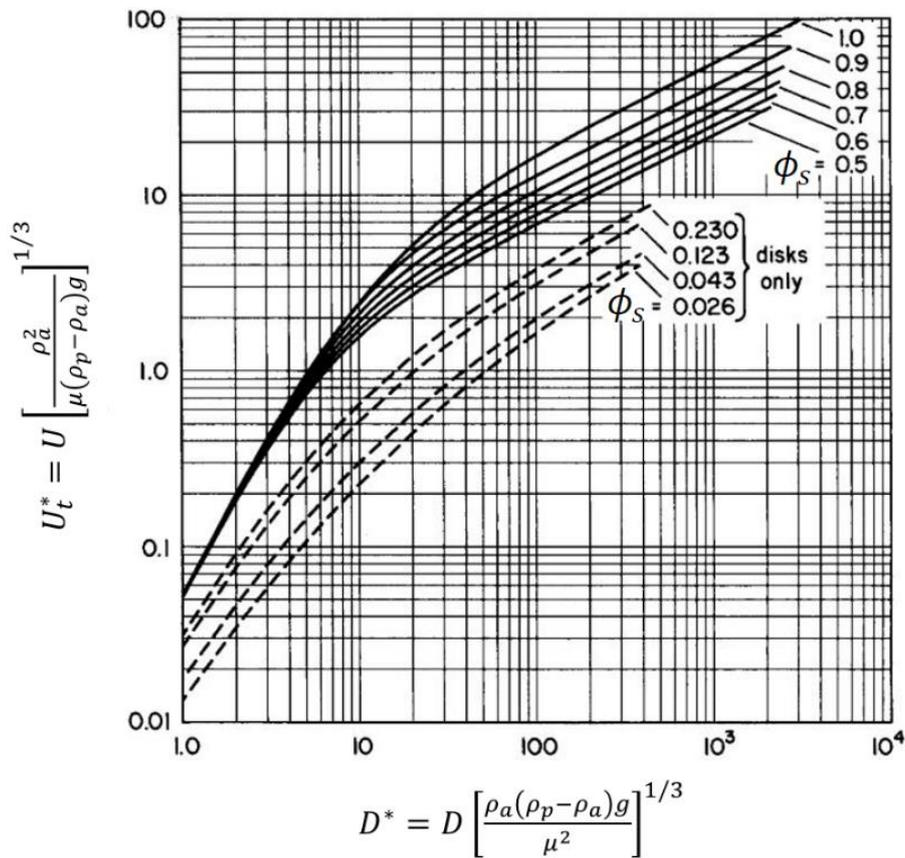
Figure 5. Chart for finding the terminal velocity of a single particle (Haider & Levenspiel, 1989).
