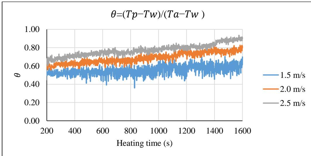
Figure 60. Effect of the inlet air velocity on  $\theta$ .
