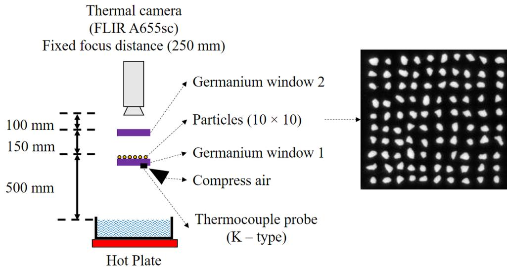
Figure 38. Calibration of the particle size and shape (experimental setup).
