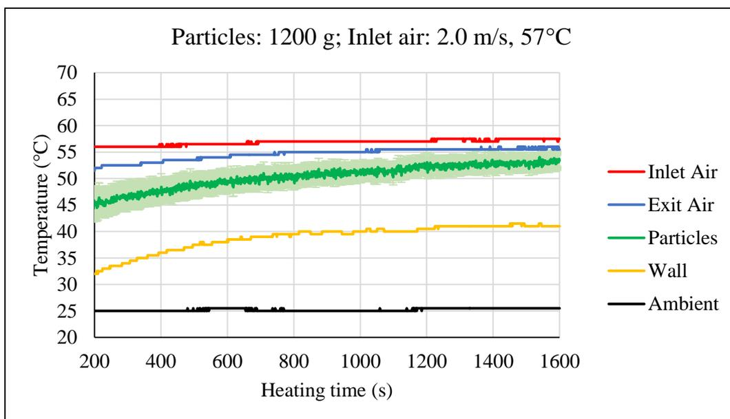
Figure 56. Online monitoring of 1200 g particles heated by 2.0 m/s and 57°C inlet air.
