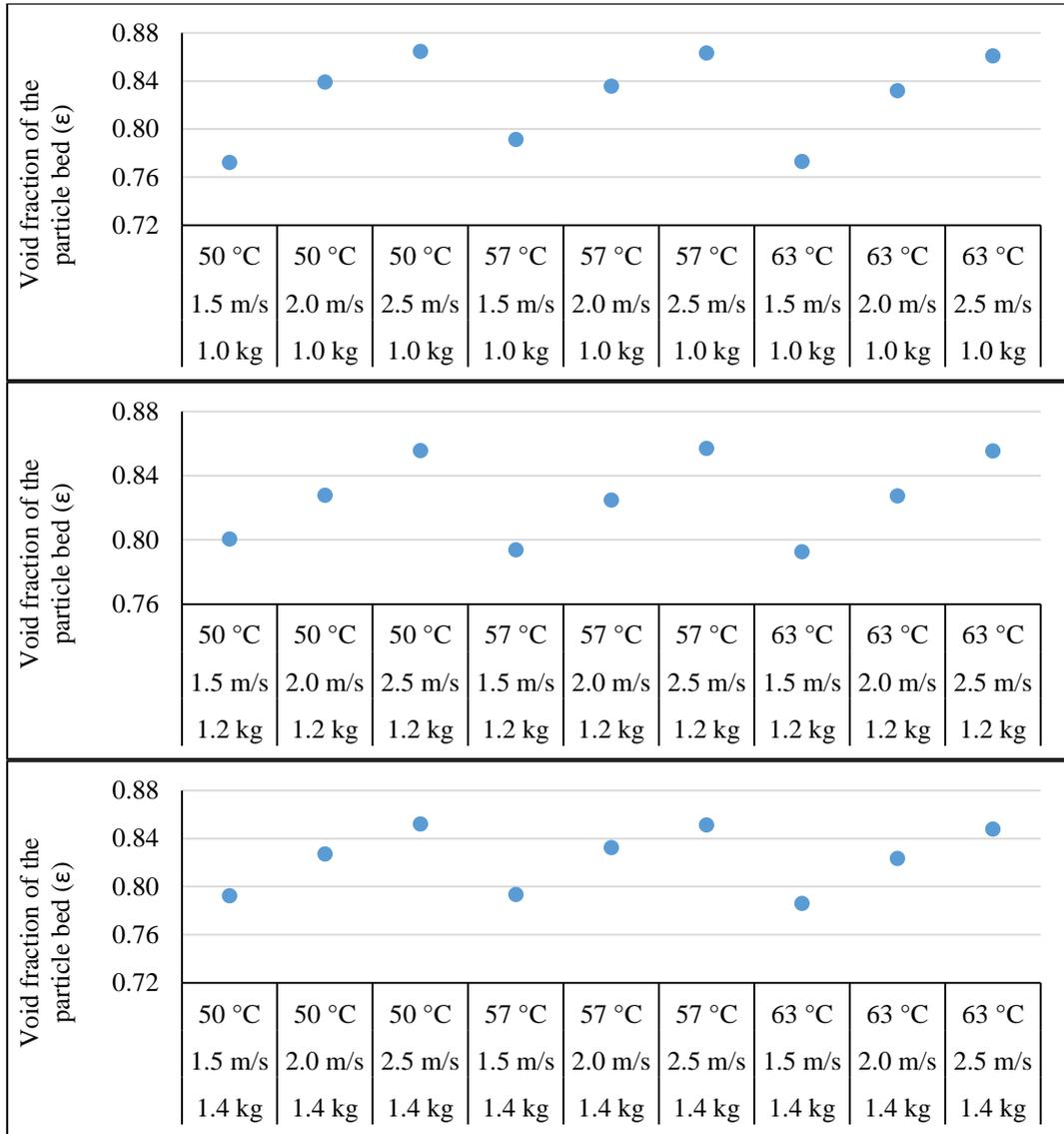
Figure 77. Void fraction of the particle bed.
