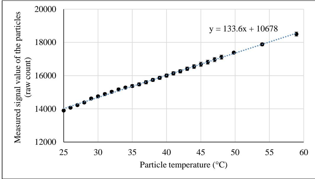
Figure 53. Correlate the measured signal value of the particles to the particle temperature.
