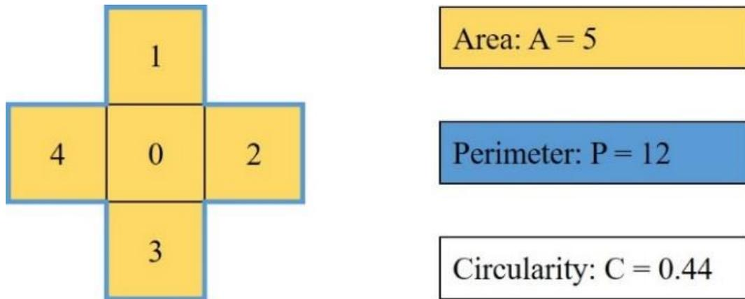
Figure 22. Example for calculating the particle size and shape.
