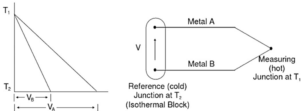
Figure 8. Structure of a thermocouple (J. Park & Mackay, 2003).
