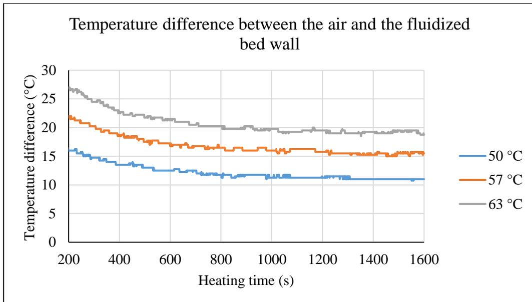
Figure 64. Effect of the inlet air temperature on the temperature difference between the air and the fluidized bed wall.
