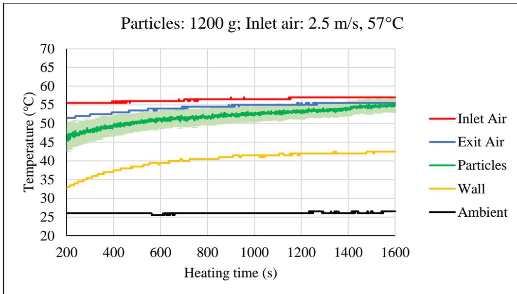
Figure 57. Online monitoring of 1200 g particles heated by 2.5 m/s and 57°C inlet air.
