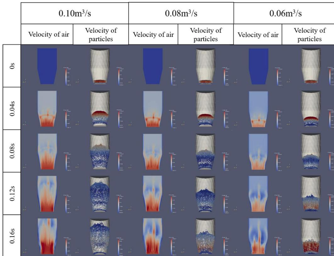
Figure 101. CFD-DEM Simulation of fluidized bed (future work).
