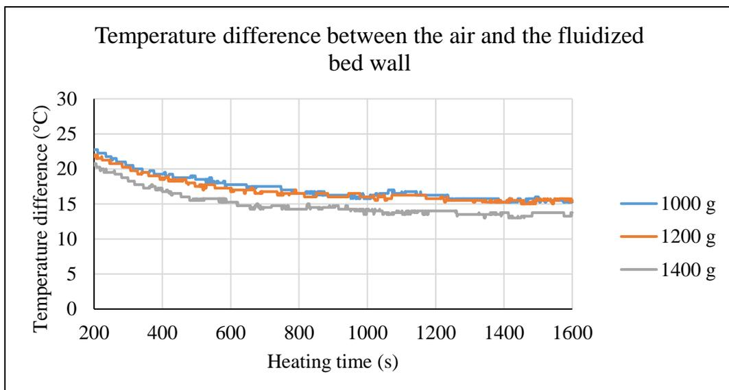
Figure 69. Effect of the loaded particle mass on the temperature difference between the air and the fluidized bed wall.
