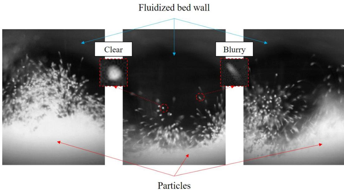
Figure 25. Example of the thermal images.
