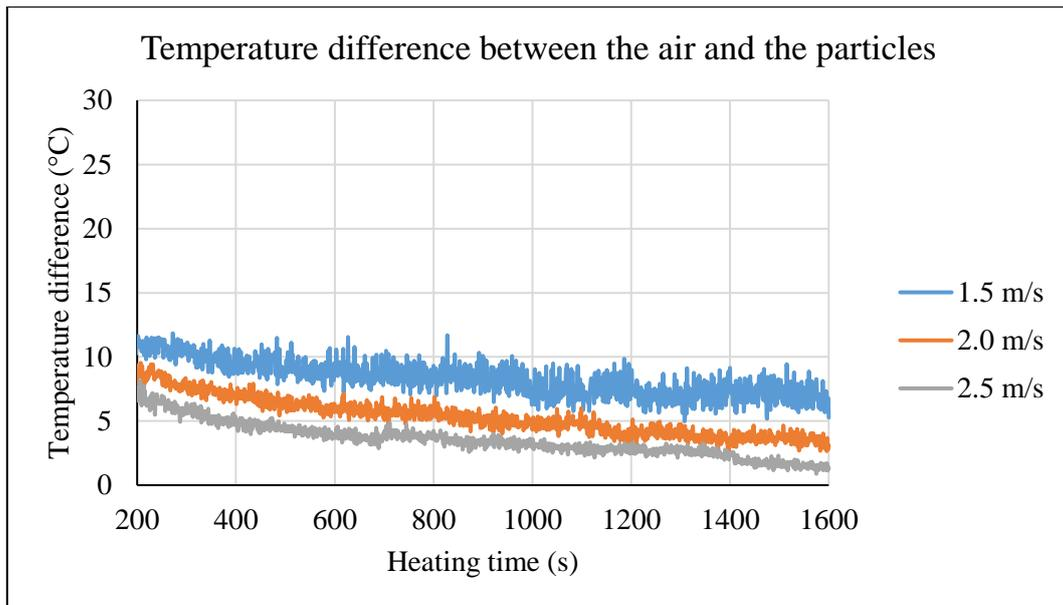
Figure 58. Effect of the inlet air velocity on the temperature difference between the air and the particles.
