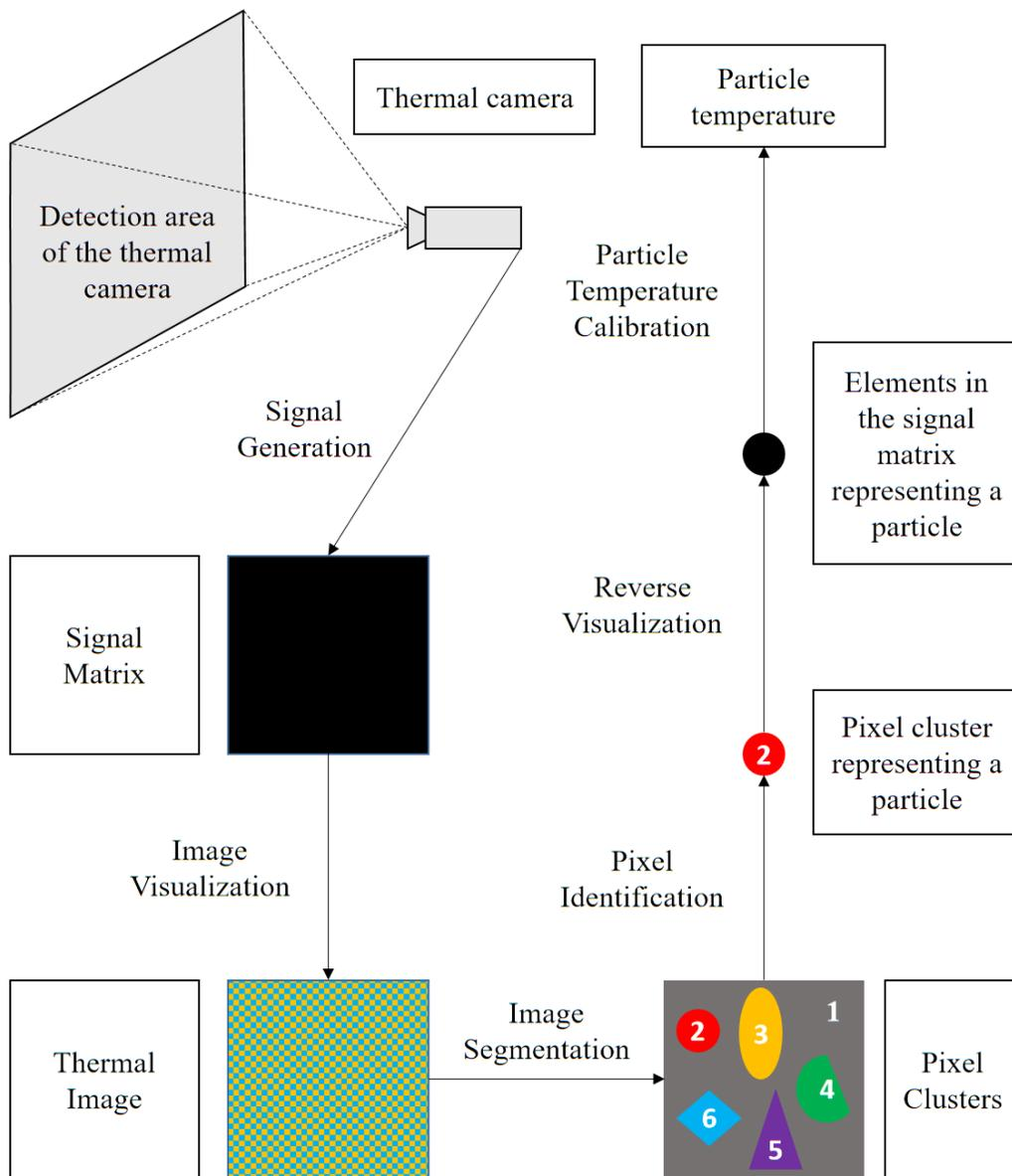
Figure 1. Temperature measurement using a thermal camera.
