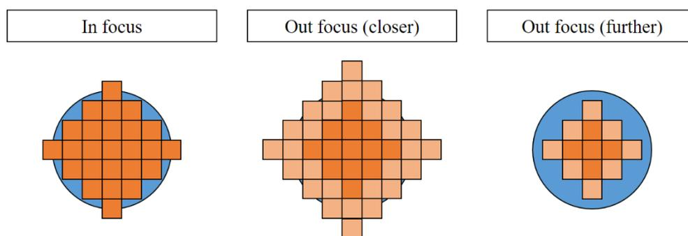
Figure 26. Blurry particles caused by the focus of the thermal camera.
