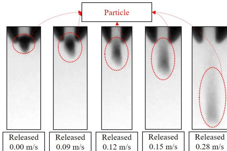
Figure 32. Blurry particle caused by the movement of the particle (thermal images).
