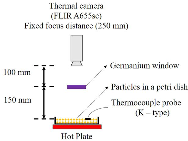
Figure 44. Calibration method A (experimental setup).
