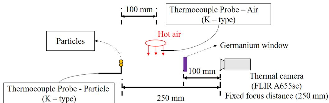
Figure 42. Effect of hot inlet air on the relationship between the signal values corresponding to the identified pixels and the particle temperature (experimental setup).
