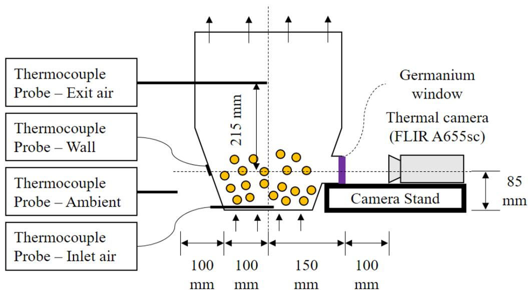
Figure 54. Experimental setup.
