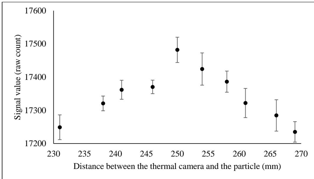
Figure 30. Blurry particle caused by the focus of the thermal camera (signal value).
