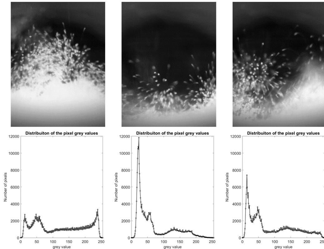
Figure 34. Distribution of the pixel grey values in the thermal images.
