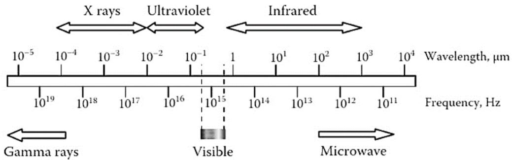
Figure 10. Names of the radiation with different wavelength (Pan & Atungulu, 2010).
