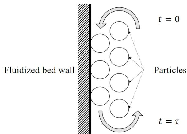
Figure 19. Models for heat transfer between particles and the fluidized bed wall.
