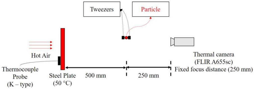
Figure 31. Blurry particle caused by the movement of the particle (experimental setup).
