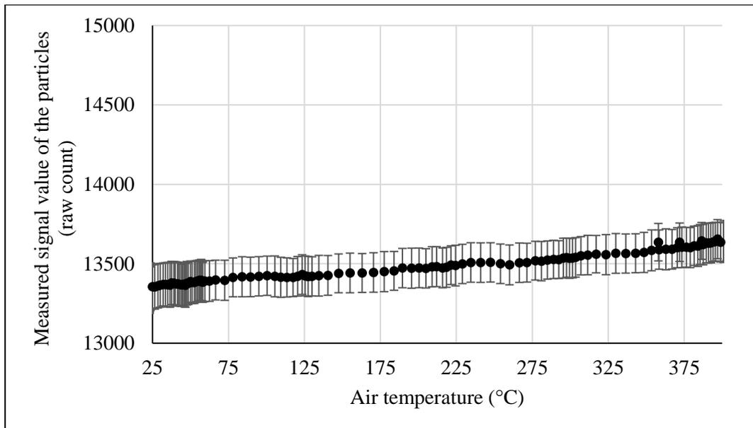
Figure 43. Effect of hot inlet air on the relationship between the signal values corresponding to the identified pixels and the particle temperature (results).
