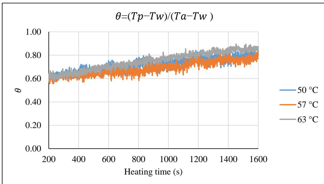
Figure 65. Effect of the inlet air temperature on  $\theta$ .
