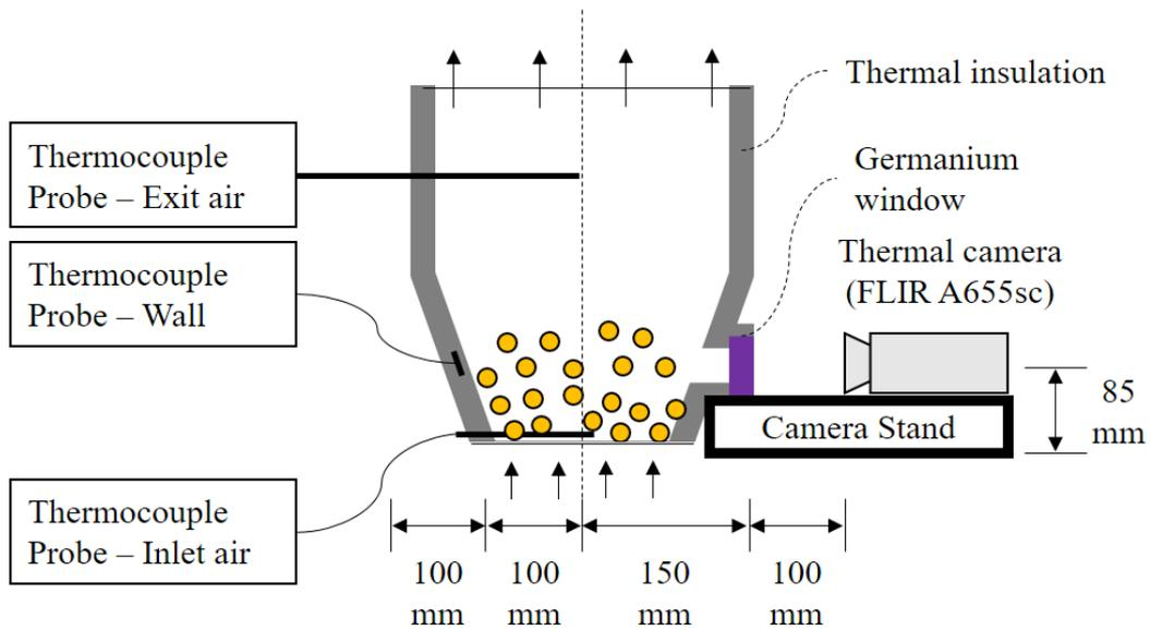
Figure 49. Calibration Method C (experiment).
