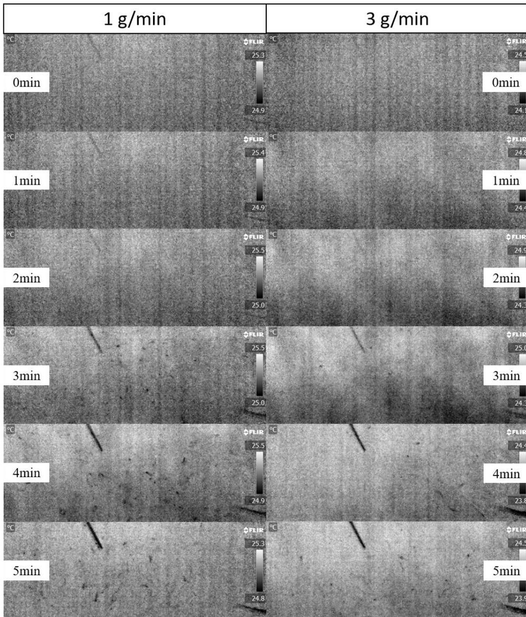
Figure 100. Comparison of the contact between particles and droplets with two different spray rates.
