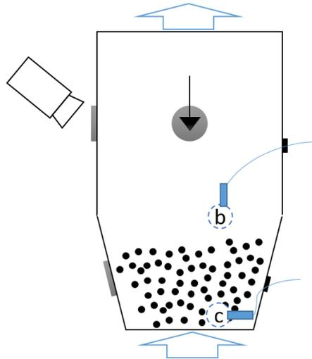
Figure 94: Monitor the temperature of air and particles without water sprayed
