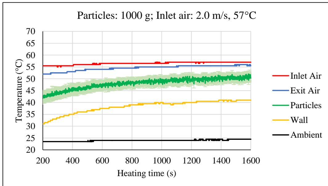
Figure 66. Online monitoring of  $1000\text{ g}$  particles heated by  $2.0\text{ m/s}$  and  $57^\circ\text{C}$  inlet air.
