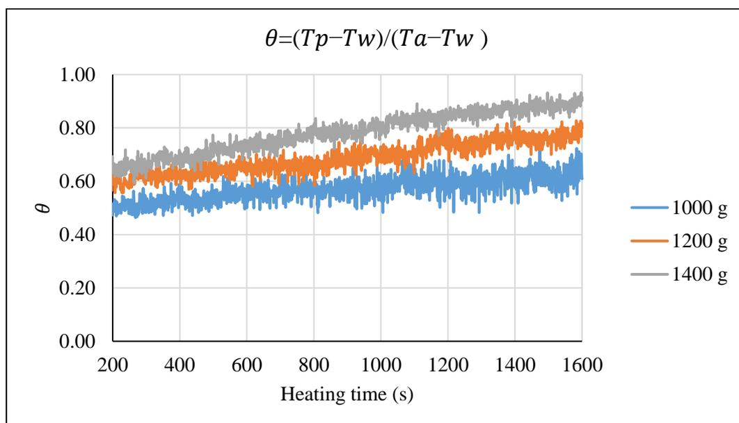
Figure 70. Effect of the loaded particle mass on  $\theta$ .
