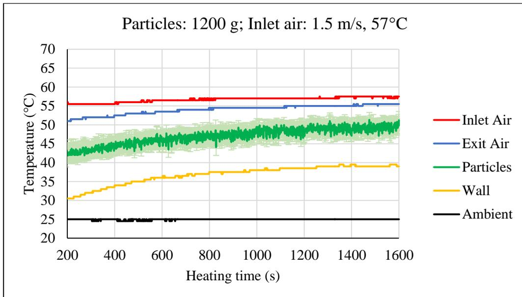
Figure 55. Online monitoring of 1200 g particles heated by 1.5 m/s and 57°C inlet air.
