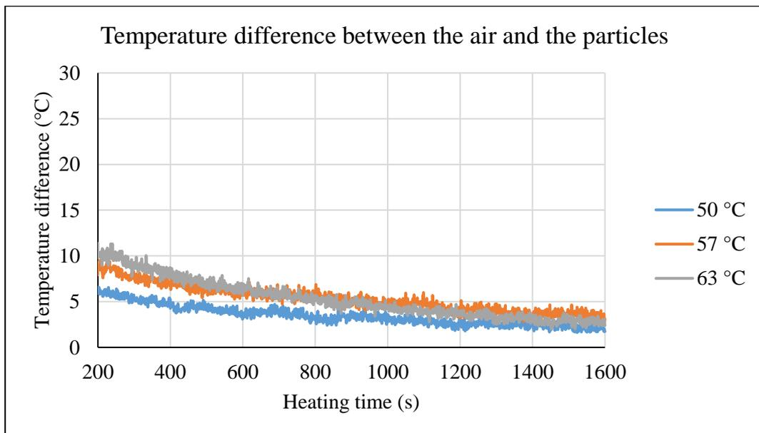
Figure 63. Effect of the inlet air temperature on the temperature difference between the air and the particles.
