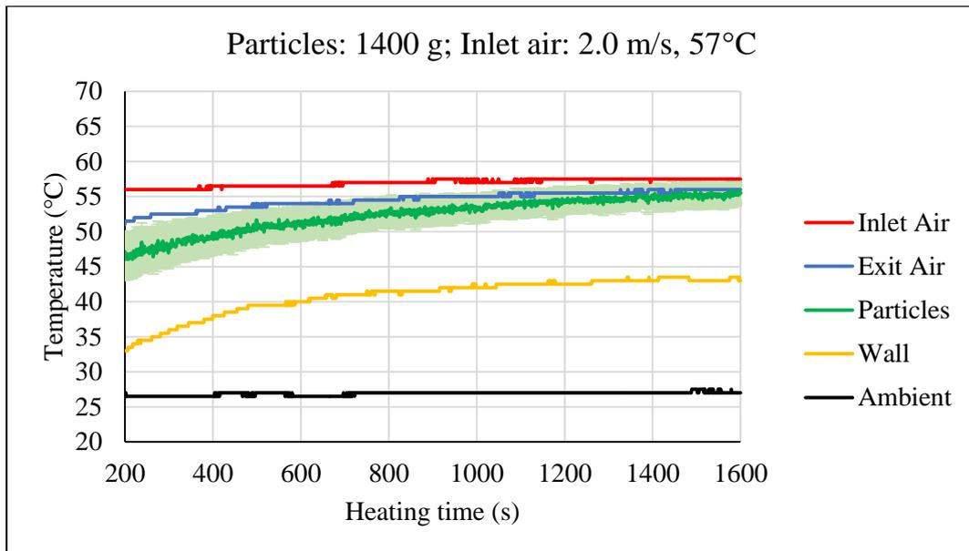
Figure 67. Online monitoring of 1400 g particles heated by 2.0 m/s and 57°C inlet air.
