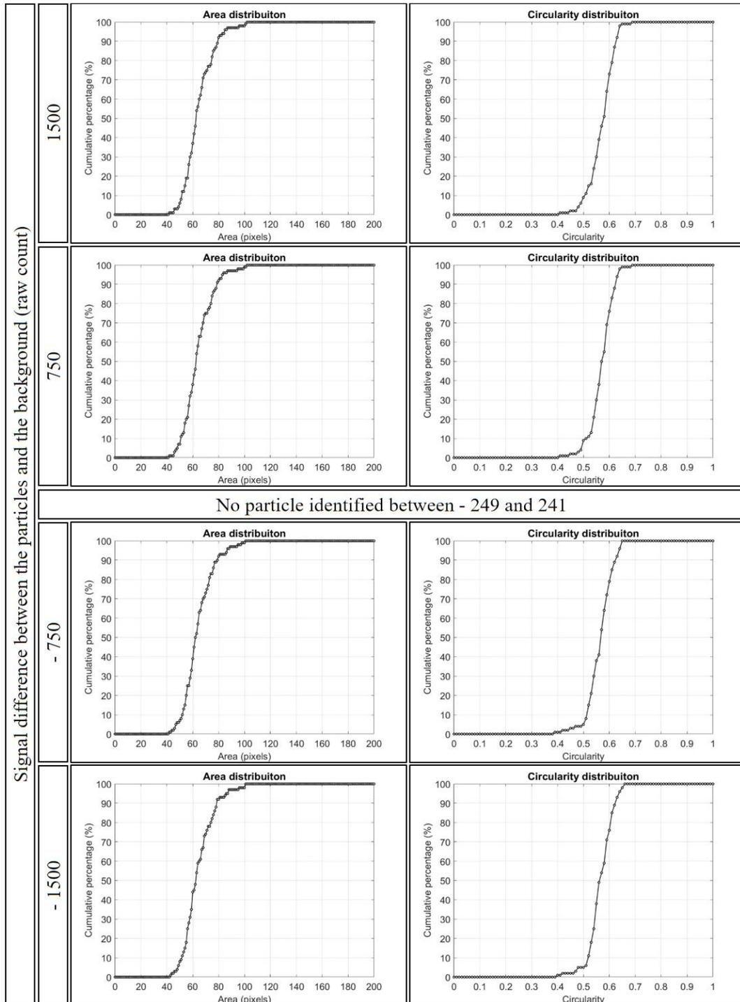
Figure 40. Calibration of the particle size and shape (cumulative distribution).
