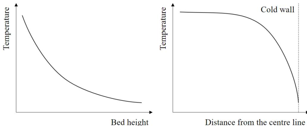
Figure 16. Typical temperature profile for a spouted bed (Malek & Lu, 1964).
