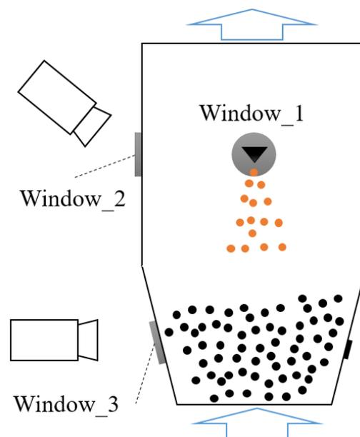
Figure 90: Thermal camera set-up
