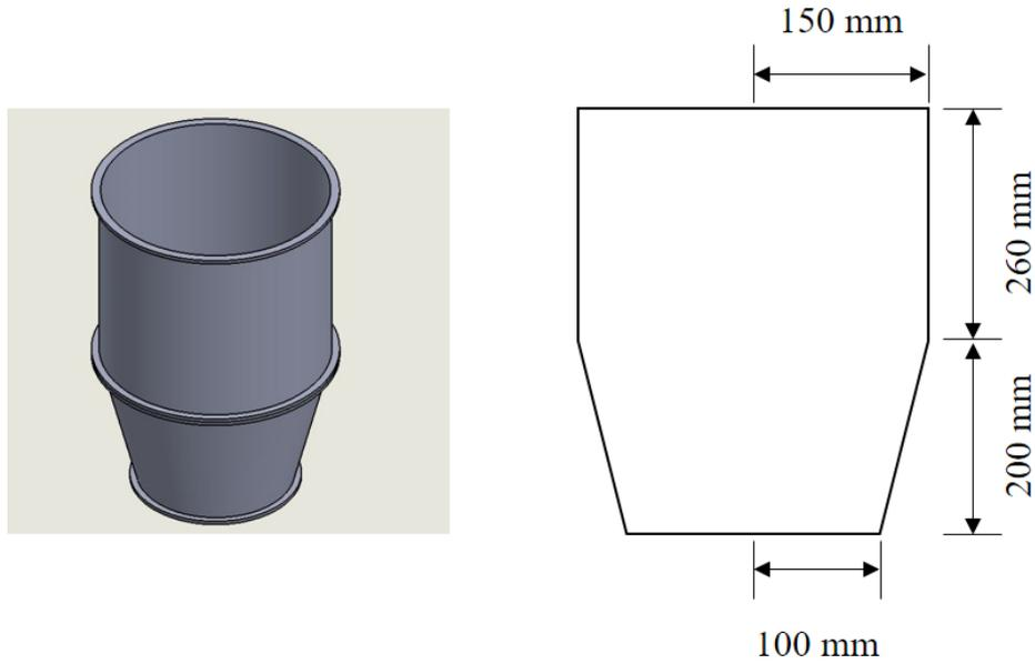
Figure 23. Dimension of the fluidized bed (GLATT-WSG-3).
