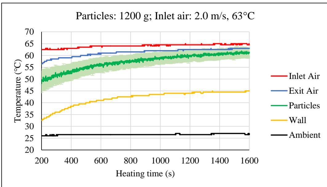
Figure 62. Online monitoring of 1200 g particles heated by 2.0 m/s and 63°C inlet air.
