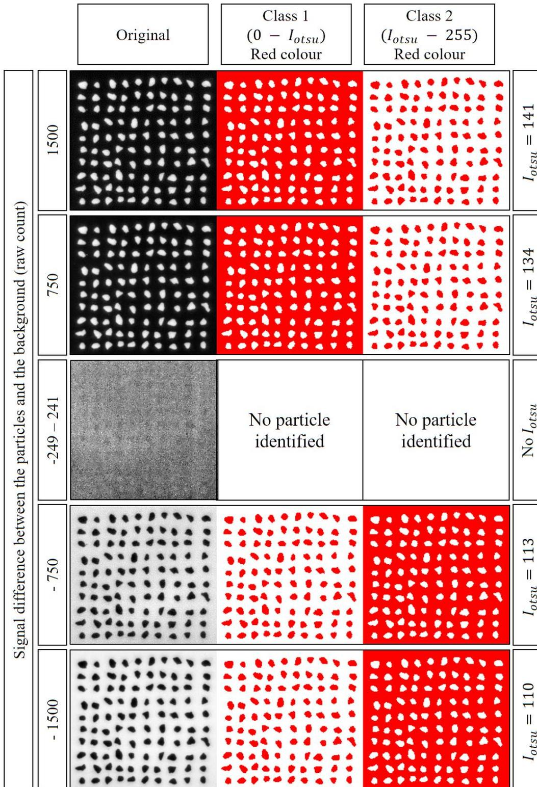
Figure 39. Calibration of the particle size and shape (pixel classes from the thermal images).
