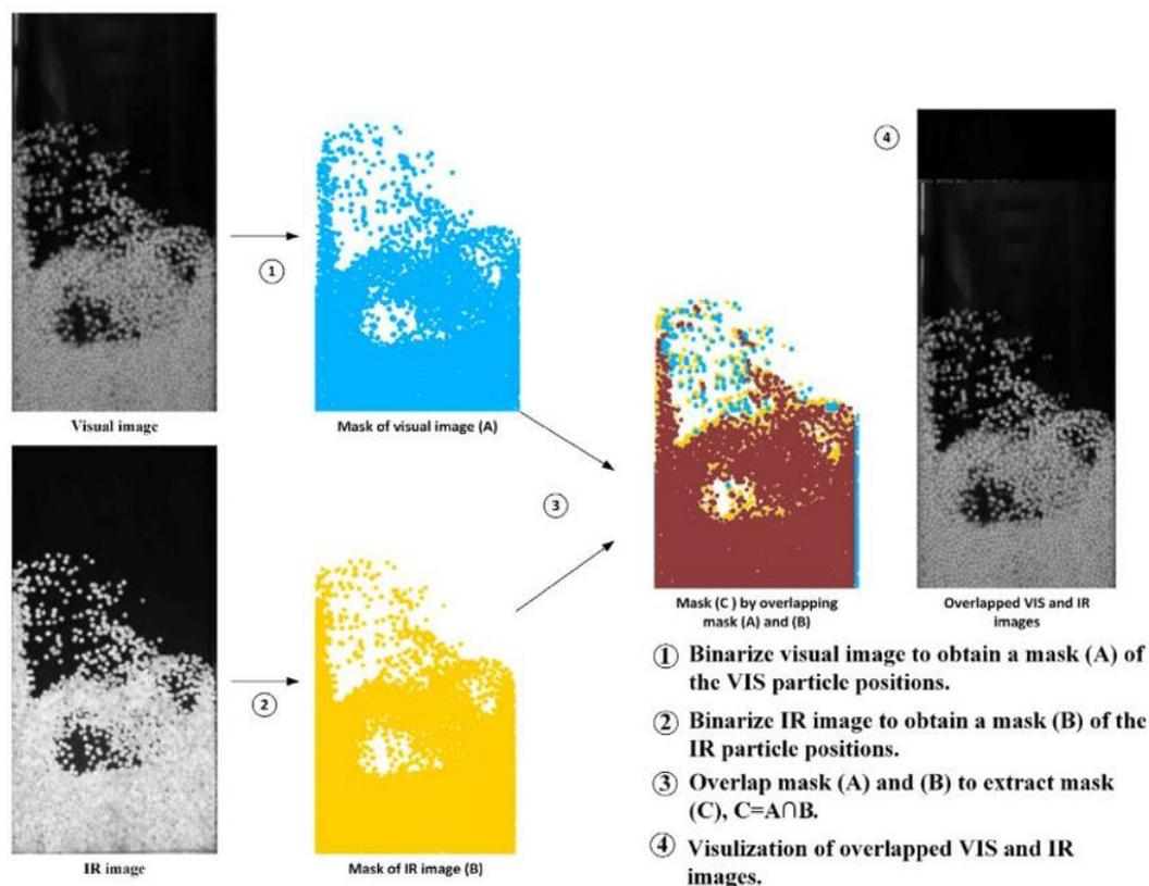
Figure 15. Thermal images used by Li et al. (2017).
