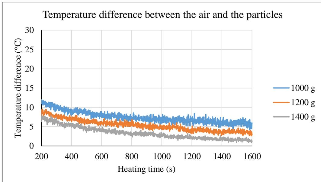
Figure 68. Effect of the loaded particle mass on the temperature difference between the air and the particles.
