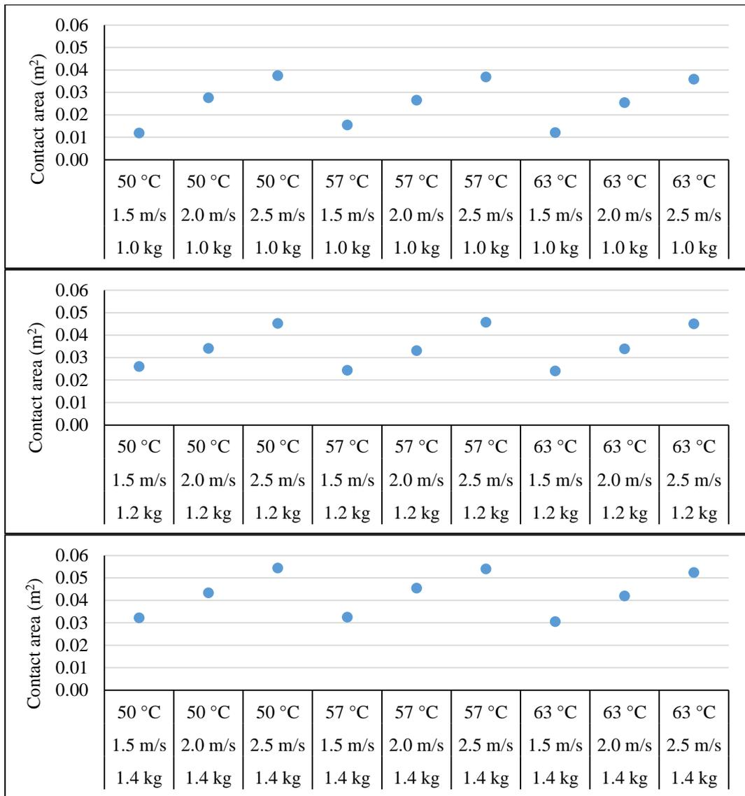
Figure 75. Contact area between the particles and the Fluidized bed wall ( $m^2$ ).
