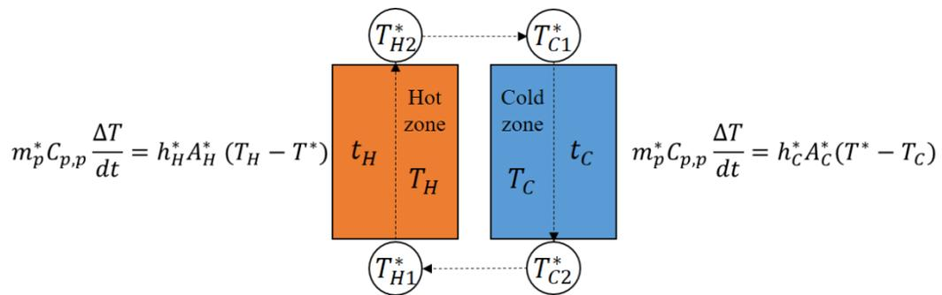
Figure 80. Two compartment model (single particle).
