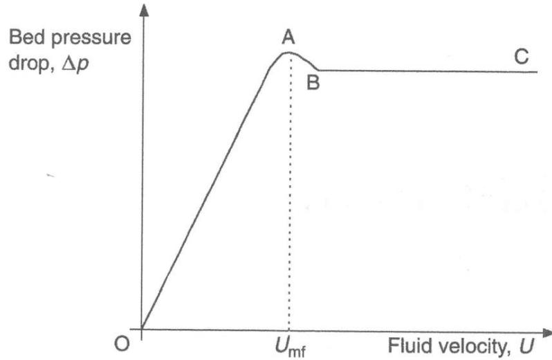
Figure 4. Ideal pressure drop velocity curve (Rhodes, 2008).
