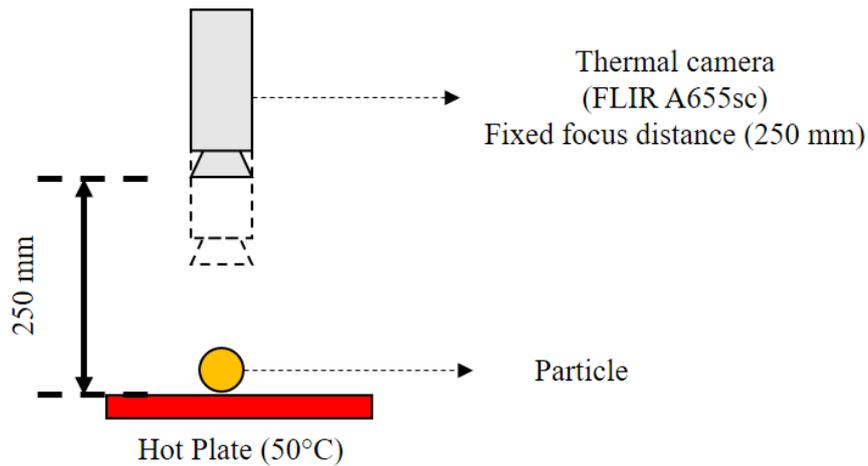
Figure 28. Blurry particle caused by the focus of the thermal camera (experimental setup).
