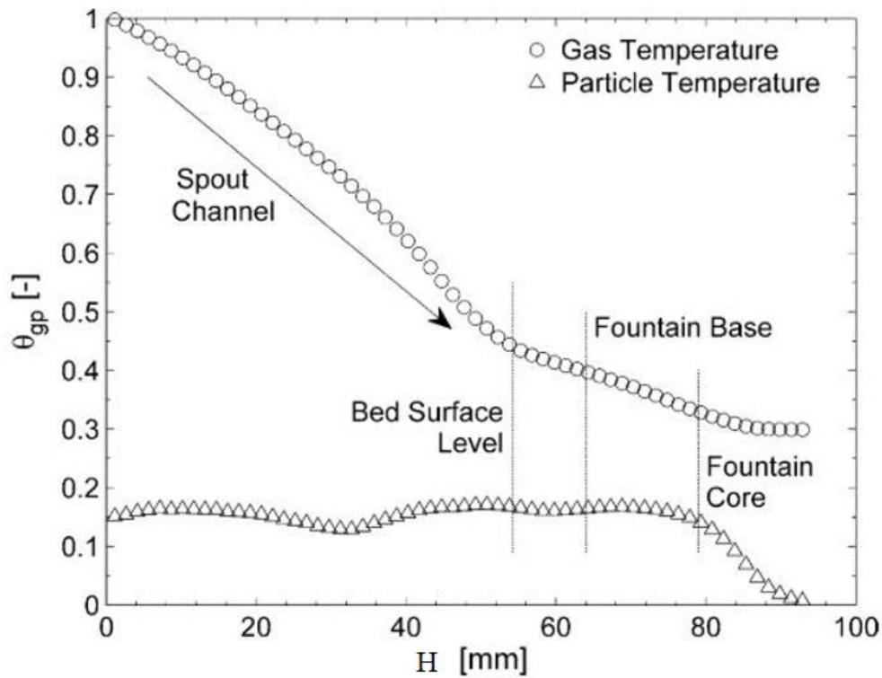
Figure 17. The 60 s time average dimensionless air and particle temperature distribution in the spouted regime at  $3.0 u_{mf}$  (Brown & Lattimer, 2013).
