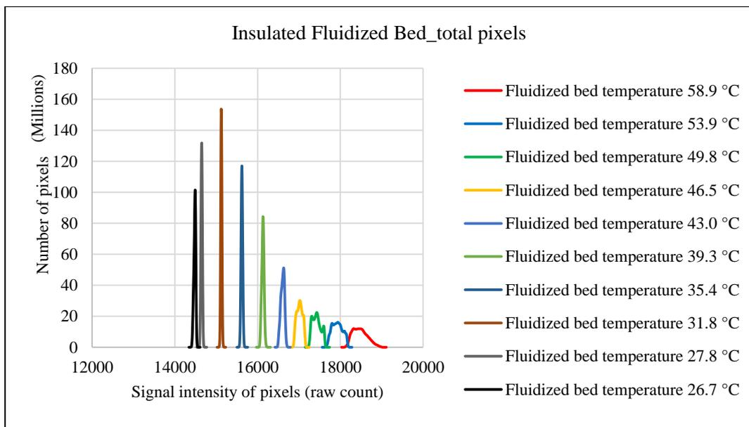
Figure 50. Total pixels in the thermal images (2 min).
