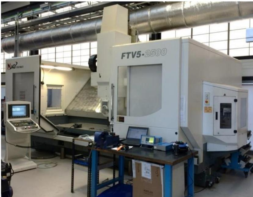
**Figure 3.9 – MAG Cincinnati FTV5 milling machine**
