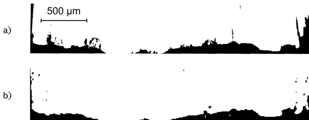
**Figure 4.32 – Binary image representation of damage for a) EFM and b) XCT images showing more captured damage through a), the EFM method which captures 3.77% more damage due to increased resolution**
