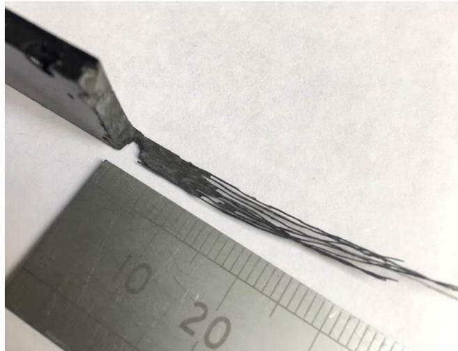
**Figure 7.4 – a) Up milling configuration for flexural coupons shown in black with red showing small overhang and b) result of small overhang edge trimming showing fibres exposed by pyrolysis of the epoxy matrix during CFRP milling at starting temperature of 50 °C**
