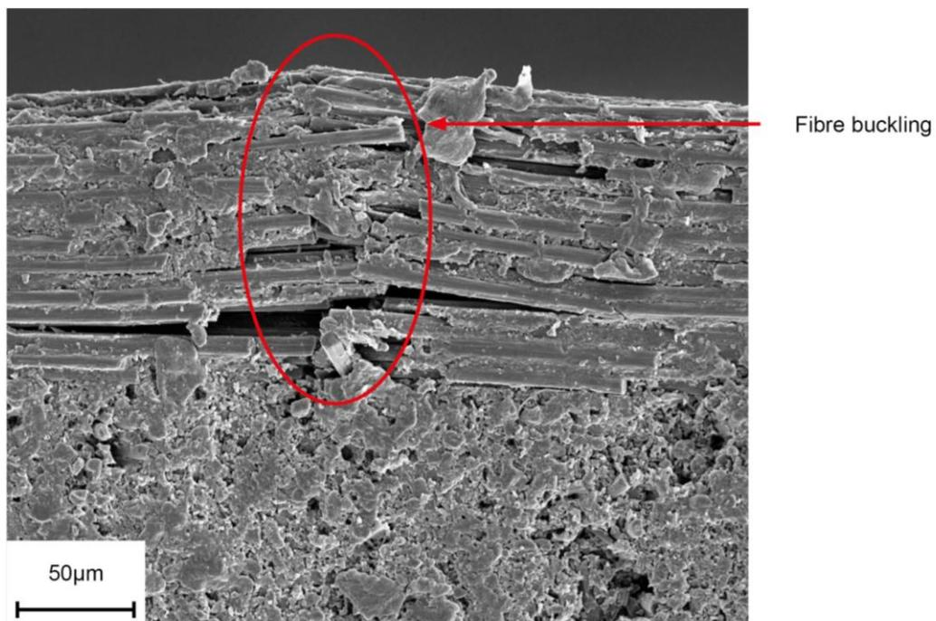
**Figure 7.16 – Typical buckling of  $0^\circ$  fibres at the top surface which started at CFRP preheating temperatures of  $40^\circ\text{C}$  (image of buckling at  $100^\circ\text{C}$ )**
