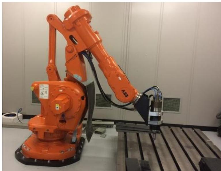
Figure 3.10 – ABB IRB6660 Engineering robotic arm with spindle
