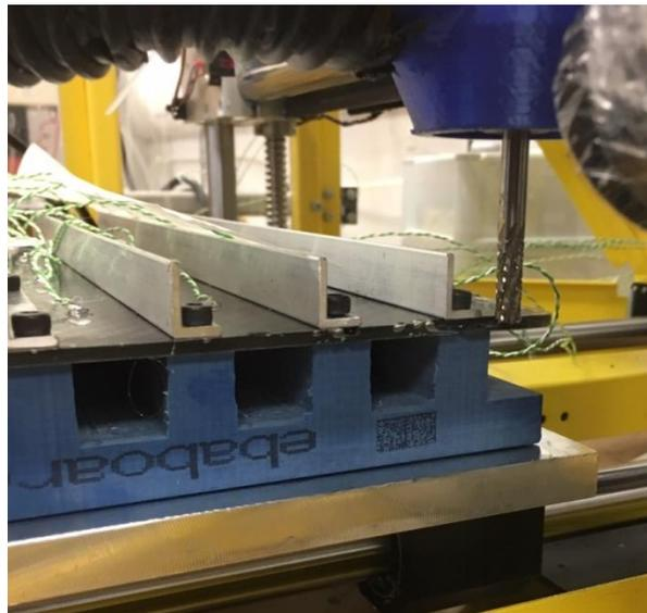
**Figure 4.13 – Final GTC milling fixture for preliminary tool wear and temperature trials showing Aluminium L-brackets and Ebaboard slots for tool clearance**
