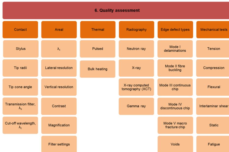
**Figure 2.17 – Quality assessment of edge trimmed CFRP [10, 82]**
