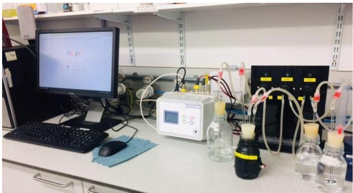
**Fig. 6-7** Complete bioreactor unit
