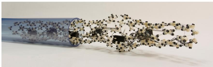
Figure 2.24: CMMWorm, continuous-wave peristalsis pipe robot [19].
