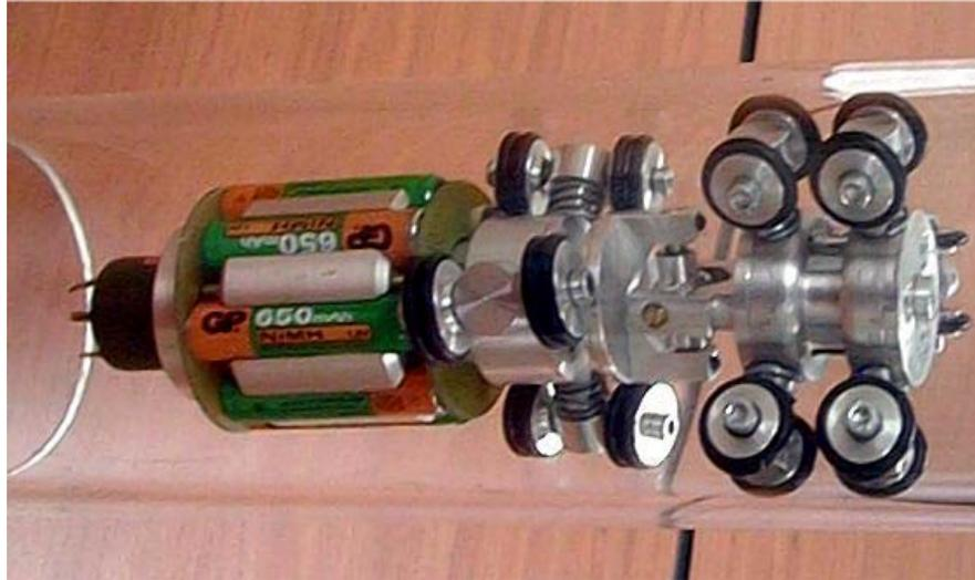
Figure 2.18: Heli-Pipe screw wall-press system [13].
