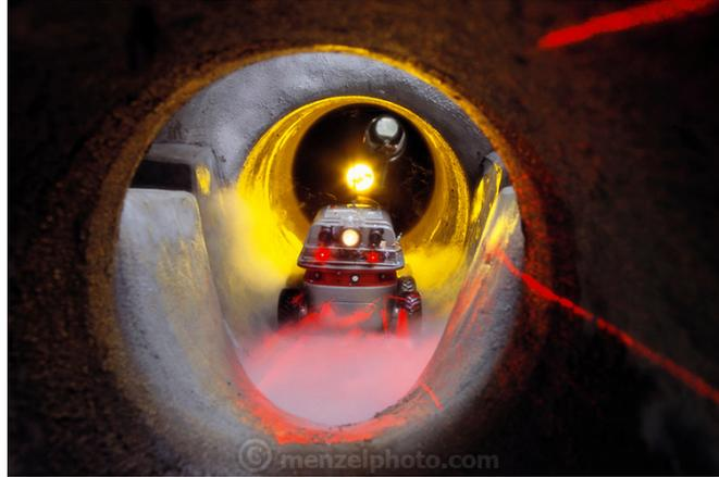
Figure 2.8: Kurt II, an autonomous wheeled in-pipe robot [3].
