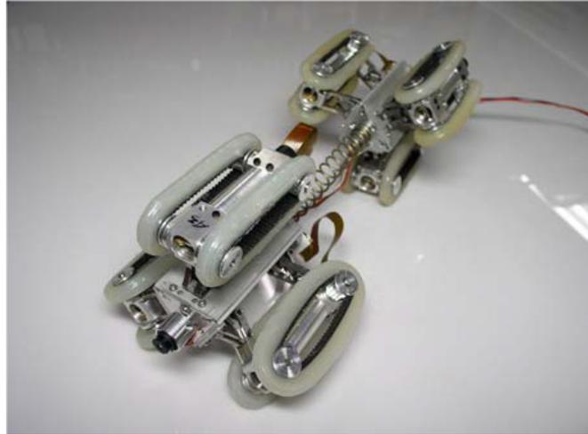
Figure 2.16: Hanyang's two module caterpillar wall-pressing robot [11].
