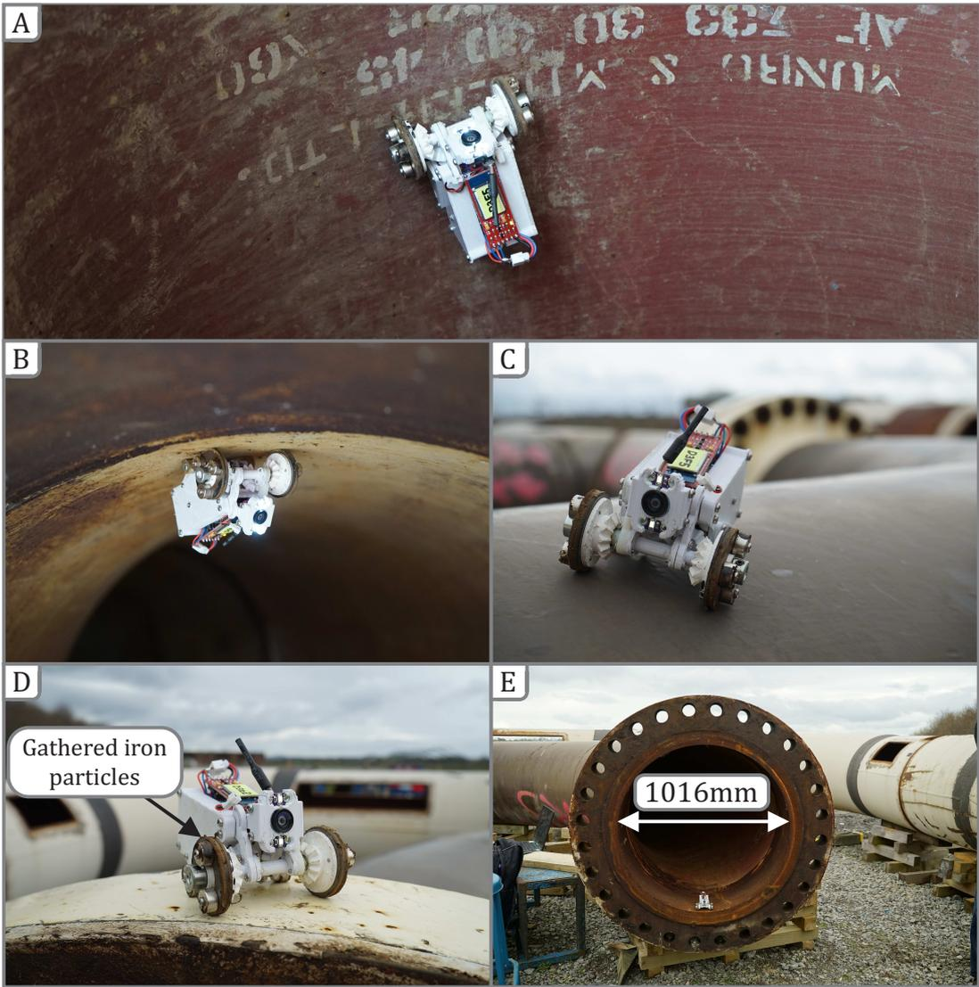
Figure 7.17: Pictures from the real world tests on a decommissioned 1016mm natural gas pipeline. A: Driving vertically. B: Inverted. C: On the outer side of the pipe. D: Iron particles and scales that "clogged" the wheel flux. E: Full shot view of the pipe size versus the robot size.
