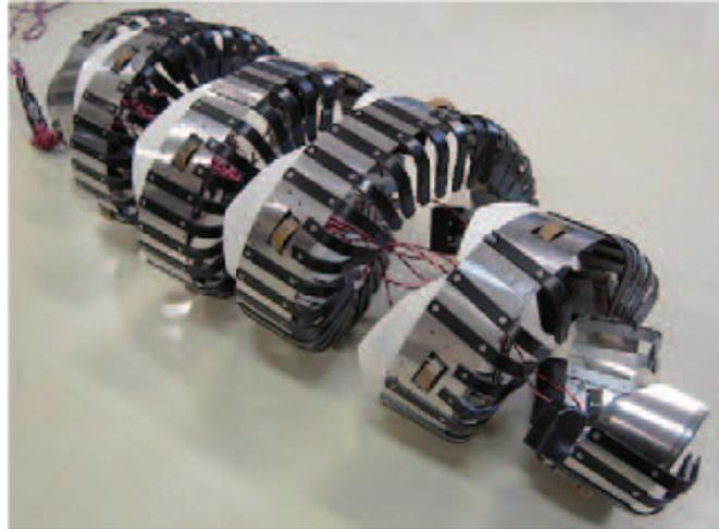
Figure 2.19: Osaka University's SPRING pipe robot [14].
