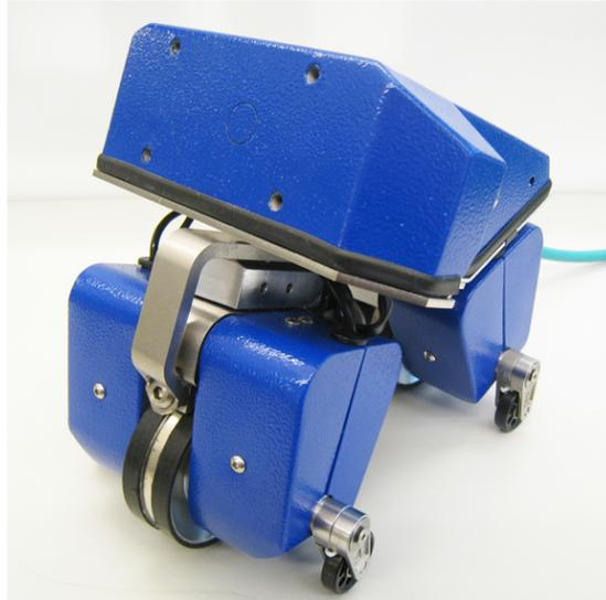
Figure 2.13: MagneBike developed by Autonomous Systems Lab, ALSTOM uses wheeled magnetic wheels with actuated lateral lever arms to overcome magnetic contact forces [8].
