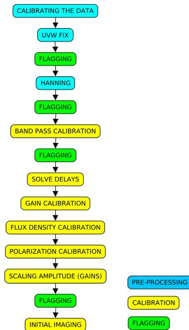
Figure 2.18: Stages of the eMerlin pipeline.
