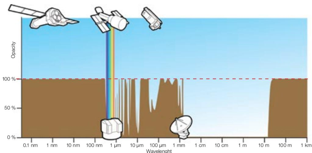
Figure 2.2: Atmospheric window (opacity generated by the atmosphere (percentage) v/s signal wavelength (m)).
