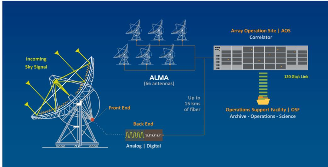
Figure 2.3: Signal processing using several radio telescopes).
