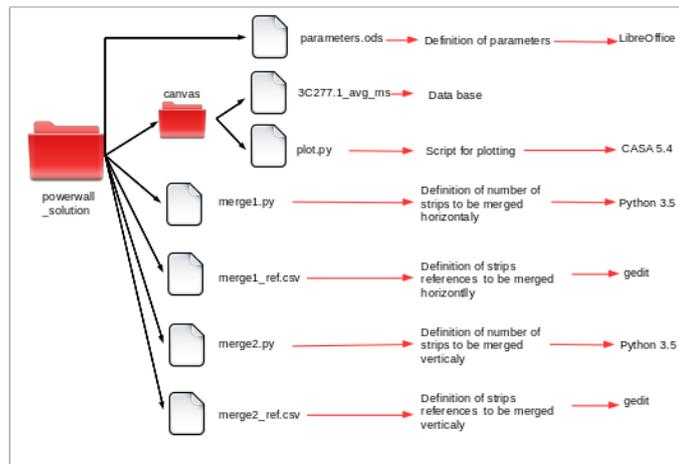
**Image 1 Software architecture of the powerwall solution**
