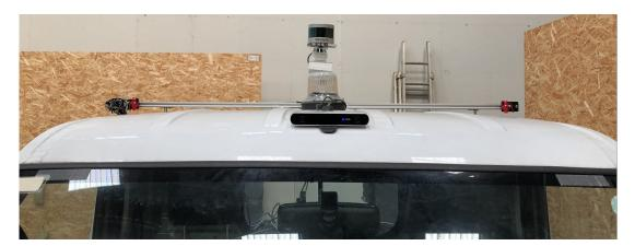
Figure 5.3: Front view to the AV showing the stereo camera, and the LiDAR which is attached to belt driven linear actuator.
