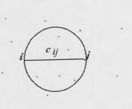
In this case, destinations are considered to be intervening if they fall within a circle, the diameter of which is the line joining origin i to destination j.
