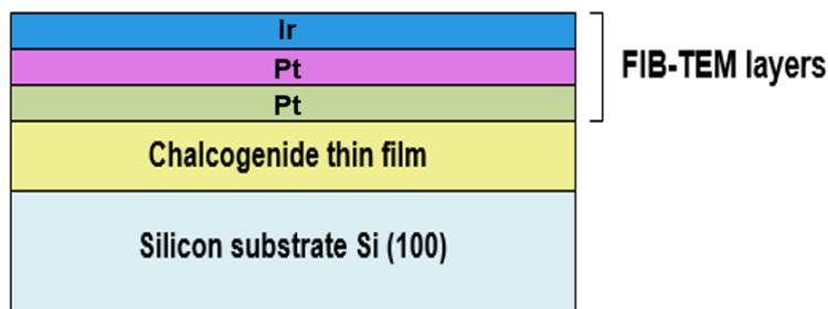
**Fig. 3.11:** Schematic diagram showing coating FIB-TEM layers.
