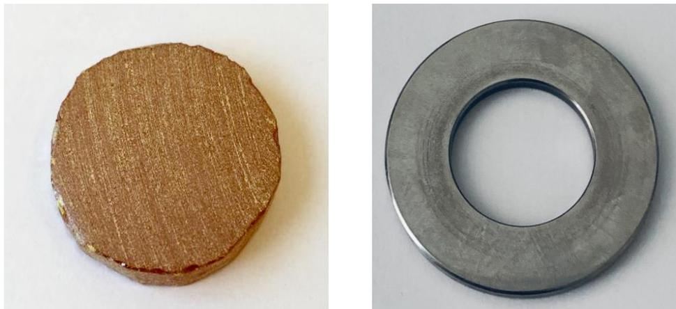
**Fig. 5.1:** Er<sup>3+</sup>-doped Ga-La-S bulk glass (**left**) and Er<sup>3+</sup>-doped Ga-La-S bulk glass holder (**right**) which is used for fs-PLD.
