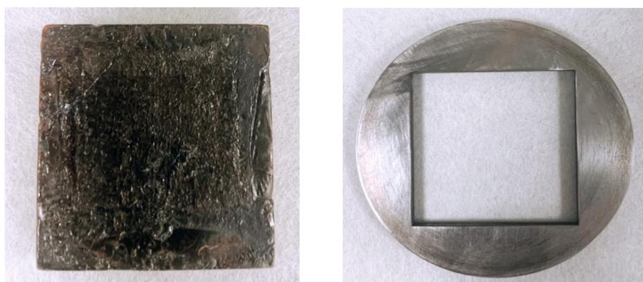
**Fig. 6.1:** GeSe<sub>4</sub> bulk glass (**left**) and GeSe<sub>4</sub> bulk glass holder (**right**) which are used for fs-PLD.
