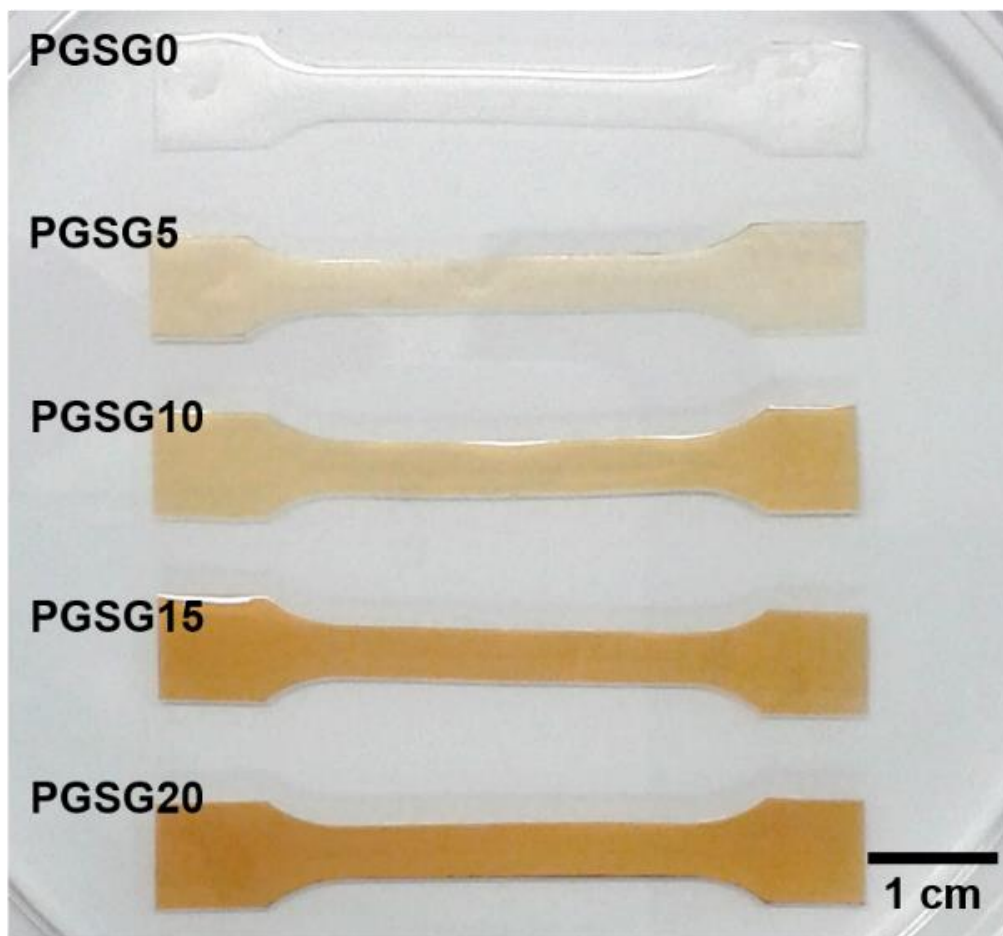
Figure 3.3 A photograph showing fully-cured PGSG copolymer specimens with various gelatin contents. The colour change from pale yellow to orange was observed due to the addition of gelatin in copolymer synthesis.
