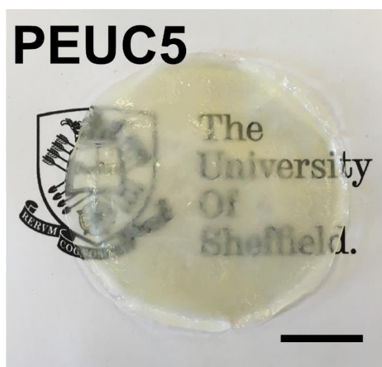
Figure 4.7 Photograph showing a PEUC5 films with visible clay agglomerates (scale bar: 2cm).
