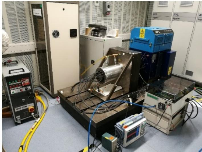
Fig. 4-18. The prototype on the test rig with oil cooling system.
