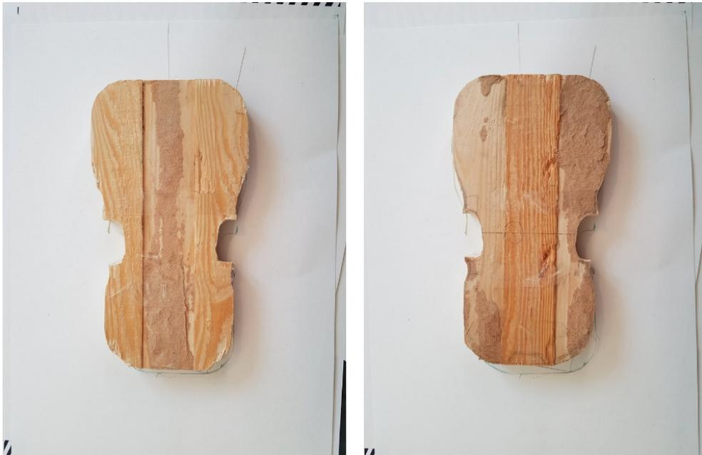
*Figure 5.3.5 Second, used wooden form in Violino-Piccolo.*
