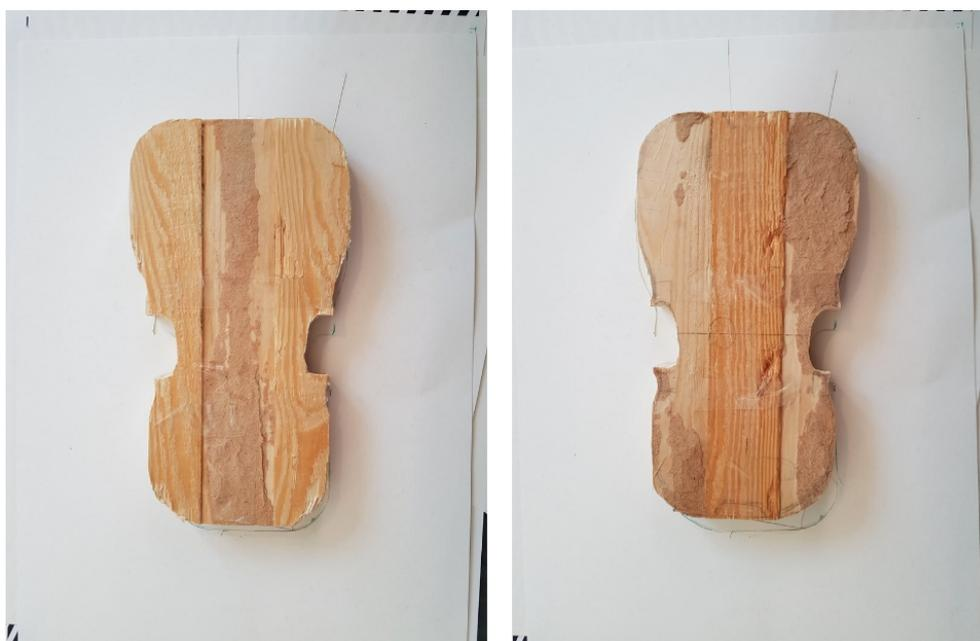
*Figure 5.3.5 Second, used wooden form in Violino-Piccolo.*
