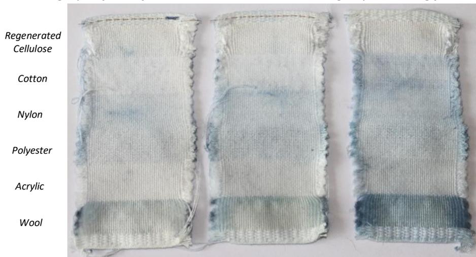
*left to right the swatches are washed without polymer, with GTAC-nanocellulose (low) and GTAC-nanocellulose (high).*
